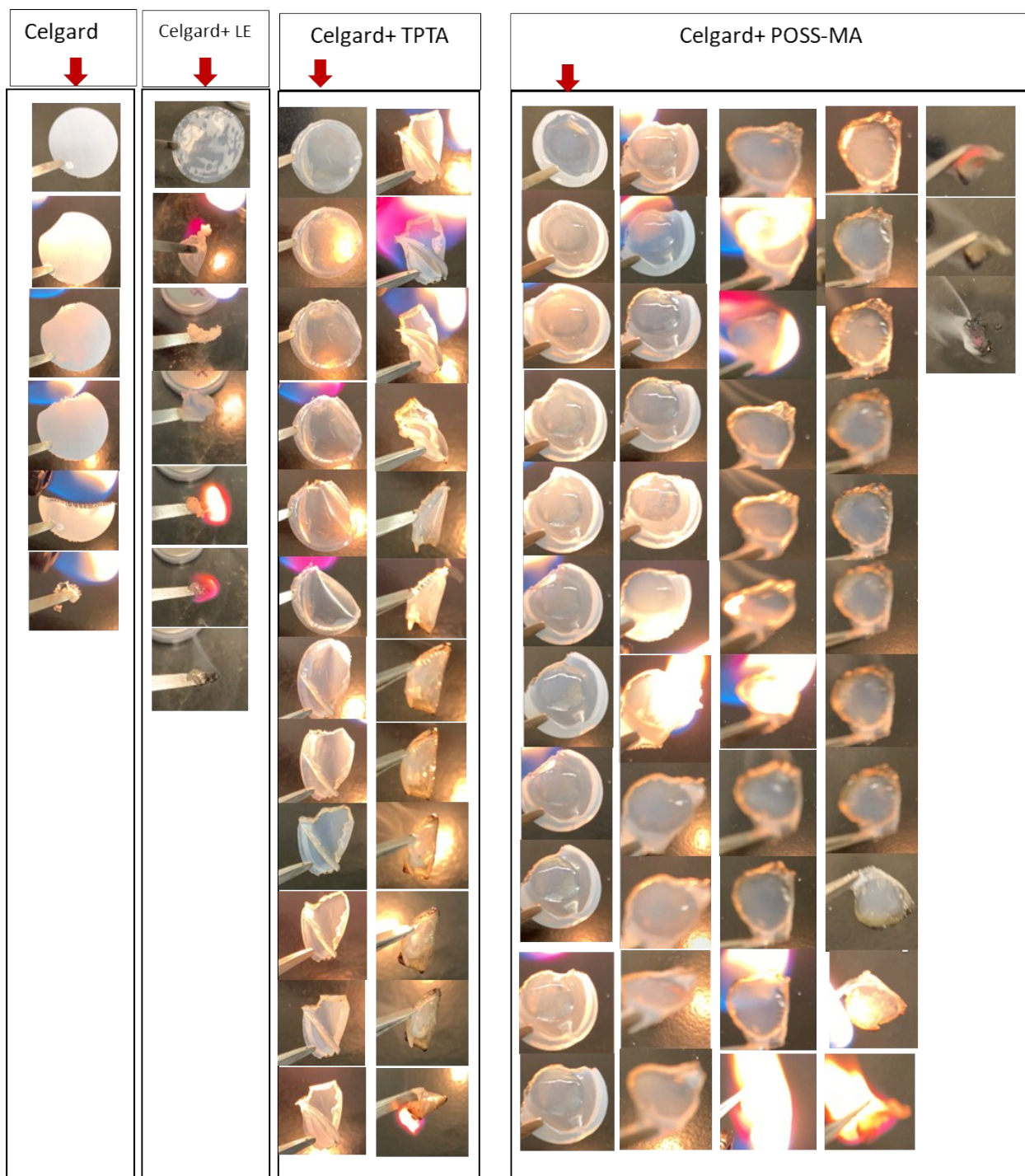
Fig. S3. Time lapse images of flammability test on a) dry celgard, b) Celgard soaked in LE, c) TPTA gelled Celgard, and d) MA-POSS gelled Celgard. Each image is after a three-second exposure of the separator to the flame.
