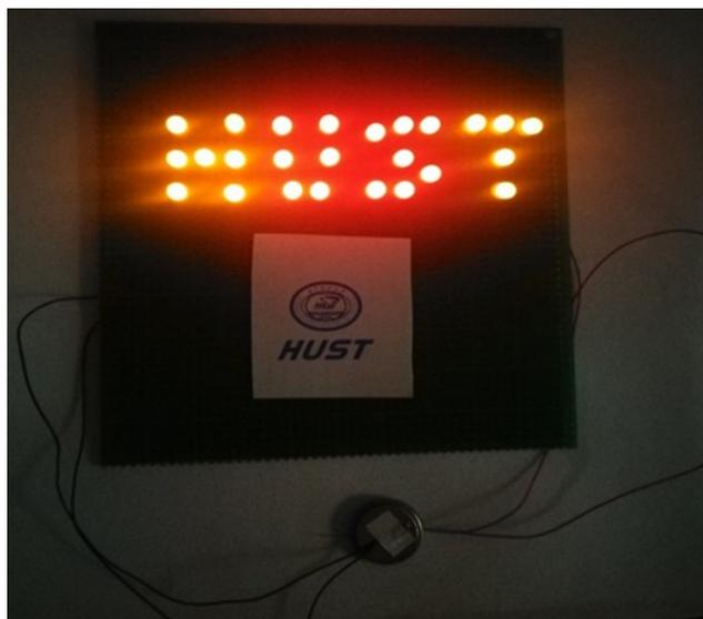
**Fig. S14.** LEDs lighted by a all-solid Li-metal battery cell.
