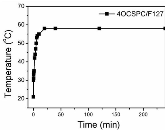
**Figure S8.** The photothermal heating curve of 4OCSPC/F127 solutions ( $C_{4OCSPC} = 5.0$   $\mu\text{g/mL}$ ) under 808 nm continuous laser irradiation at the power density of  $0.7 \text{ W/cm}^2$  for 4 h.
