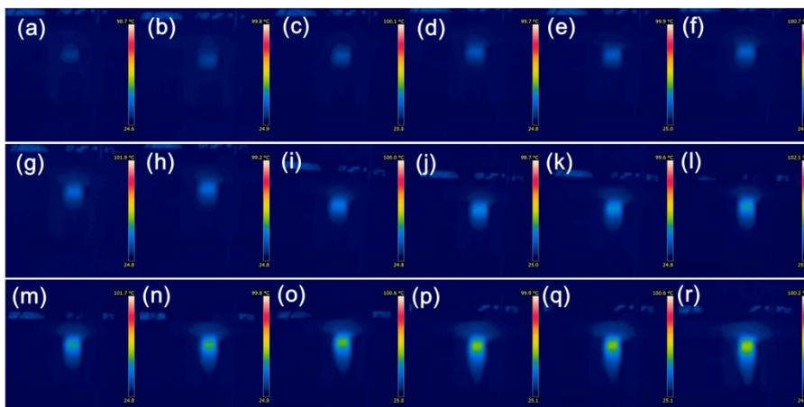
**Figure S7.** Thermal imaging of 4OCSPC/F127 micelle ( $C_{4OCSPC} = 5 \mu\text{g/mL}$ ) under 808 nm laser irradiation ( $0.7 \text{ W/cm}^2$ ) for different times, a: 0 s; b: 5 s; c: 10 s; d: 15 s; e: 20 s; f: 25 s; g: 30 s; h: 40 s; i: 60 s; j: 120 s; k: 180 s; l: 240 s; m: 300 s; n: 360 s; o: 420 s; p: 480 s; q: 540 s; r: 600 s.
