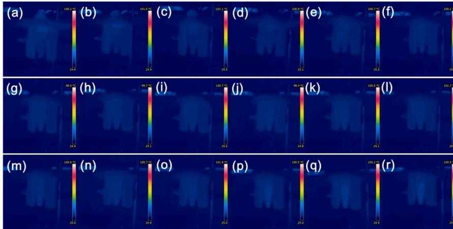
**Figure S6.** Thermal imaging of PBS under 808 nm laser irradiation ( $0.7 \text{ W/cm}^2$ ) for different times, a: 0 s; b: 5 s; c: 10 s; d: 15 s; e: 20 s; f: 25 s; g: 30 s; h: 40 s; i: 60 s; j: 120 s; k: 180 s; l: 240 s; m: 300 s; n: 360 s; o: 420 s; p: 480 s; q: 540 s; r: 600 s.
