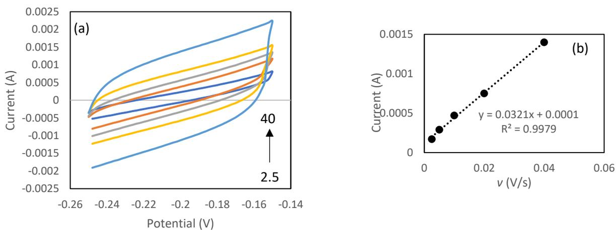
**Fig. S1** Electrochemically active surface area analysis of (a) CoNi<sub>2</sub>Se<sub>4</sub>-rGO@NF at different scan rates, (b) linear fitting of capacitive currents vs. scan rate.
