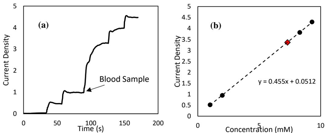
**Fig. S8** A typical electrochemical measurement for blood glucose determination performed through (a) amperometric response of CoNi<sub>2</sub>Se<sub>4</sub>-rGO@NF upon the addition of blood sample in 0.05 M NaOH at an applied potential of 0.35 V vs Ag|AgCl. Current density is in mA/cm<sup>2</sup>. (b) estimating the glucose level from the fitted linear plot of current response vs glucose concentration.
