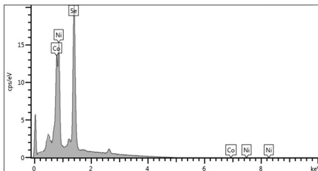
**Fig. S2** EDS of  $\text{CoNi}_2\text{Se}_4$  on Ni Foam
