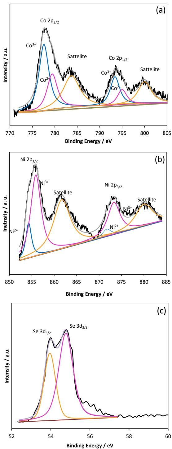
**Fig. S5** XPS of as-synthesized  $\text{CoNi}_2\text{Se}_4\text{-rGO}$  (Ni 2p, Co 2p and Se 3d).
