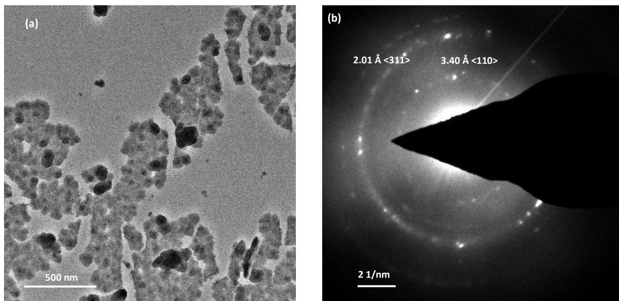
**Fig. S4** TEM image (a) and SAED pattern (b) of CoNi<sub>2</sub>Se<sub>4</sub> catalyst.
