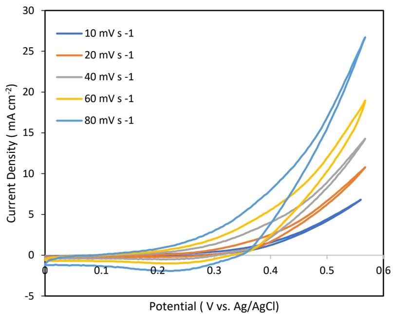
**Fig. S6** Cyclic voltammetry of reduced graphene oxide on Ni Foam at various scan rates at presence of 0.1 mM glucose.
