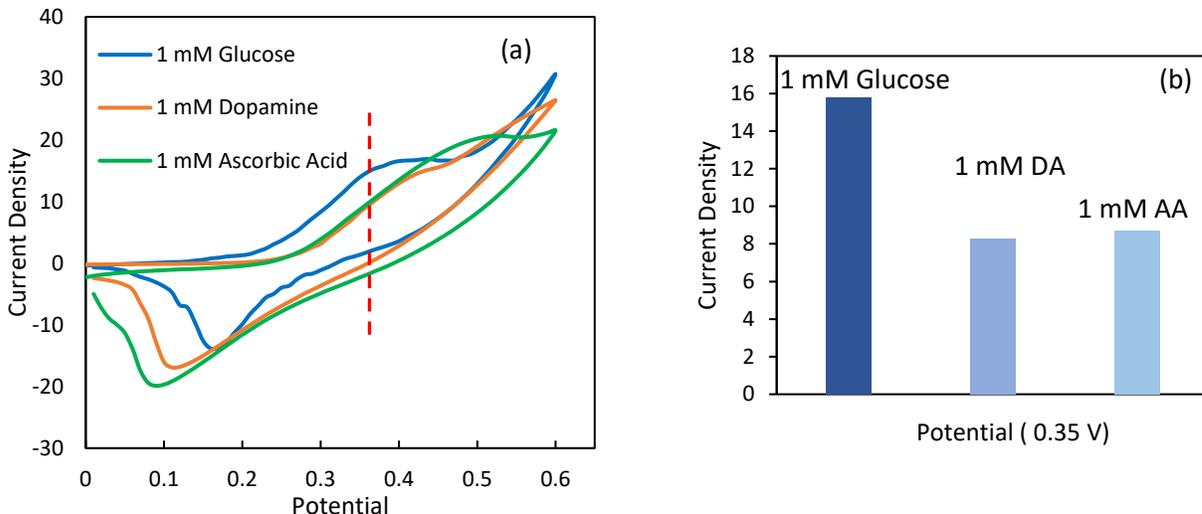
Figure S7. (a) CVs of CoNi<sub>2</sub>Se<sub>4</sub>-rGO@NF in presence of 1mM of Dopamine, ascorbic acid and glucose solution separately at the same potential (0.35 V) (b) current densities at 0.35 V for 1 mM glucose, 1mM dopamine or 1 mM ascorbic acid solutions. Current densities in both plots are in mA/cm<sup>2</sup>.
