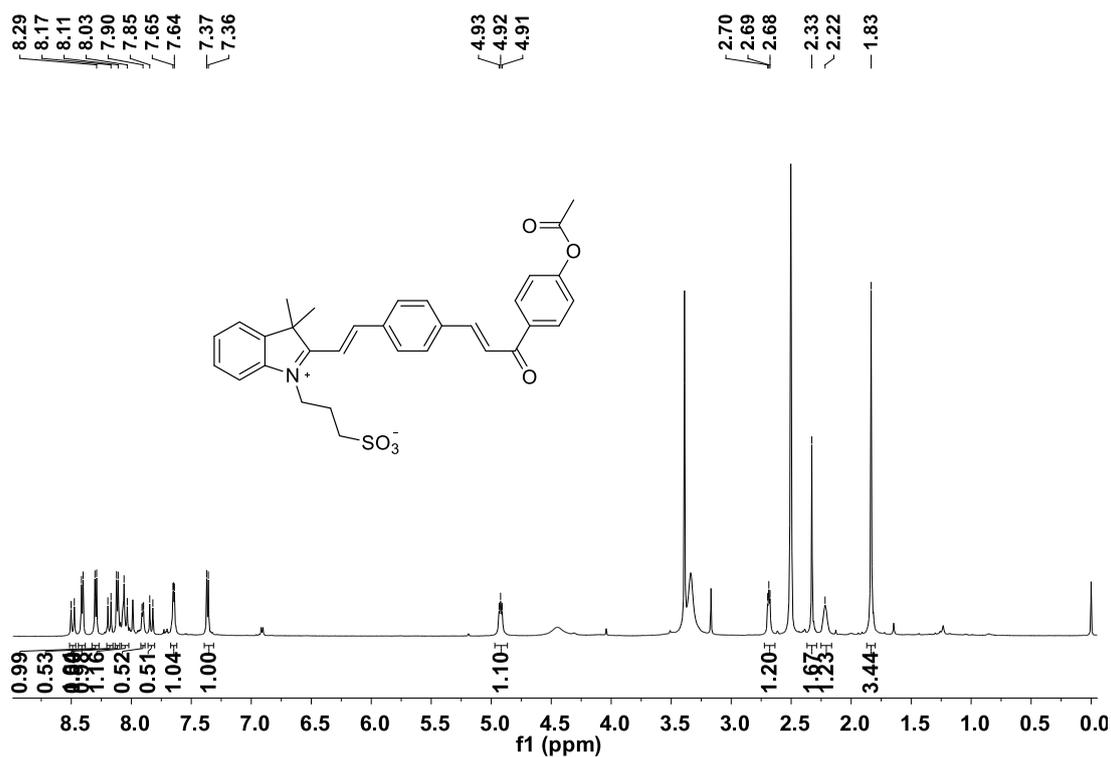
Fig. S11  $^1\text{H}$  NMR of **Hcy-Ac** in  $\text{DMSO-}d_6$
