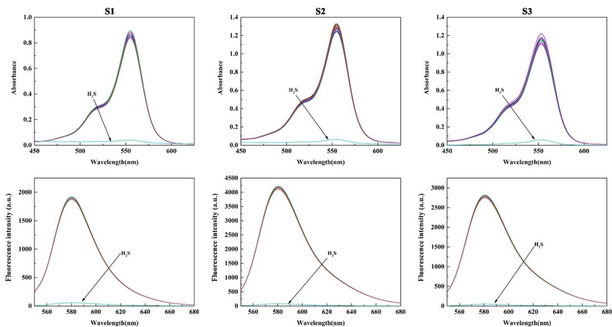
**Fig. S4** Absorption and fluorescence spectra of probe- $\text{Cu}^{2+}$  ( $10 \mu\text{mol/L}$ ) in EtOH-PBS (5:5, v/v) solution upon addition of various species ( $20 \mu\text{mol/L}$ ),  $\lambda_{\text{ex}} = 540 \text{ nm}$ .
