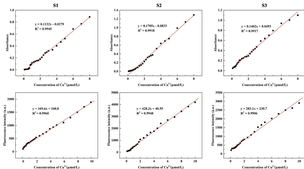
**Fig. S2** Absorption of linear of probe S1-S3 (10  $\mu\text{mol/L}$ ) with 0.1-8  $\mu\text{mol/L}$   $\text{Cu}^{2+}$ , and fluorescence intensity of linear of probe S1-S3 (10  $\mu\text{mol/L}$ ) with 0.1-10  $\mu\text{mol/L}$   $\text{Cu}^{2+}$ ,  $\lambda_{\text{ex}} = 540 \text{ nm}$ .
