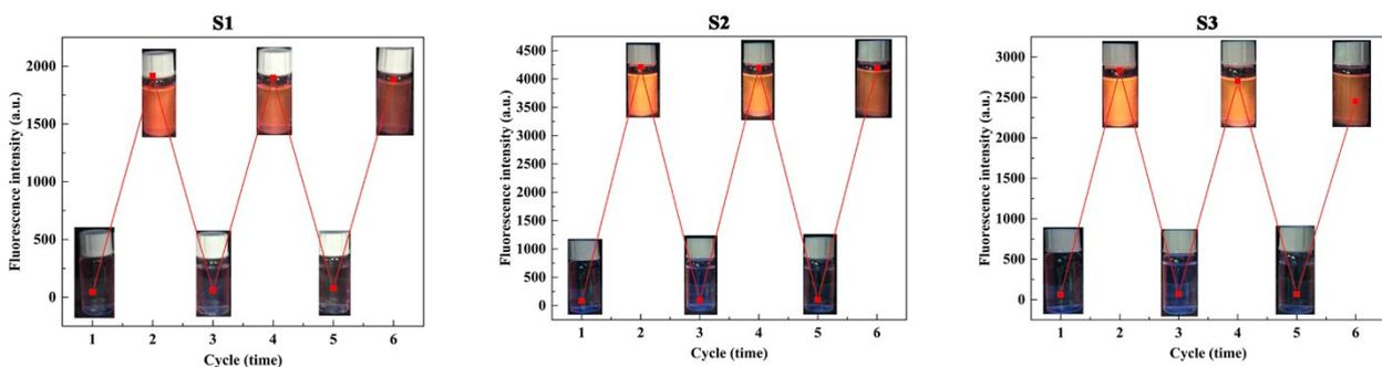
**Fig. S6** Fluorescence changes of S1-S3 at 580 nm upon alternate addition of Cu<sup>2+</sup> and H<sub>2</sub>S in the solution (5:5, v/v, EtOH: PBS, pH 7.4).
