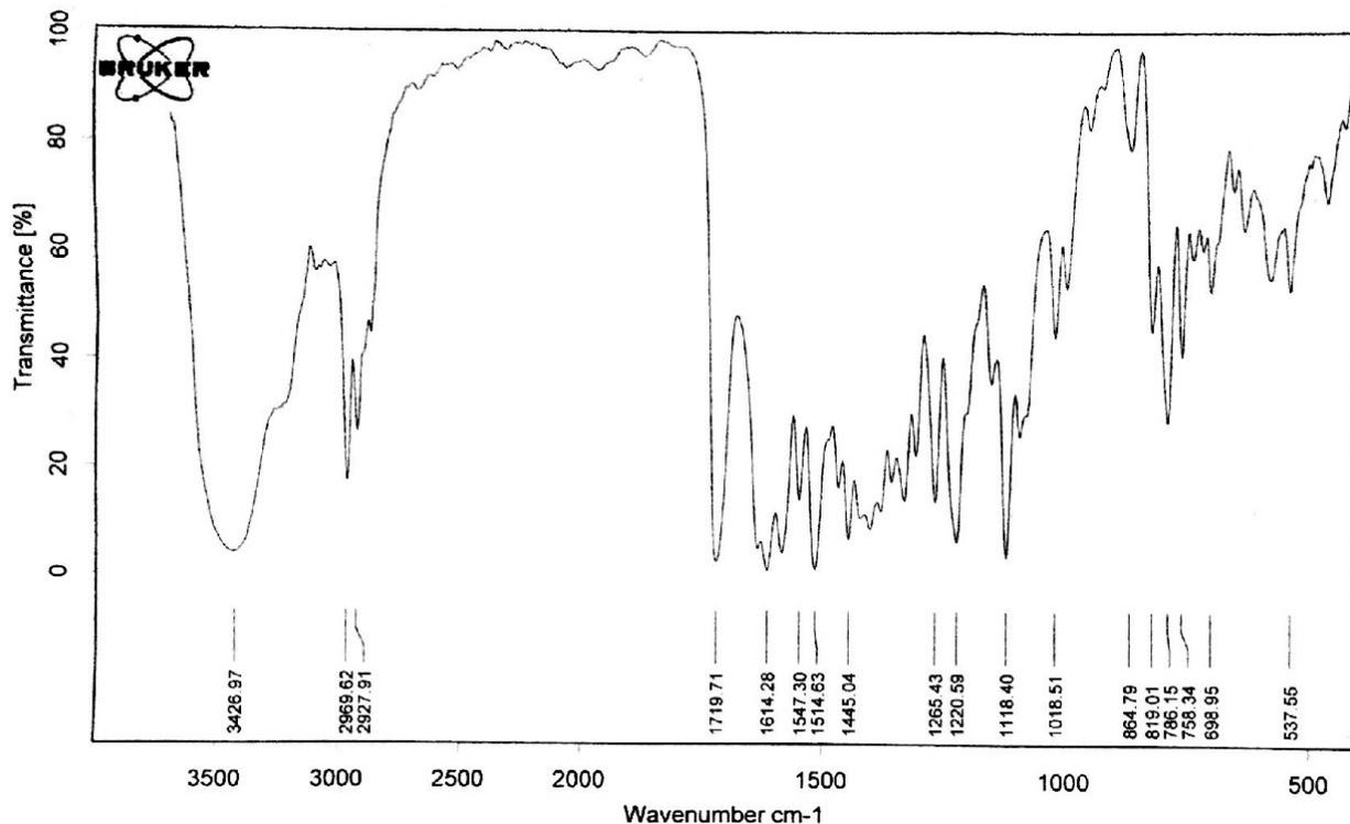
Fig. S14 IR spectrum of S1 in KBr disks.
