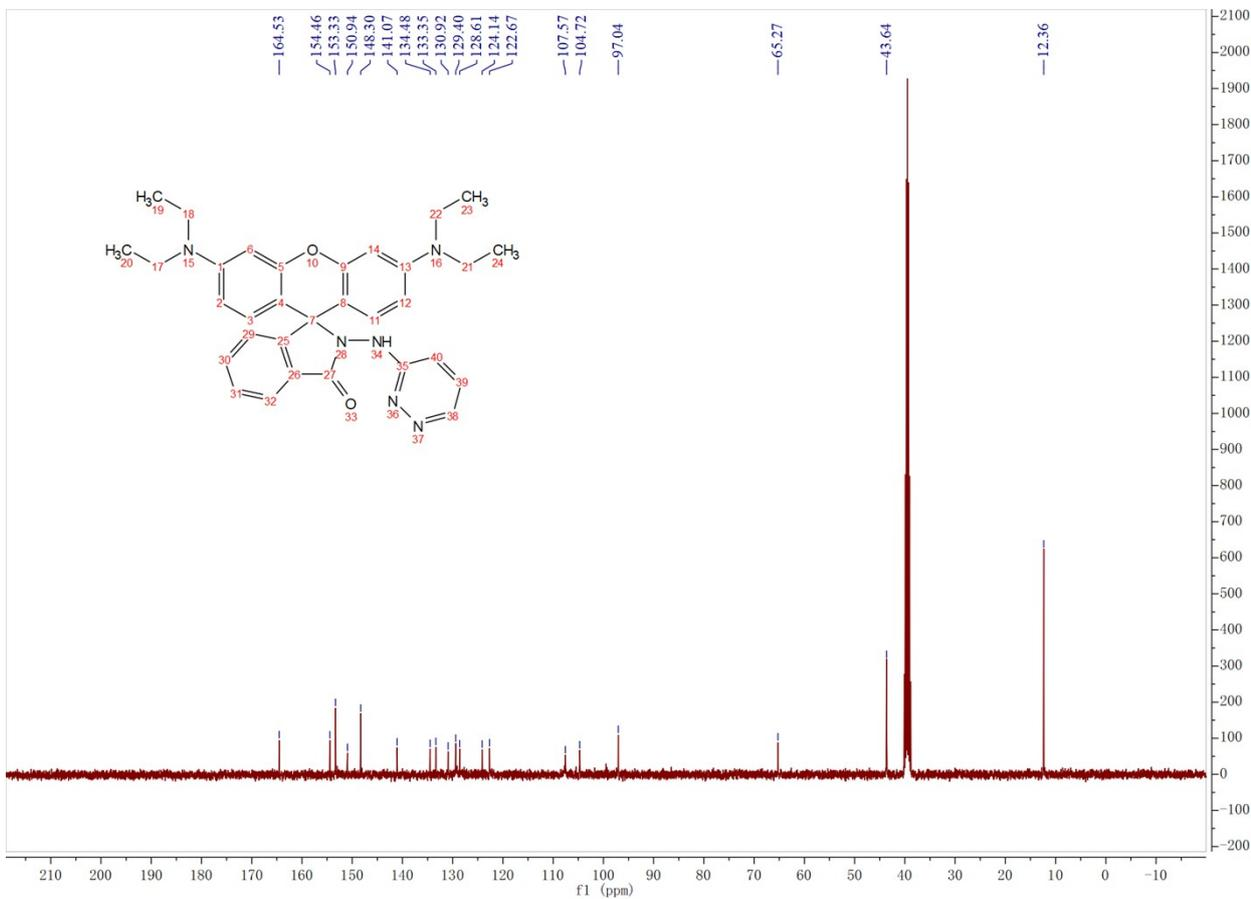
Fig. S21  $^{13}\text{C}$  NMR spectrum of S2 in DMSO.
