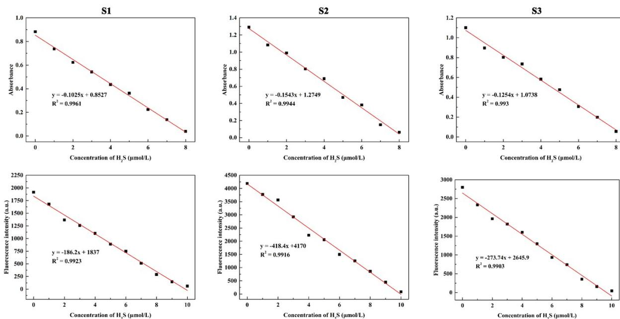
**Fig. S5** Absorption of linear of probe-Cu<sup>2+</sup> (10 μmol/L) with 0-8 μmol/L H<sub>2</sub>S, and fluorescence intensity of linear of probe-Cu<sup>2+</sup> (10 μmol/L) with 0-10 μmol/L H<sub>2</sub>S, λ<sub>ex</sub> = 540 nm.
