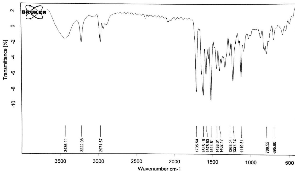
Fig. S22 IR spectrum of S3 in KBr disks.
