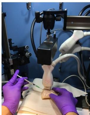
**Figure S19.** Experimental setup for *ex vivo* PA imaging.
