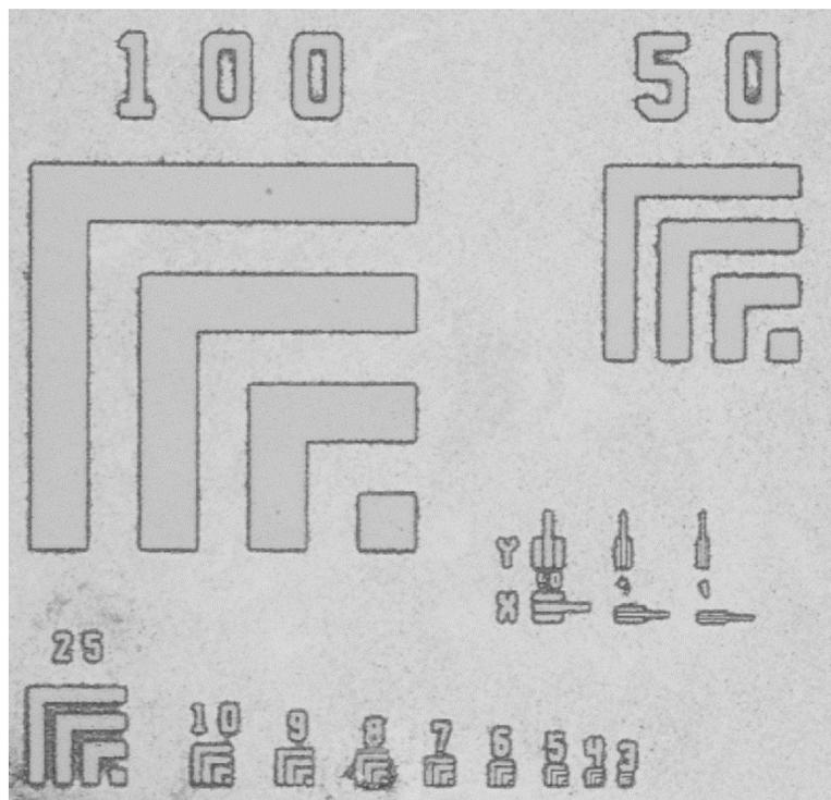
**Figure S5:** High resolution structures that can be formed using photolithography. The lower panel shows a test mask showing that features down to 10 μm can be easily formed.
