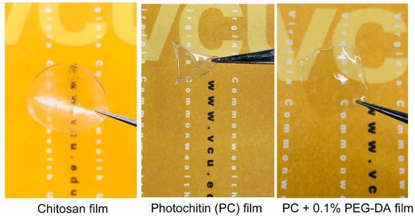
**Figure S3:** Photochitin films are optically transparent and strong (middle). However, the addition of a small amount (0.1% w/w) of PEG-DA enabled the formation of robust films which are easier to handle.
