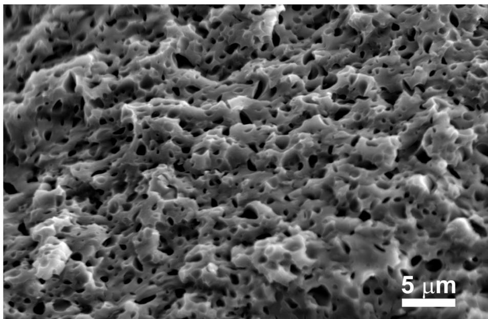
**Figure S8:** SEM image showing the porous surface of the 3D photochitin hydrogels.
