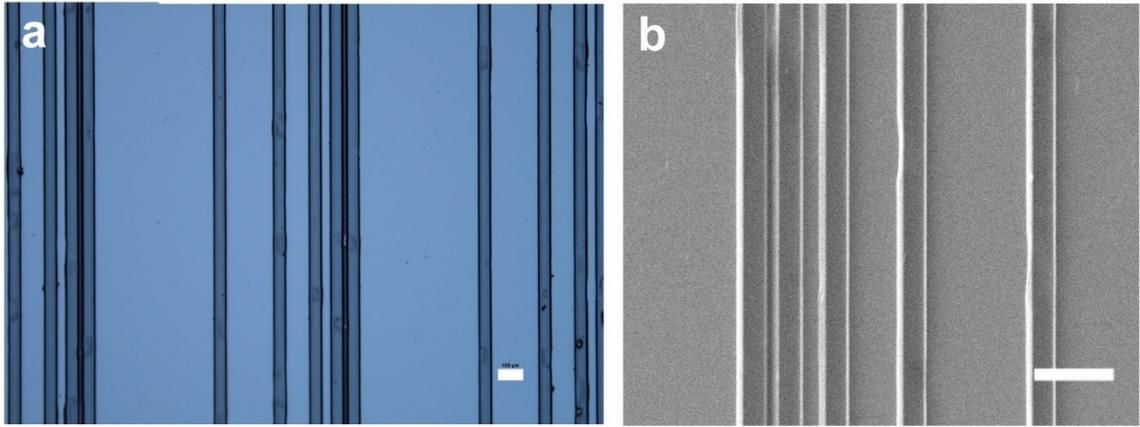
**Figure S7:** Gradient architectures used in the cell culture experiments. (L) Optical image and (R) SEM image. Scale bar = 100  $\mu\text{m}$  on both images.
