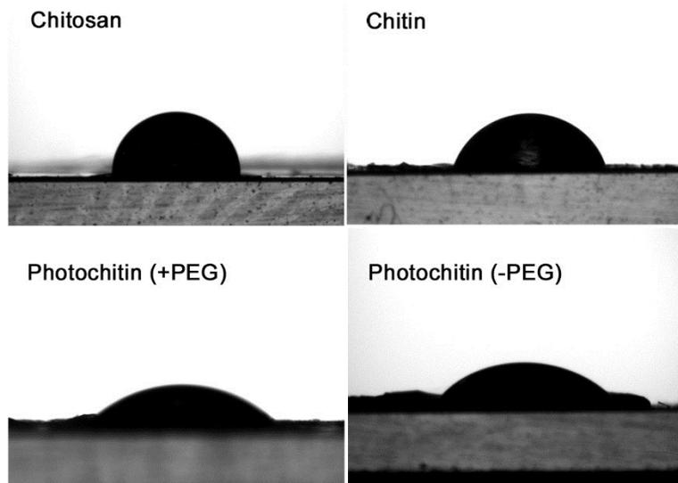
**Figure S4:** Contact angle measurements showing droplet on top: chitosan and chitin films. Bottom: photochitin (with 0.1% PEG-DA) films and photochitin (with no PEG-DA)
