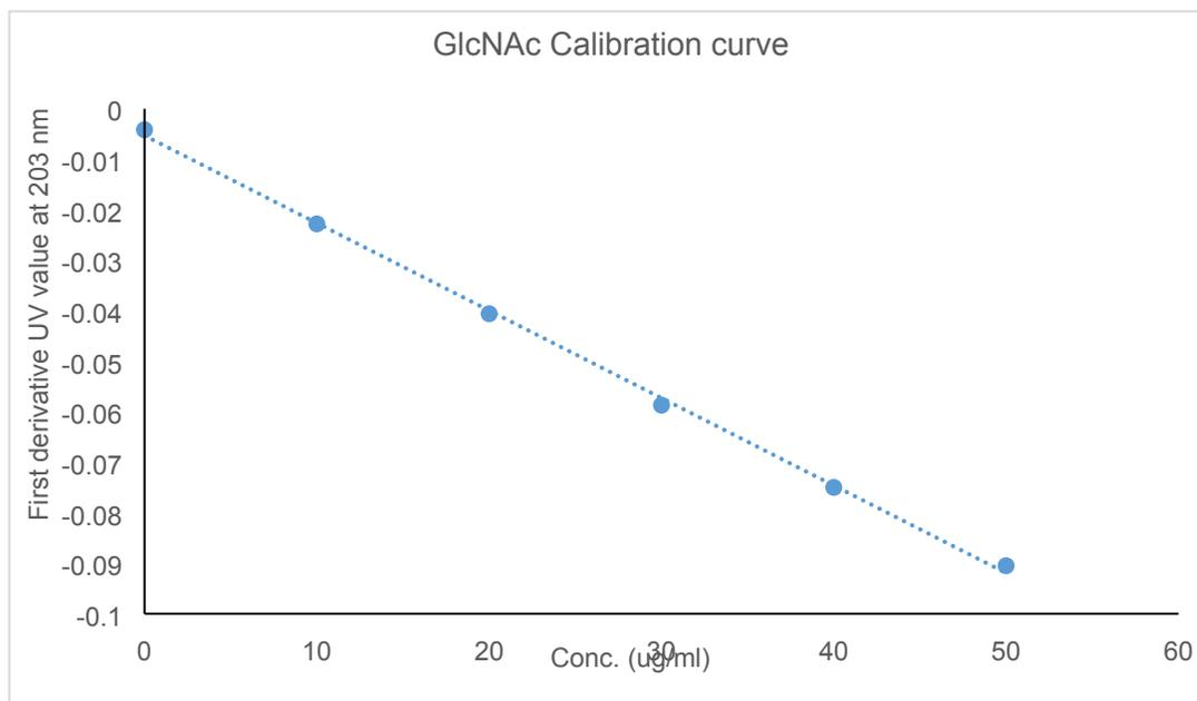
Solutions in concentrated phosphoric acid at concentration 5 mg/ml was prepared by mixing chitin and photochitin (PC) in 85% phosphoric acid at 60°C for 40 mins. The solution was then diluted 100 times using DI water and placed in the oven at 60°C for 40 mins. The first derivative values at 203 nm of the samples were obtained. Chitosan was not tested in this method since the GlcNAc is very low (as expected). The amount of GlcNAc was determined using the calibration graph:
