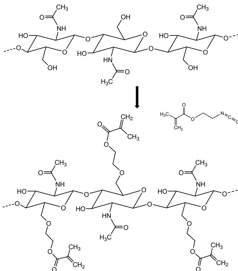
**Figure S1:** Reaction scheme of chitin with 2-isocyanatoethylmethacrylate to form photoreactive chitin.
