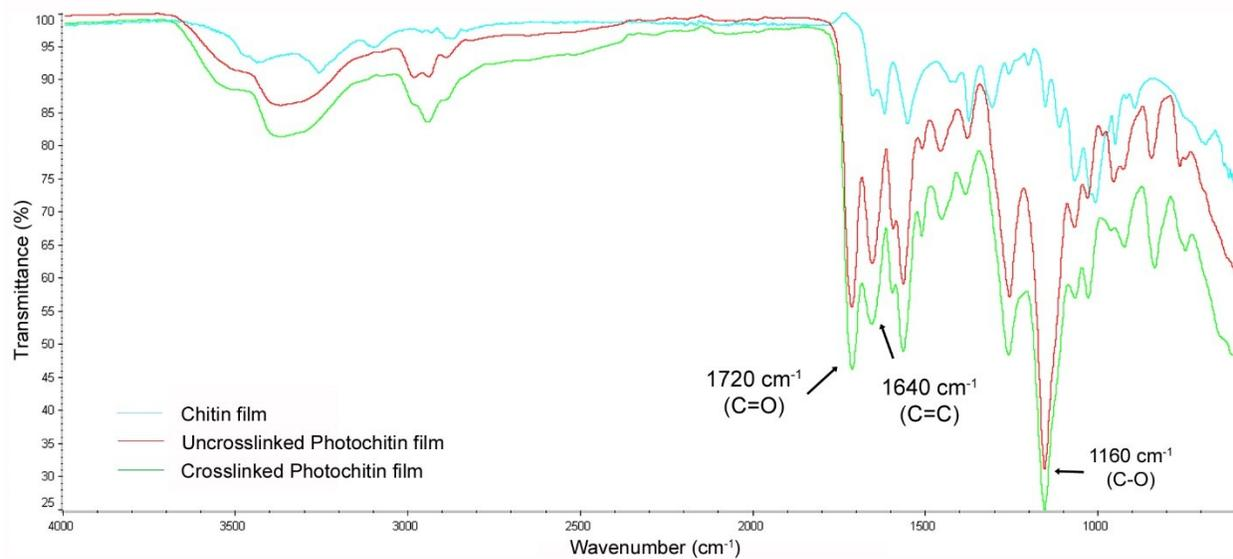
**Figure S2:** FTIR analysis to confirm the conjugation of photoreactive groups on the chitin.
