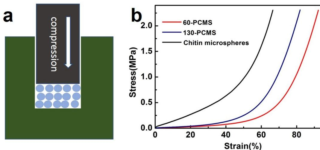
**Figure S4.** Schematic diagram of compressive test of the chitin microspheres and PCMS with the FTIR Infrared compression mold (a); Typical compressive stress – strain curves of chitin microspheres and PCMS with different pore size (b).
