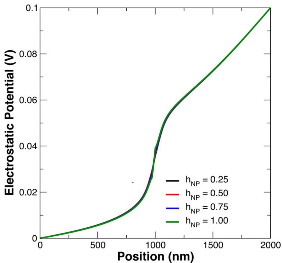
**Figure S2.** Variation of the electrostatic potential with particle hardness, calculated from PNP. Slight variation is observed near 1000 nm, where the particle is located, but the changes are subtle with  $h_{NP}$ .
