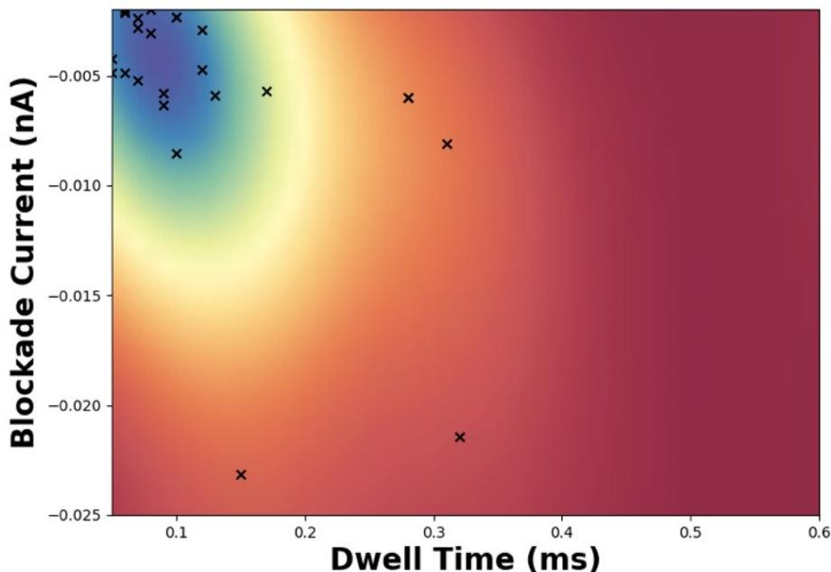
**Figure S4.** Translocation characteristics of 35 nm phytyglycogen nanoparticles through a 40 nm diameter nanochannel. The 2D histogram for  $n = 29$  events shows an average dwell time of 0.15 ms and an average blockade current of 0.010 nA.
