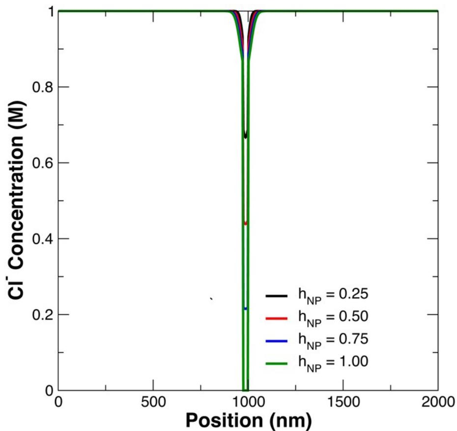
**Figure S3.** Concentration of chloride ions in the channel as a function of vertical position. The nanoparticle is located in the center of the system at 1000 nm. As the hardness of the nanoparticle decreases, the concentration of ions in the channel increases, resulting in a lower value for the blockade current.
