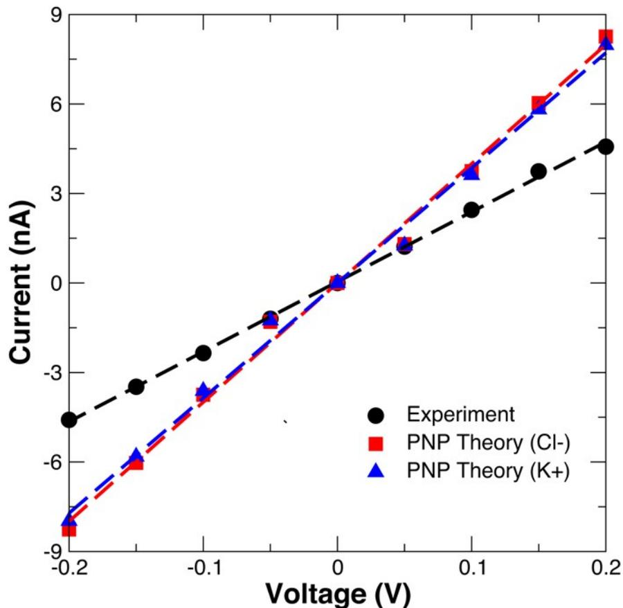
**Figure S1.** I-V characteristics of a  $d_p = 80$  nm nanochannel. The points correspond to experimental measurements (circles), calculations using the PNP framework (squares) for the anion (red) and cation (blue).
