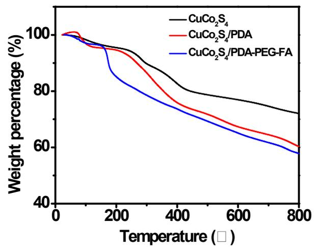
Figure S3. TGA analysis results for  $\text{CuCo}_2\text{S}_4$ ,  $\text{CuCo}_2\text{S}_4/\text{PDA}$  and  $\text{CuCo}_2\text{S}_4/\text{PDA-PEG-FA}$ .
