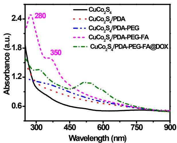
Figure S2. UV-vis-NIR absorption spectra of CuCo<sub>2</sub>S<sub>4</sub>, CuCo<sub>2</sub>S<sub>4</sub>/PDA, CuCo<sub>2</sub>S<sub>4</sub>/PDA-PEG, CuCo<sub>2</sub>S<sub>4</sub>/PDA-PEG-FA and CuCo<sub>2</sub>S<sub>4</sub>/PDA-PEG-FA@DOX (150  $\mu\text{g mL}^{-1}$  for CuCo<sub>2</sub>S<sub>4</sub>, 20  $\mu\text{g mL}^{-1}$  for the loaded DOX).
