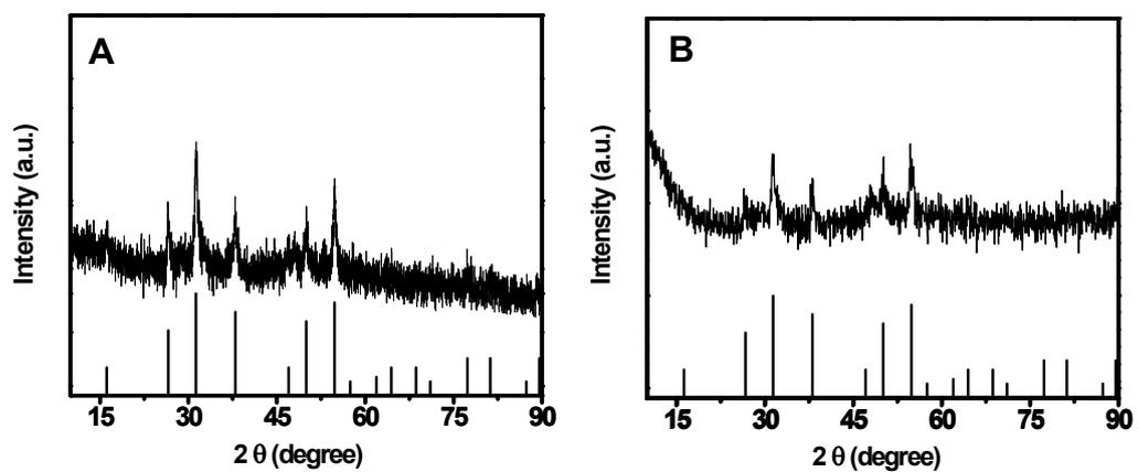
Figure S1. (A) XRD pattern of  $\text{CuCo}_2\text{S}_4$ . (B) XRD pattern of  $\text{CuCo}_2\text{S}_4$  after treated with  $10 \text{ mmol L}^{-1}$  GSH for 72 h.
