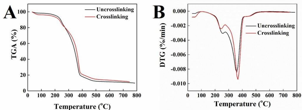
Fig. S2 (A) TGA and (B) DTG curves for uncrosslinking and crosslinking SDVGs.
