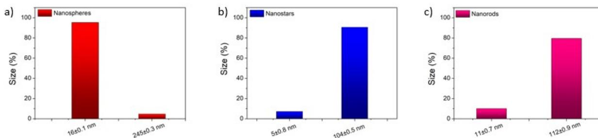
Figure S3. Mean dimensions of hydrodynamic diameters of different populations of citrate-capped (a) gold nanospheres, (b) gold nanostars, and (c) CTAB-capped gold nanorods calculated by DLS analysis.
