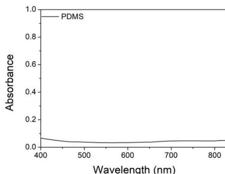
Figure S1. UV-vis absorbance spectrum of bare PDMS showing poor absorbance in the visible range.
