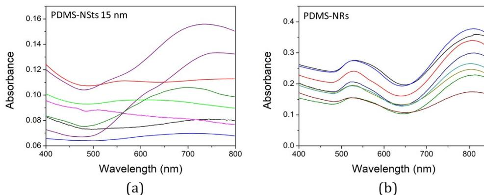
**Figure S6.** To verify the repeatability of optimized NPs deposition processes, UV-vis spectra were acquired on different NSts-decorated (a) and NRs-decorated (b) PDMS substrates. Optical density mean values and relative standard deviations were considered as indication of process repeatability.
