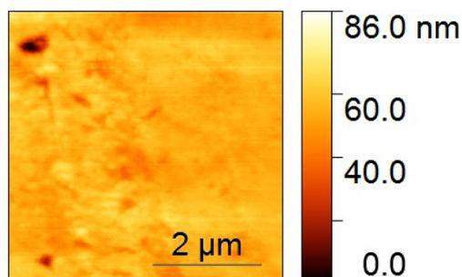
Figure S2. AFM images of the top surface of PDMS caps after releasing from the mold.
