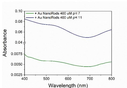
**Figure S4.** UV-Vis absorption spectrum of MPTMS-silanised PDMS flat surfaces after 12h incubation with NRs solution prepared at pH 7 (green line) and pH 11 (blue line).
