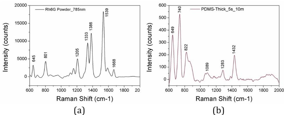
Figure S8. Raman spectra for (a) Rh6G powdered and (b) bulk PDMS (thickness > 5mm)
