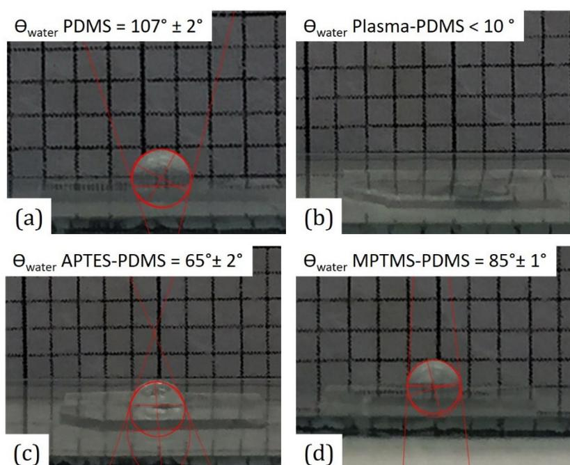
**Figure S5.** Static contact angles of water on bare PDMS (a), air plasma-treated PDMS (b), APTES-modified (c) and MPTMS-modified (d) PDMS. Ultrapure water was used as probe liquid. The contact angles were measured at room temperature by drop technique determining the contact angle based on both the circle and elliptic fitting with ImageJ dedicated plugin. Droplets of  $5 \div 10 \mu\text{l}$  were gently dispersed on the surfaces and measurements were repeated thrice and results were averaged.
