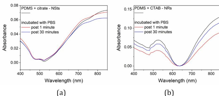
**Figure S7.** UV-vis spectra of NSts-decorated (a) and NRs-decorated (b) PDMS substrates acquired before and after incubation (from 1 minute till 30 minutes) with PBS buffer solution used for A $\beta$  protein dilution.
