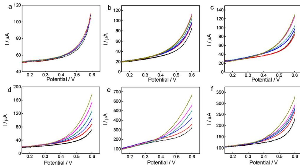
**Figure S7.** Cyclic Voltammetry (CV) for (a) MUA/AuNPs/PTFE/CP, (b) C16/AuNPs/PTFE/CP, (c) C8/AuNPs/PTFE/CP, (d) C12/AuNPs/PTFE/CP in 0.1 M, pH 7.4 PB in the presence of various  $\beta$ -D-glucose concentrations: 0 to 50 mM (scan rate:  $100 \text{ mV s}^{-1}$ ).
