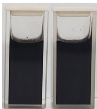
Fig. S6 Photographs of the PPy-RB NPs ( 0.1 \text{ mg}\cdot\text{mL}^{-1} ) dispersed in PBS (left) before and (right) after stored for one week.
