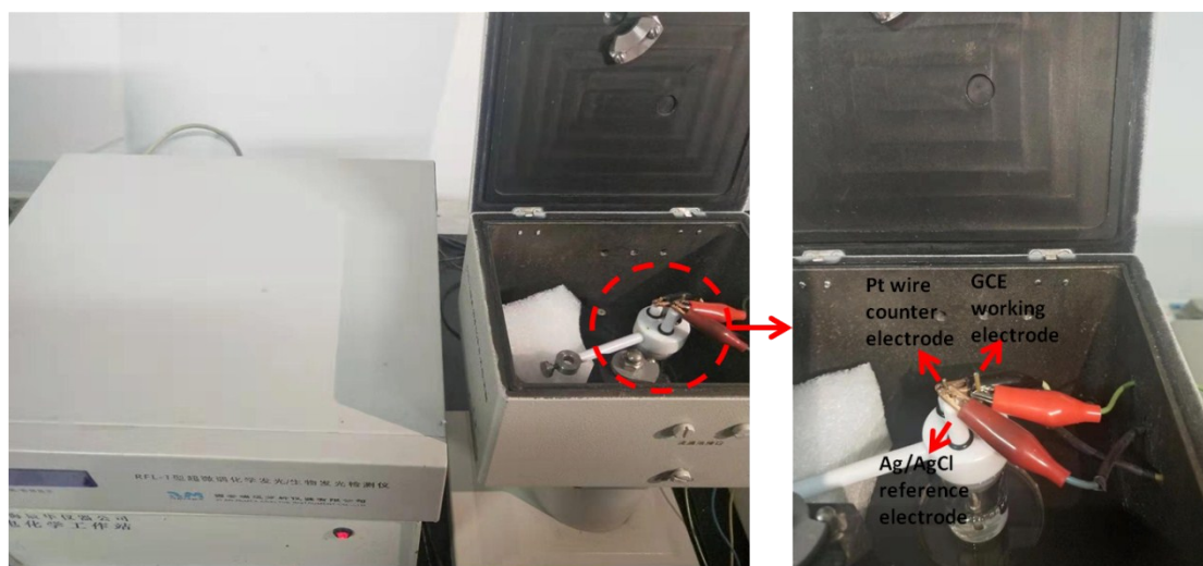
Fig. S11 The photo of experimental set-up for ECL assay
