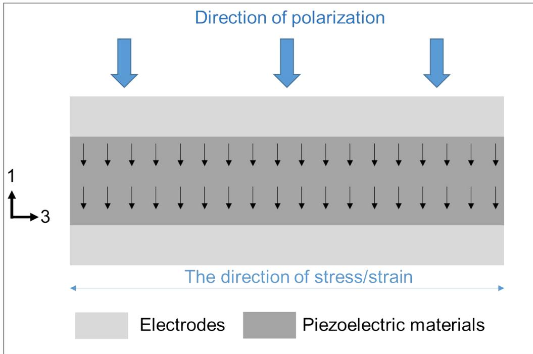
Fig S2. The schematic diagram for  $d_{31}$  mode of piezoelectric nanogenerator.
