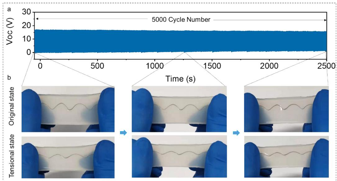
Fig S6. Durability test of the device. (a) Voc of the device that lasted for ~5000 cycles stretched by a linear motor at 2 Hz. (b) the surface of device after durability test at different times.
