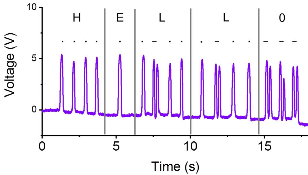
Fig S9. The word “HELLO” encoded by the voltage signal from the FSDM-NG.
