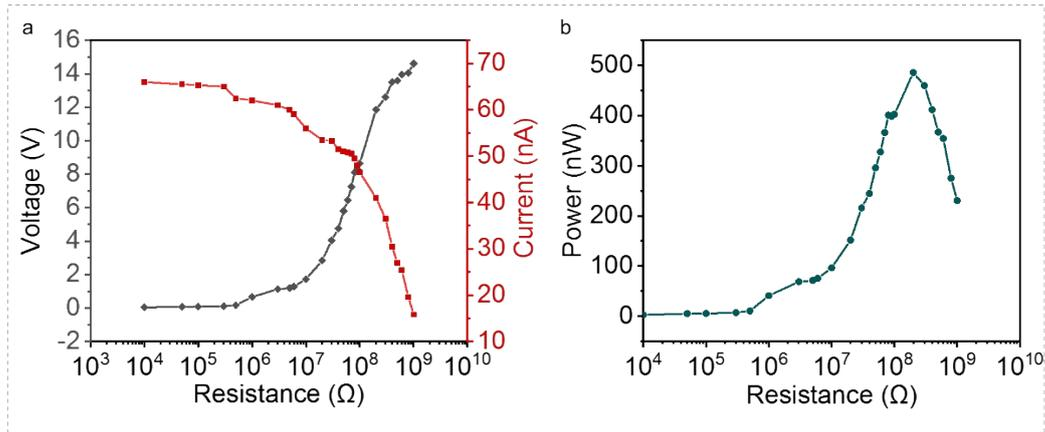
Fig S7. Characterization of output performance of the device with load resistances. (a) Voltage and current of the device at different load resistances. (b) Output power of the device at different load resistances
