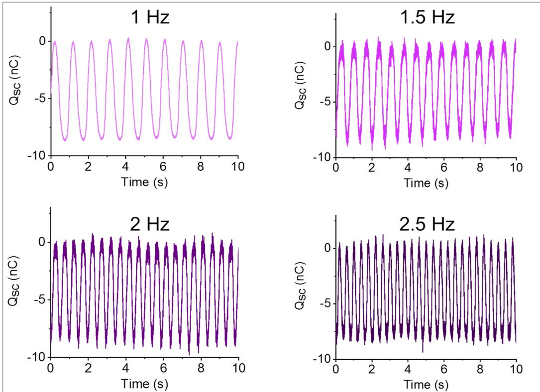
Fig S5.  $Q_{sc}$  of the FSDM-NG under different loading frequencies from 1 Hz to 2.5 Hz.
