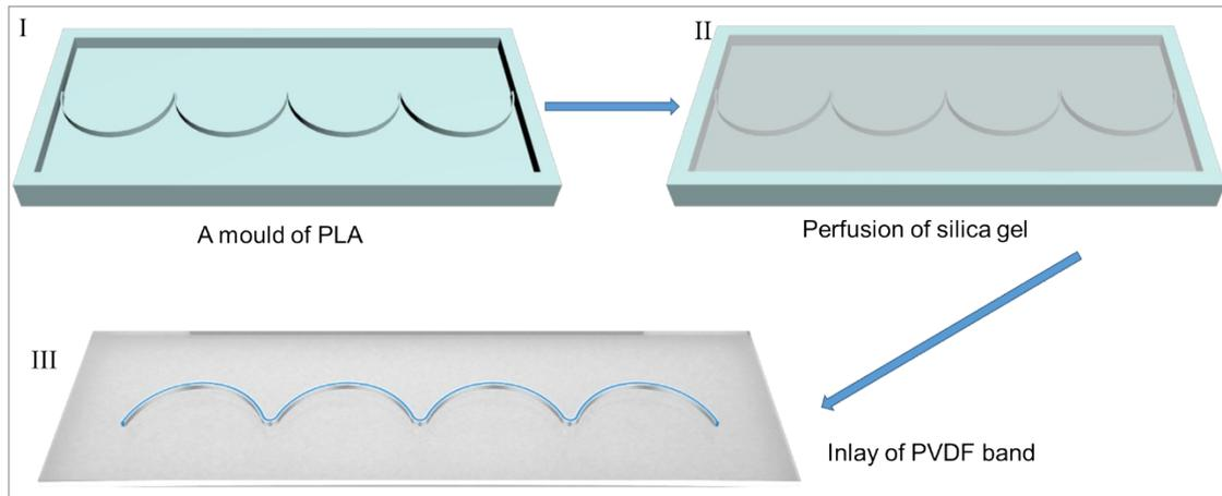
Fig S1. The fabrication process of the FSDM-NG.
