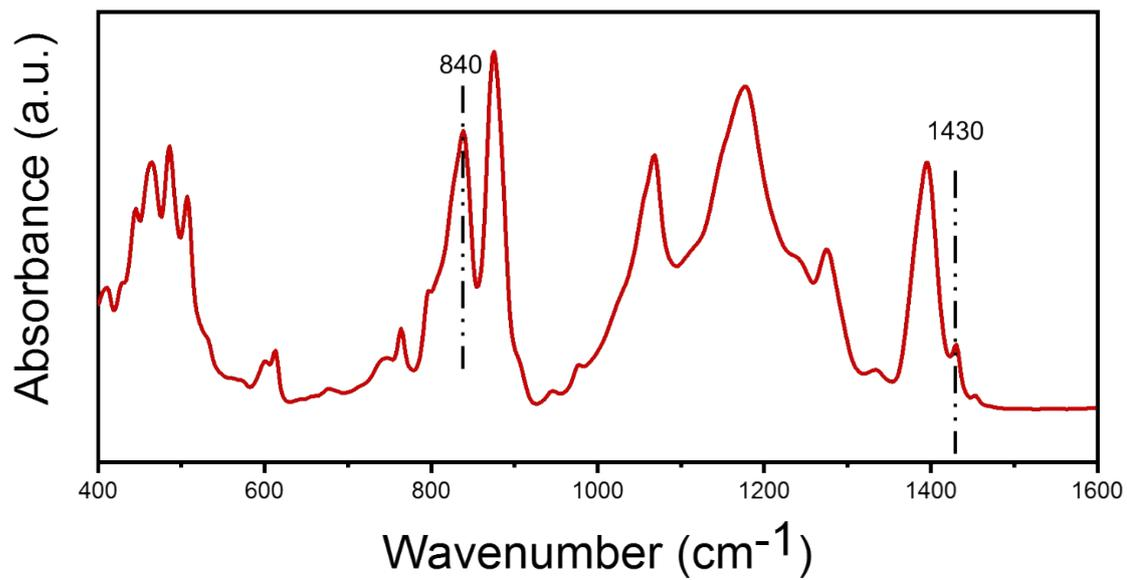
Fig S4. Fourier transform infrared spectra of the PVDF layer.
