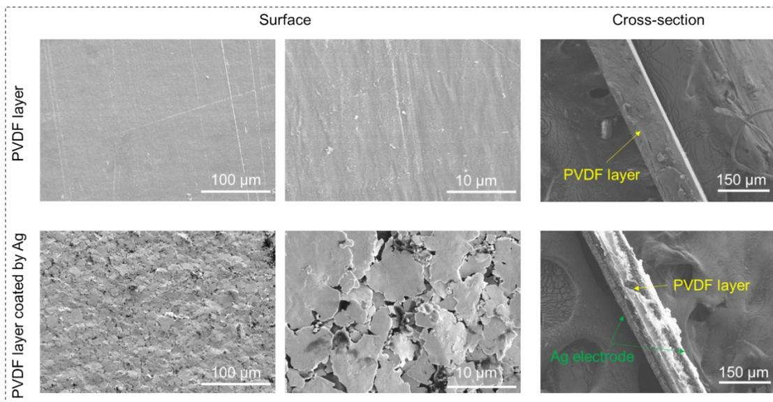
Fig S3. The SEM images for the surface and cross-section of PVDF layer with or without Ag electrode.
