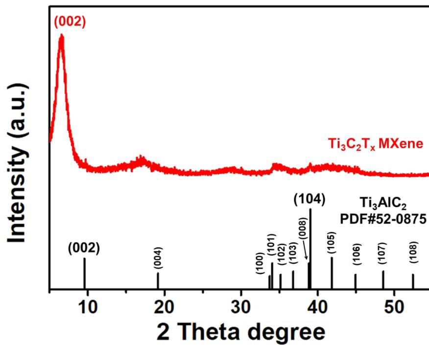
Fig. S1 The XRD patterns of  $\text{Ti}_3\text{C}_2\text{T}_x$  MXene.
