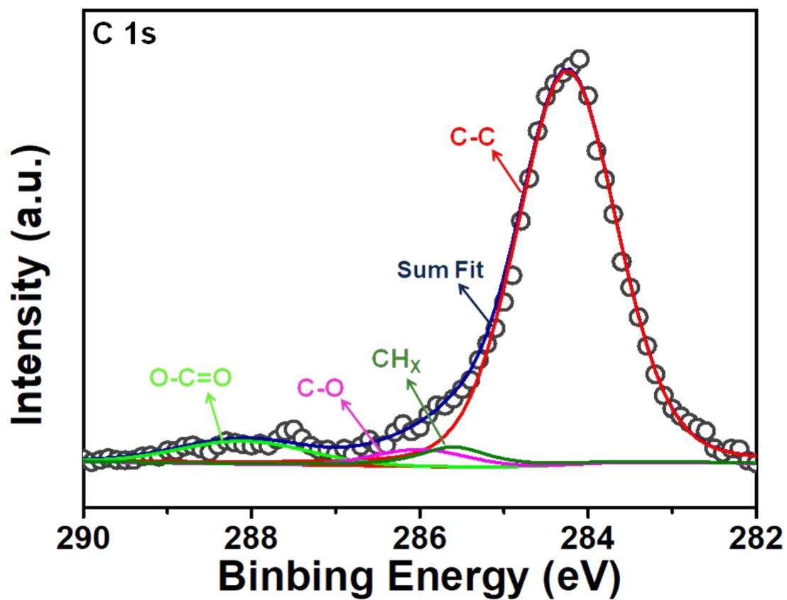
Fig. S6 The XPS narrow scan spectra of C 1s.
