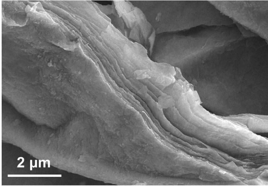
**Fig. S2** SEM image of Ti<sub>3</sub>C<sub>2</sub>T<sub>x</sub> MXene after stripping with LiF-HCl mixed solution.
