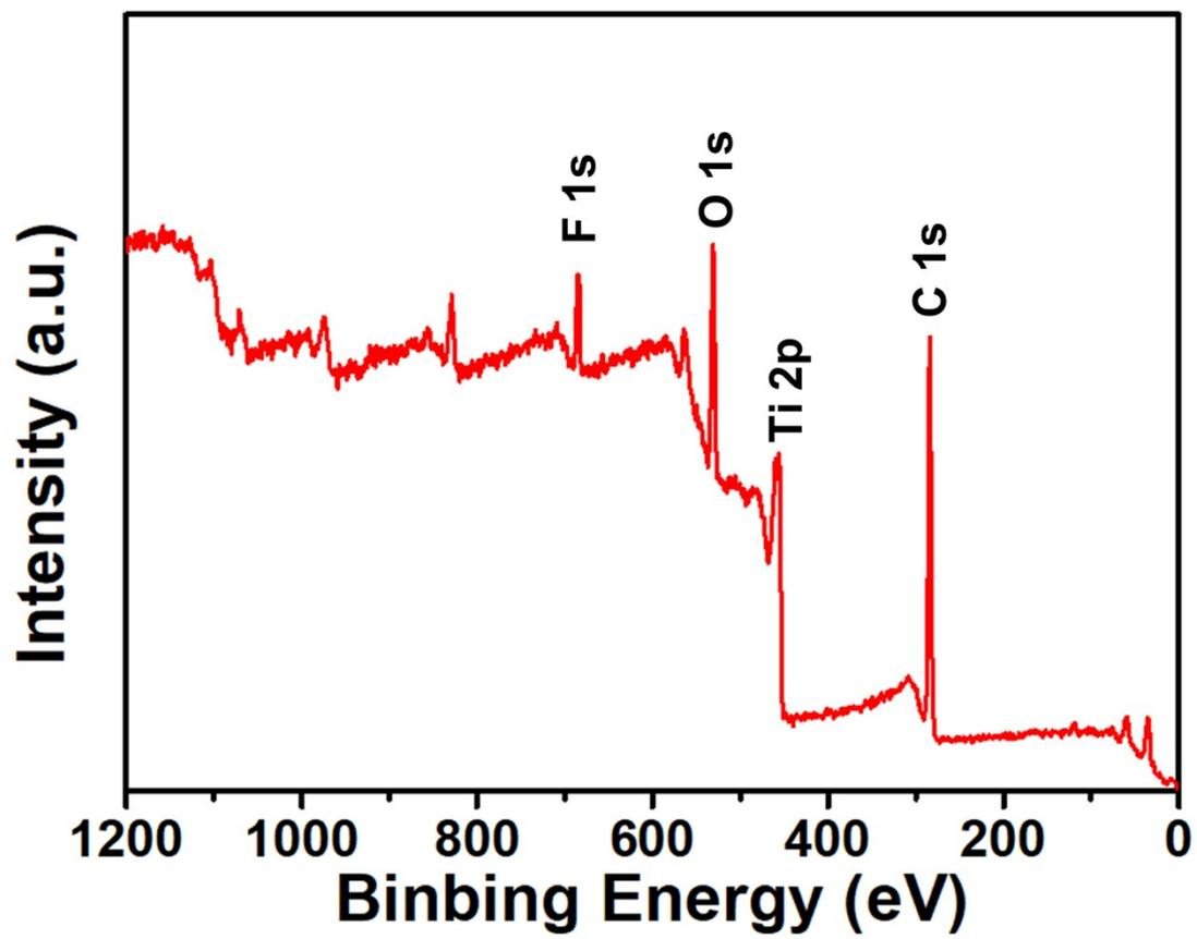
Fig. S5 The survey XPS spectra of TiO<sub>2</sub>/C-QDs.
