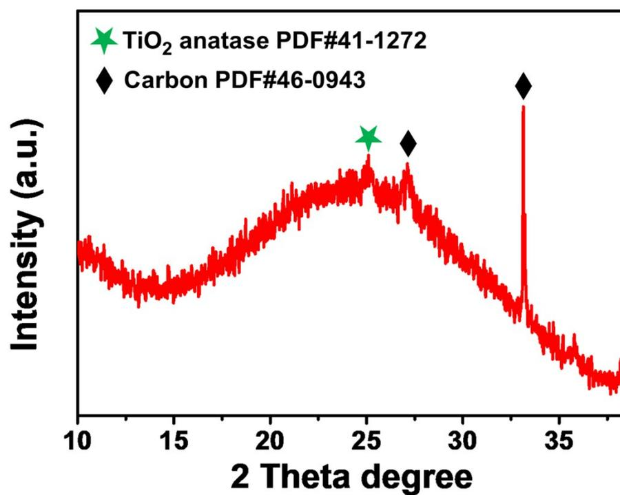
Fig. S4 XRD patterns of TiO<sub>2</sub>/C-QDs.
