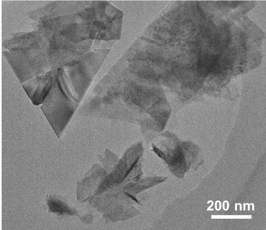
**Fig. S3** TEM image of few-layer Ti<sub>3</sub>C<sub>2</sub>T<sub>x</sub> MXene nanosheet suspension.
