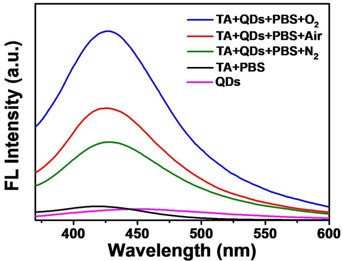
**Fig. S8** The Fluorescence spectra in different reaction systems. (TA, 0.5 mM, pH = 5,  $\lambda_{\text{ex}}$ : 315 nm,  $\lambda_{\text{em}}$ : 435 nm.)
