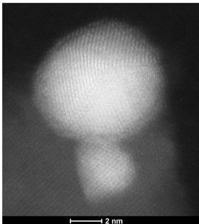
Figure S3 - HAADF-STEM image of multiple-twinned Au NP in the  $\text{Fe}_3\text{O}_4$ -Au hybrid structure for the RT sample.
