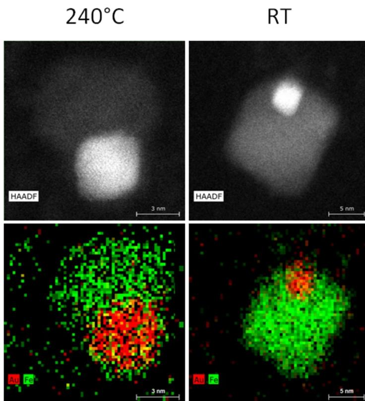
Figure S2 - HAADF-STEM images and EDX elemental maps for the  $\text{Fe}_3\text{O}_4$ -Au NPs probes taken at 240°C and after cooling to room temperature (RT). The EDX maps of Au and Fe are shown in red and green colors, respectively. Scale bars for the 240°C and RT samples are 3 and 5 nm, respectively.
