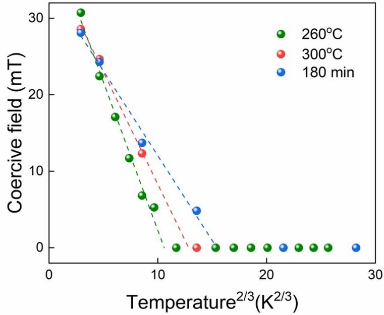
Figure S6 - Coercive field as a function of temperature<sup>2/3</sup> for Fe<sub>3</sub>O<sub>4</sub>-Au liquid probes (samples 260°C, 300°C and 180 min) taken from the reaction mixture during synthesis. Fits using Sharrock's equation are shown by the broken lines.
