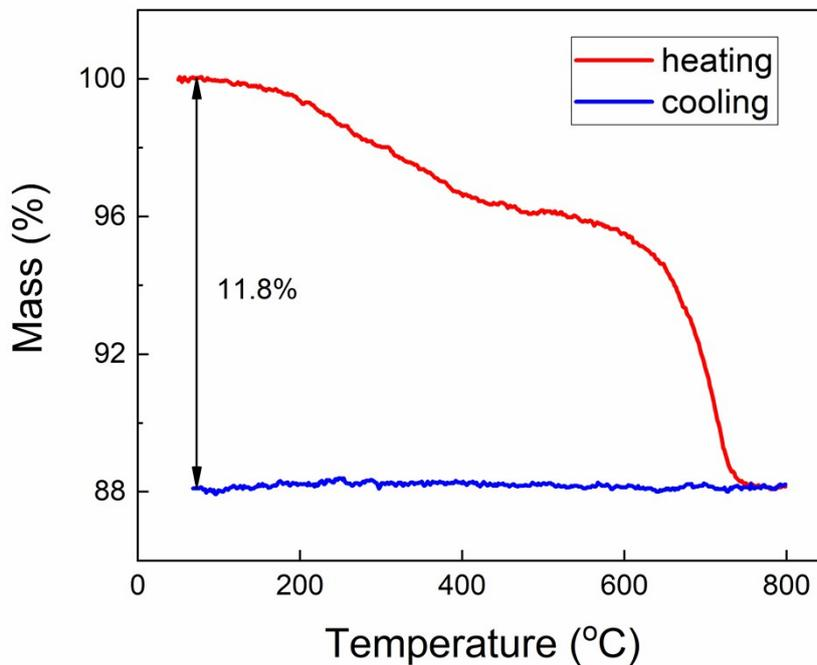
Figure S5 - Mass change of the Fe<sub>3</sub>O<sub>4</sub>-Au NPs powder (sample PS) during heating to 800°C (red line) and cooling to 30°C (blue line). Heating and cooling rate is 10°C/min.
