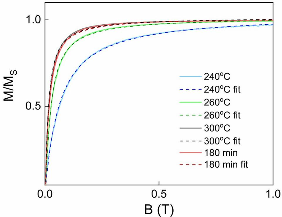
Figure S7 - Magnetization curves in the field region 0 – 1 T measured at 200 K for the probes taken from the reaction mixture at 240°C, 260°C, 300°C and 180 min. The magnetization is normalized to the saturation value. Broken lines are Langevin fits.
