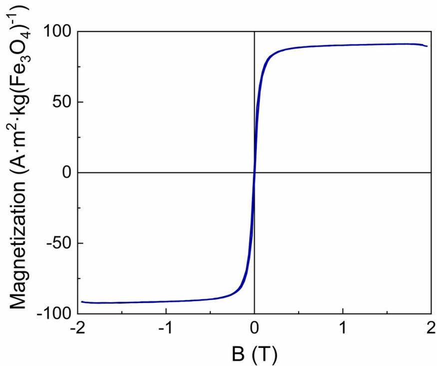
Figure S4 - Hysteresis loop for Fe<sub>3</sub>O<sub>4</sub>-Au NPs powder (sample PS) measured at room temperature. Magnetization is normalized to the mass fraction of Fe<sub>3</sub>O<sub>4</sub>.
