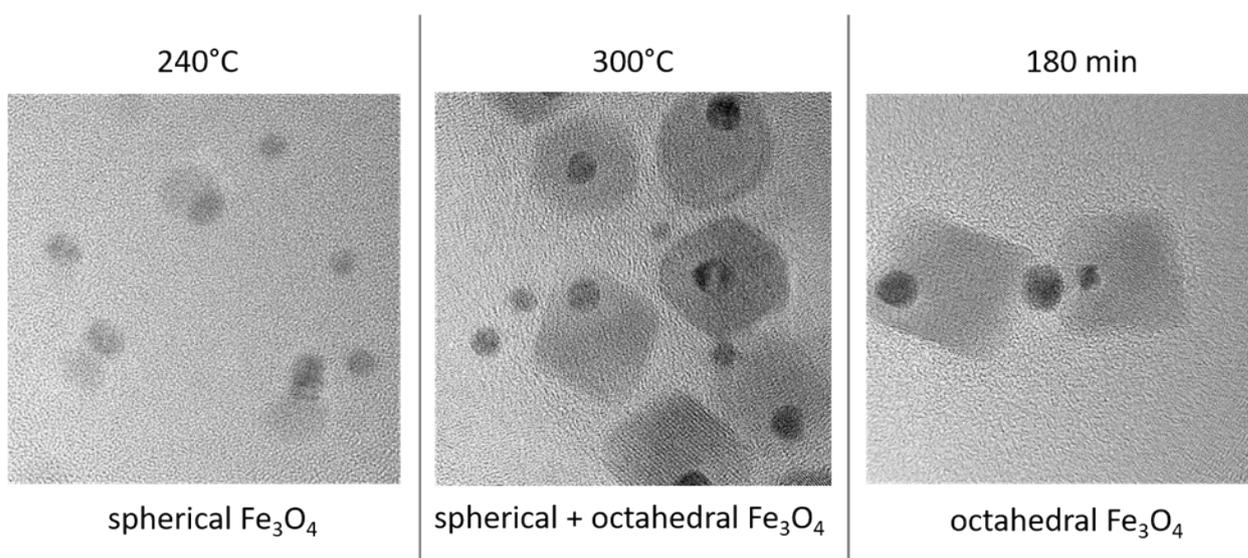
Figure S1 - Bright-field high resolution TEM of Fe<sub>3</sub>O<sub>4</sub>-Au NPs taken at different stages of the synthesis. In the heating stage, Fe<sub>3</sub>O<sub>4</sub> crystallizes (lower contrast than spherical Au NPs) at about 240°C forming spherical motifs. Upon further heating, the NPs grow rapidly and faceting towards truncated octahedra sets in at 300°C while after 180 min reflux time highly crystalline octahedra are found. Total area of all images is 50x50 nm<sup>2</sup>
