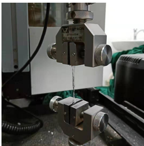
FIGURE S3. Photography of the tensile test of HAMA/PE (NAC) 4 -1% hydrogel.
