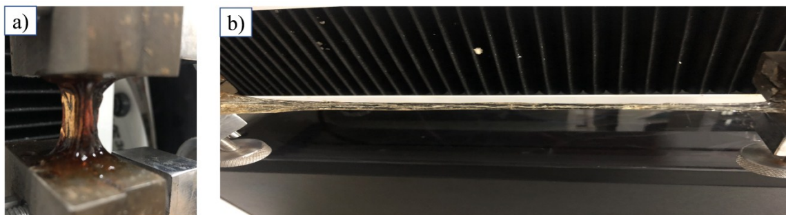
Figure S2. Optical images of OCMC-DA6/PAM5 hydrogel sample with an initial length of 20 mm (a) and a stretched length of 200 mm (b).
