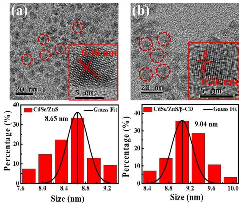
**Fig. S3** TEM images and the corresponding size distributions of green emissive CdSe/ZnS QDs (a), yellow emissive CdSe/ZnS/ $\beta$ -CD QDs (b). Inset: HRTEM images of the corresponding QDs.
