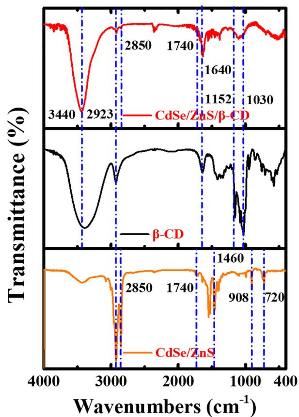
**Fig. S2** IR spectra of CdSe/ZnS QDs,  $\beta$ -CD and CdSe/ZnS/ $\beta$ -CD QDs.
