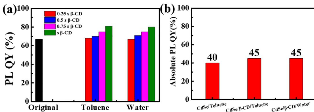
**Fig. S1** (a) Absolute PL QY of CdSe/ZnS/β-CD QDs by using different concentration of aqueous solutions of β-CD: s β-CD, 0.75 s β-CD, 0.5 s β-CD, 0.25 s β-CD. (b) Absolute PL QY of orange emissive CdSe QDs dispersed in toluene and CdSe/β-CD QDs dispersed in toluene and water.
