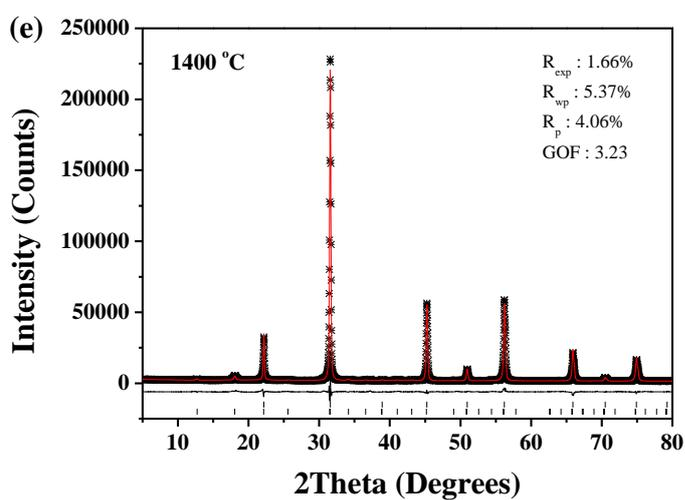
**Figure S1.** (a) Results of quantitative refinements of SZT obtained at 1100 - 1400 °C temperature range. Corresponding refinement plots at: (b) 1100 °C, (c) 1200 °C, (c) 1300 °C and (d) 1400 °C, respectively.
