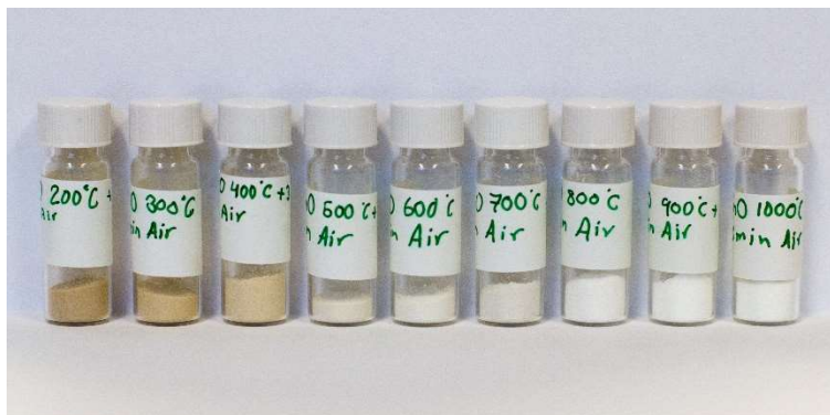
Figure S7. Photograph of ZnO powders annealed at various temperatures. Upon increase of the annealing temperature, the sample colour changed from light brown to pure white indicating increased chemical purity.
