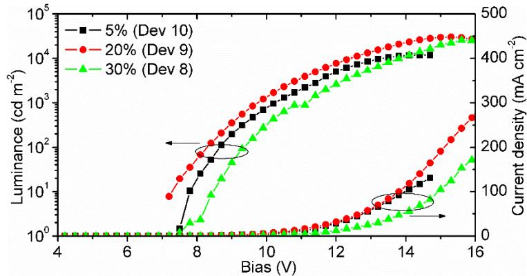
**Figure S27** Luminance-voltage and current density-voltage characteristics of devices 8-10.
