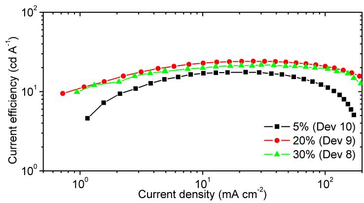
**Figure S29** Current efficiency-current density characteristics of devices 8-10.
