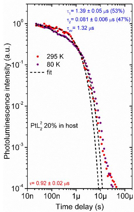
**Figure S9** Photoluminescence decay of  $\text{PtL}_2$  20% (w/w) doped in OLED host (mCP:OXD7 80:20).
