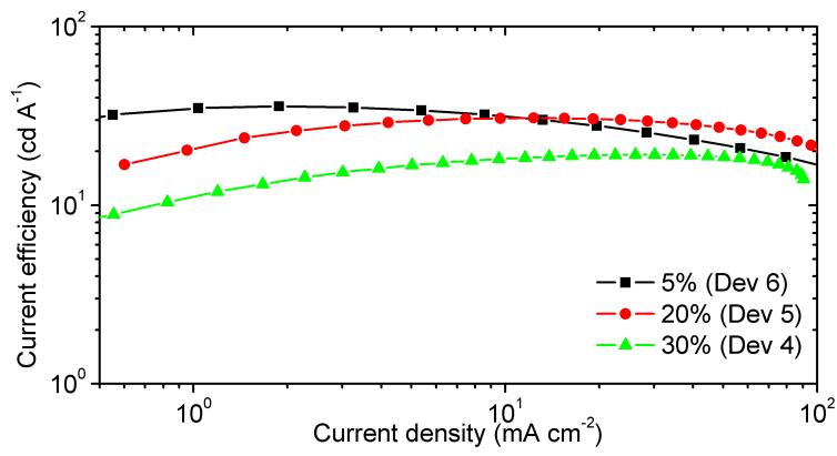
**Figure S26** Current efficiency-current density characteristics of devices 4-6.
