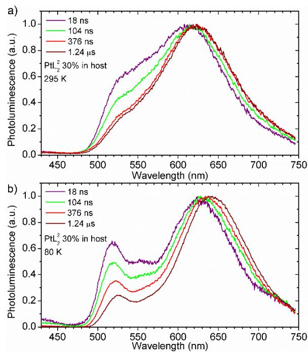
**Figure S19** Time-resolved photoluminescence spectra of  $\text{PtL}_2$  30% (w/w) doped in OLED host (mCP:OXD7 80:20).
