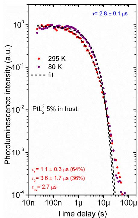
**Figure S8** Photoluminescence decay of  $\text{PtL}_2$  5% (w/w) doped in OLED host
