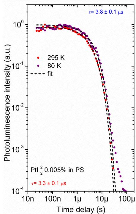
**Figure S7** Photoluminescence decay of  $\text{PtL}_2$  0.005% (w/w) doped in polystyrene (PS).
