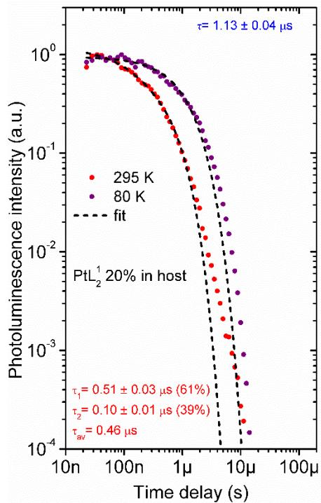
**Figure S5** Photoluminescence decay of  $\text{PtL}_2$  20% (w/w) doped in OLED host (mCP:OXD7 80:20).
