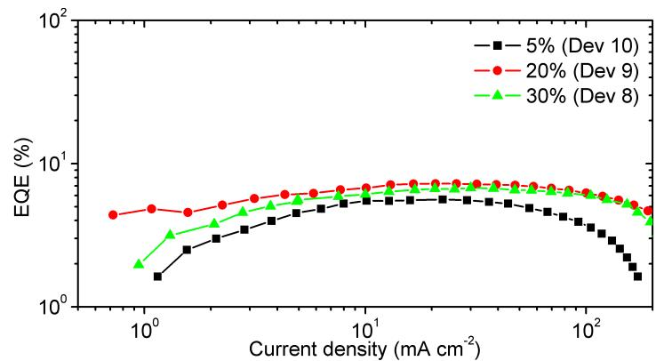
**Figure S31** External quantum efficiency (EQE)-current density characteristics of devices 8-10.
