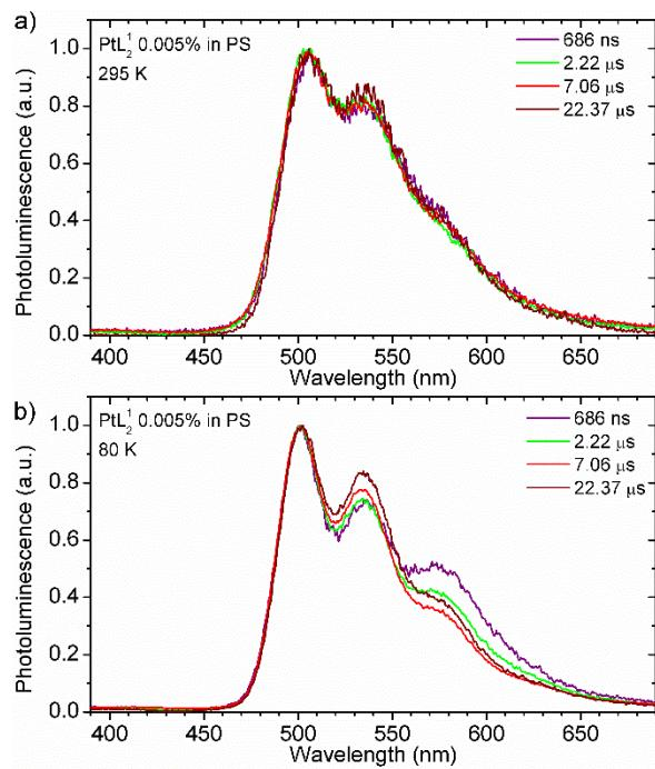
**Figure S12** Time-resolved photoluminescence spectra of PtL<sub>2</sub> 0.005% doped PS film.
