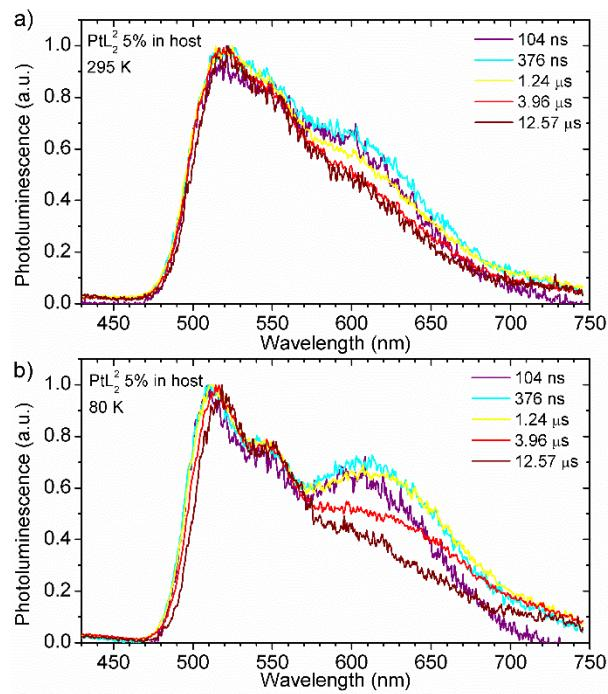
**Figure S17** Time-resolved photoluminescence spectra of  $\text{PtL}_2$  5% (w/w) doped in OLED host (mCP:OXD7 80:20).
