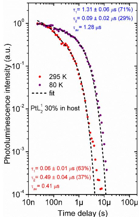
**Figure S6** Photoluminescence decay of  $\text{PtL}_2$  30% (w/w) doped in OLED host (mCP:OXD7 80:20).
