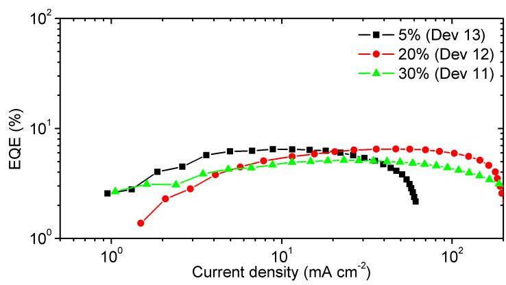
**Figure S32** External quantum efficiency (EQE)-current density characteristics of devices 11-13.
