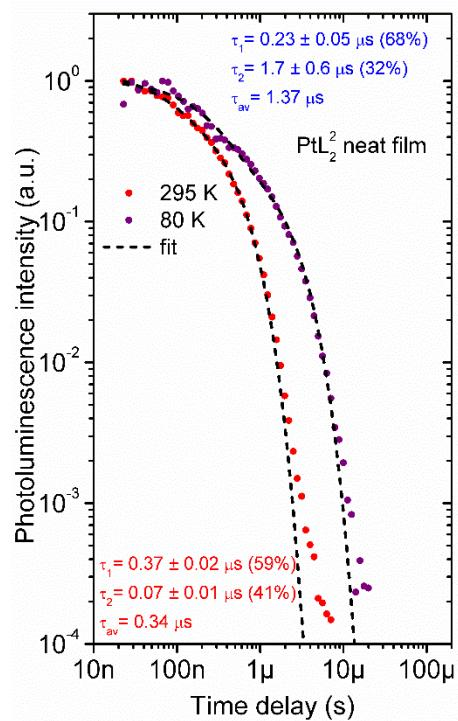
**Figure S11** Photoluminescence decay of PtL<sub>2</sub> neat film.
