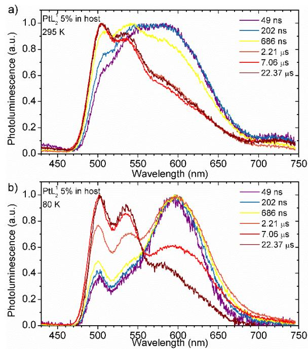
**Figure S13** Time-resolved photoluminescence spectra of  $\text{PtL}_1^1$  5% (w/w) doped in OLED host (mCP:OXD7 80:20).
