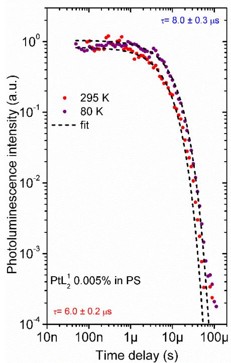
**Figure S3** Photoluminescence decay of  $\text{PtL}_2$  0.005% (w/w) doped in polystyrene (PS).
