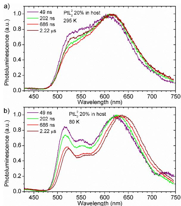
**Figure S18** Time-resolved photoluminescence spectra of  $\text{PtL}_2$  20% (w/w) doped in OLED host (mCP:OXD7 80:20).
