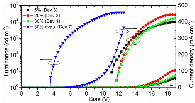
**Figure S23** Luminance-voltage and current density-voltage characteristics of devices 1-3 and 7.
