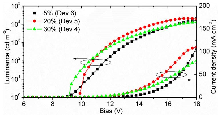
**Figure S24** Luminance-voltage and current density-voltage characteristics of devices 4-6.
