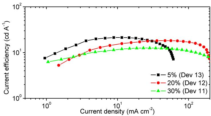
**Figure S30** Current efficiency-current density characteristics of devices 11-13.
