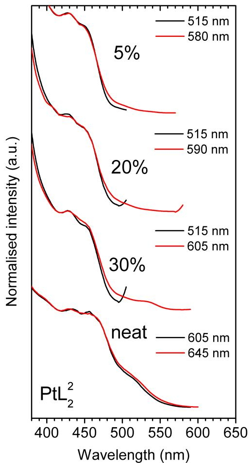
**Figure S22** Excitation spectra of thin films of  $\text{PtL}_2^2$ . The % represents the weight concentration of the emitter in mCP:OXD7 (80:20) host. The wavelength at which the emission was registered is given in the figure legend.
