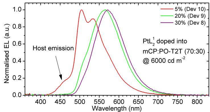
**Figure S33** Electroluminescence spectra of devices 8-10.
