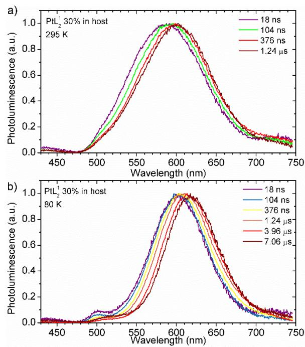
**Figure S14** Time-resolved photoluminescence spectra of  $\text{PtL}_1^1$  30% (w/w) doped in OLED host (mCP:OXD7 80:20).
