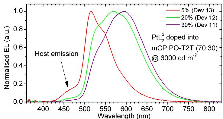
**Figure S34** Electroluminescence spectra of devices 11-13.
