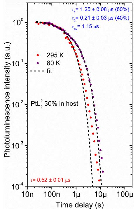
**Figure S10** Photoluminescence decay of  $\text{PtL}_2$  30% (w/w) doped in OLED host (mCP:OXD7 80:20).
