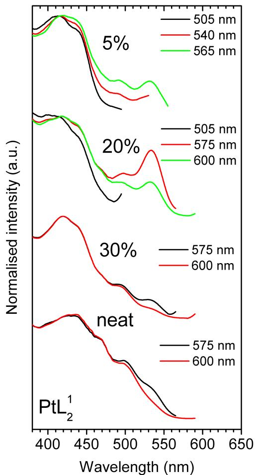
**Figure S21** Excitation spectra of thin films of  $\text{PtL}_2^1$ . The % represents the weight concentration of the emitter in mCP:OXD7 (80:20) host. The wavelength at which the emission was registered is given in the figure legend.
