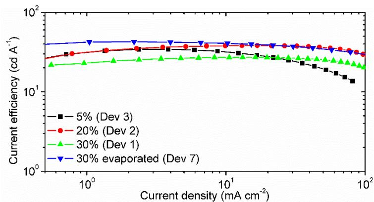
**Figure S25** Current efficiency-current density characteristics of devices 1-3 and 7.
