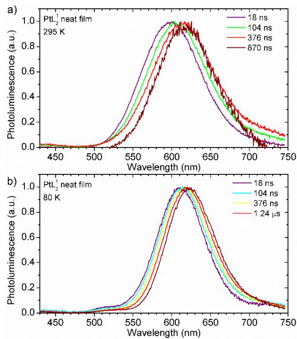
**Figure S15** Time-resolved photoluminescence spectra of  $\text{PtL}_2^1$  neat film.
