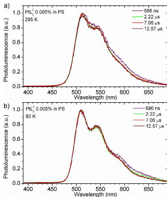
**Figure S16** Time-resolved photoluminescence spectra of  $\text{PtL}_2^2$  0.005% doped PS film.
