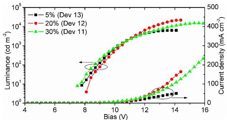
**Figure S28** Luminance-voltage and current density-voltage characteristics of devices 11-13.
