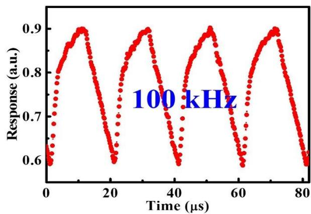
**Figure S6.** Photoresponse of the NIR detector under pulsed 1550 nm illumination with a frequency of 100 KHz.
