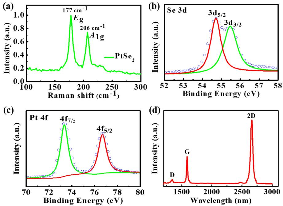
**Figure S2.** (a) Raman spectrum of the PtSe<sub>2</sub> film. The high resolution XPS spectra of (b) Se 3d and (c) Pt 4f. (d) Raman spectrum of the graphene film. The intensity ratio of  $I_{2D}:I_G \approx 2.3$ , along with the weak D-band scattering, signifies the high-quality single-layer characteristic of the graphene film.
