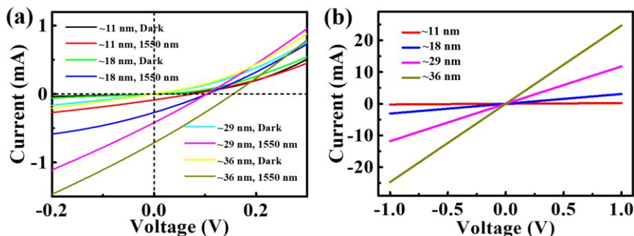
**Figure S4.** (a)  $I$ - $V$  curves of PtSe<sub>2</sub>/Ge heterojunction with different PtSe<sub>2</sub> thicknesses in dark and under 1550 nm NIR illumination. (b)  $I$ - $V$  curves of Au/PtSe<sub>2</sub>/Au structures with different PtSe<sub>2</sub> thicknesses, indicating that the sheet resistance of PtSe<sub>2</sub> layers decreases with increase in their thickness.
