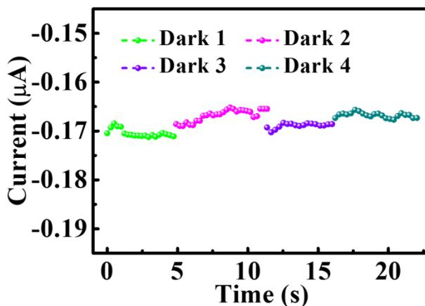
**Figure S5.** Dark currents of the PtSe<sub>2</sub>/Ge heterojunction photodetector under different NIR illuminations: Dark 1, 2, 3, 4 denote dark current under 1300, 1550, 1650 and 2200 nm illuminations, respectively.
