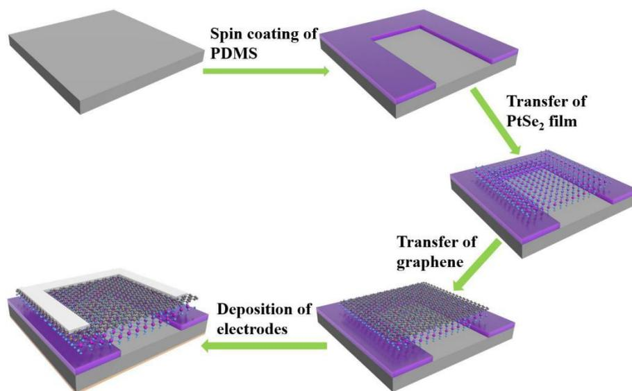
**Figure S1.** Schematic illustration of the procedures for fabrication of PtSe<sub>2</sub>/Ge heterojunction photodetector.
