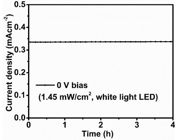
**Fig. S11** The photocurrent evolution of the MAPbBr<sub>3</sub>/MAPbBr<sub>3-x</sub>I<sub>x</sub> GHSC photodetector at 0 V bias under continuous white LED illumination of 1.45 mW cm<sup>-2</sup>.
