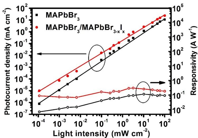
**Fig. S10** Linear dynamic range of the photodetectors based on the laminar  $\text{MAPbBr}_3$  SC and the  $\text{MAPbBr}_3/\text{MAPbBr}_{3-x}\text{I}_x$  GHSC at 0 V bias. The corresponding responsivity are shown in the figure with Y axis on the right.
