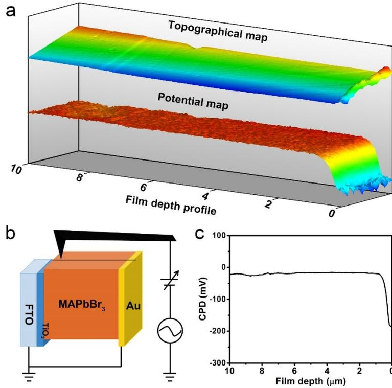
**Fig. S7** (a) AFM topography and the corresponding KPFM CPD map across the cross-section of the laminar MAPbBr<sub>3</sub> SC on TiO<sub>2</sub>/FTO substrate. (b) Schematic of cross-sectional KPFM measurement setup in short-circuit mode. 100 nm gold film was deposited on the single crystal surface and the FTO substrate by sputtering to both make well grounding. (c) CPD depth profile averaged from (a) along the lateral direction of the cross-section.
