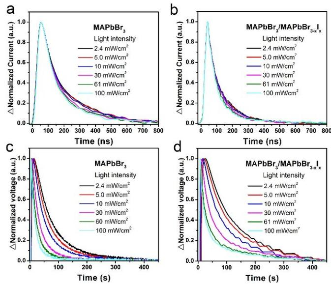
**Fig. S12** The TPC (a, b) and TPV (c, d) curves of the MAPbBr<sub>3</sub> SC and MAPbBr<sub>3</sub>/MAPbBr<sub>3-x</sub>I<sub>x</sub> GHSC devices
