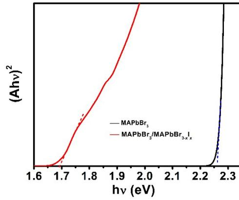
**Fig. S1** Tauc plots of the laminar  $\text{MAPbBr}_3$  SC and  $\text{MAPbBr}_3/\text{MAPbBr}_{3-x}\text{I}_x$  GHSC.
