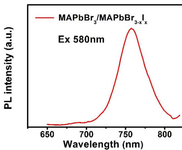
**Fig. S6** The PL spectrum of the laminar MAPbBr<sub>3</sub>/MAPbBr<sub>3-x</sub>I<sub>x</sub> GHSC under 580 nm excitation from the glass side.
