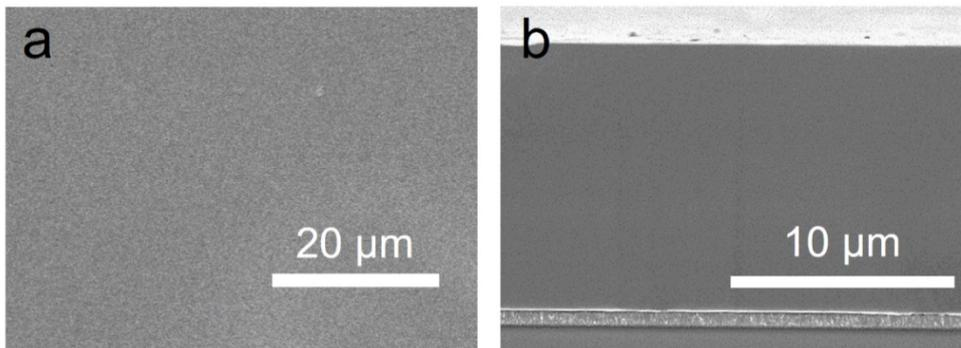
**Fig. S2** (a) The surface and (b) cross-sectional SEM images of the laminar  $\text{MAPbBr}_3$  SC.
