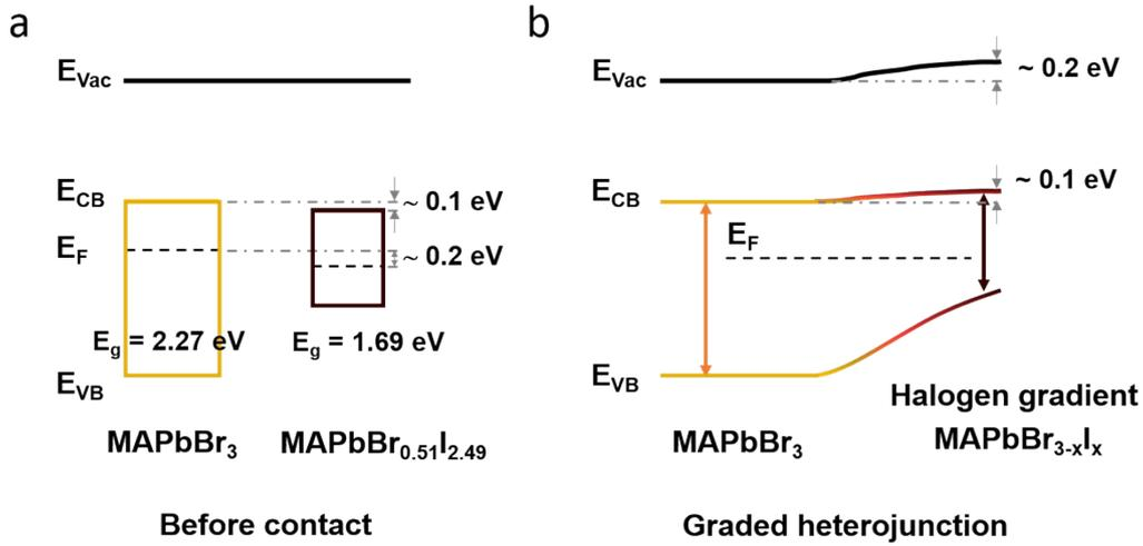
**Fig. S8** (a) The relative energy band position between the pure MAPbBr<sub>3</sub> and the iodine-rich MAPbBr<sub>3-x</sub>I<sub>x</sub> component deduced from the KPFM result and the previous reports. (b) The proposed band alignment of the MAPbBr<sub>3</sub>/MAPbBr<sub>3-x</sub>I<sub>x</sub> GHSC.
