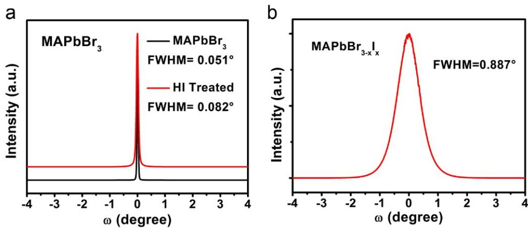
**Fig. S5** High-resolution X-ray diffraction analysis on laminar MAPbBr<sub>3</sub> SC and MAPbBr<sub>3</sub>/MAPbBr<sub>3-x</sub>I<sub>x</sub> GHSC: rocking curve of (a) the 14.97° peak of MAPbBr<sub>3</sub> and (b) the 14.26° peak of MAPbBr<sub>3-x</sub>I<sub>x</sub>.
