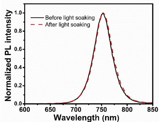
**Fig. S9** PL spectra of the laminar  $\text{MAPbBr}_3/\text{MAPbBr}_{3-x}\text{I}_x$  GHSC (excited from PVK side) before and after light soaking ( $100 \text{ mW cm}^{-2}$  from white LED) for 30 min.
