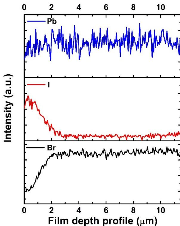
**Fig. S3** The cross-sectional EDX linescan of the laminar  $\text{MAPbBr}_3/\text{MAPbBr}_{3-x}\text{I}_x$  GHSC.
