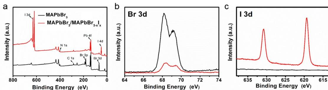
**Fig. S4** (a) XPS spectra of the laminar  $\text{MAPbBr}_3$  SC and  $\text{MAPbBr}_3/\text{MAPbBr}_{3-x}\text{I}_x$  GHSC, (b) Br 3d peak and (c) I 3d peak.
