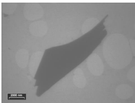
Figure S21: TEM image of the \text{Mn}_{0.73}\text{Bi}_{6.18}\text{Te}_{10} single crystal used for structure analysis.
