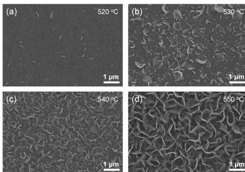
**Fig. S6** SEM images of VGPNs directly grown on SiO<sub>2</sub> substrates for growth temperature of 520 °C, 530 °C, 540 °C and 550 °C, respectively, with I<sub>RF</sub> of 400 W in 25 min.
