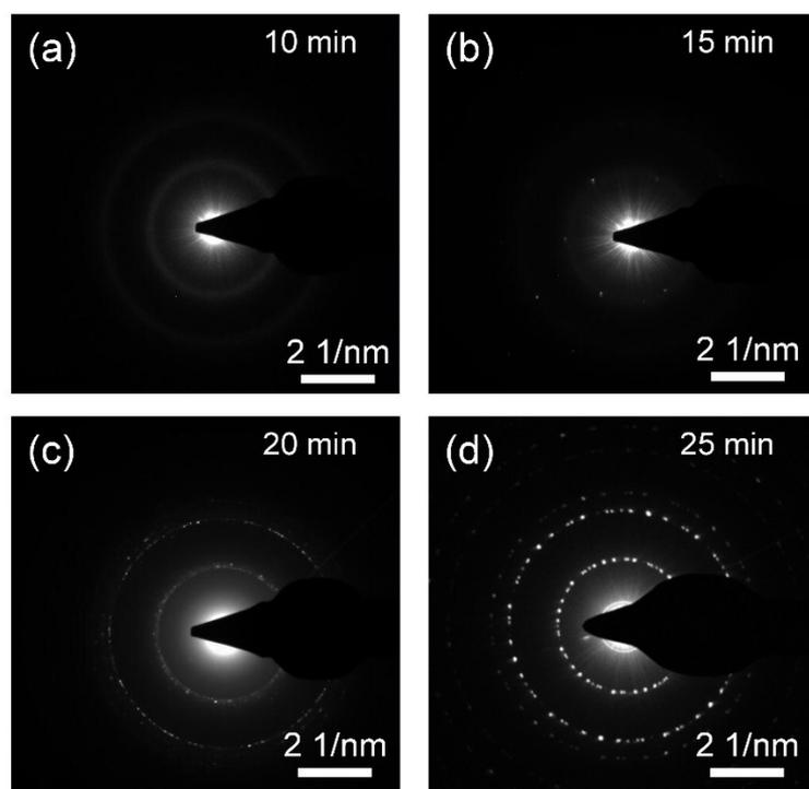
**Fig. S4** (a-d) SAED patterns of VGPNs directly grown on SiO<sub>2</sub> substrates for growth time of 10 min, 15 min, 20 min and 25 min, respectively, with  $I_{RF}$  of 400 W in 550 °C.
