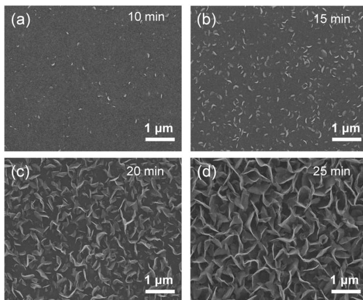
**Fig. S3** SEM images of VGPNs directly grown on SiO<sub>2</sub> substrates for growth time of 10 min, 15 min, 20 min and 25 min, respectively, with  $I_{RF}$  of 400 W at 550 °C.
