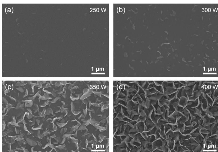
**Fig. S8** SEM images of VG NPs directly grown on SiO<sub>2</sub> substrates for plasma power of 250 W, 300 W, 350 W and 400 W, respectively, with growth time of 25 min at 550 °C.
