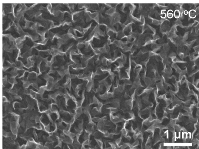
**Fig. S7** SEM image of VG NPs directly grown on SiO<sub>2</sub> substrate for growth temperature of 560 °C, with I<sub>RF</sub> of 400 W in 25 min.
