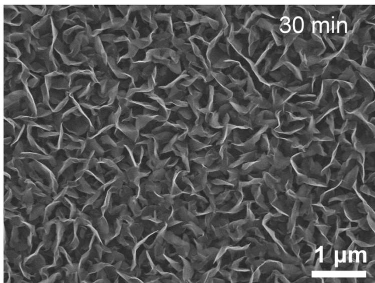
**Fig. S5** SEM images of VGPNs directly grown on SiO<sub>2</sub> substrate for growth time of 30 min, with I<sub>RF</sub> of 400 W at 550 °C.
