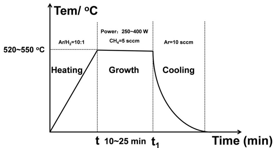
**Fig. S1** Experimental process schematic illustrates the preparation of VGNPs by PACVD
