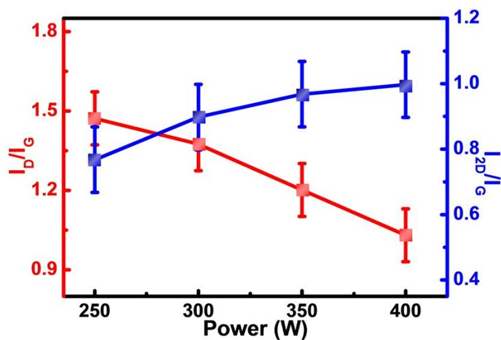
**Fig. S11** The intensity ratios  $I_D/I_G$  and  $I_{2D}/I_G$  of VG NPs directly grown on  $\text{SiO}_2$  substrates for plasma power of 250 W, 300 W, 350 W and 400 W, respectively, with growth time of 25 min at 550 °C.
