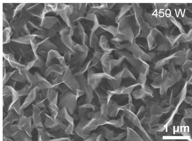
**Fig. S10** SEM image of VGPNs directly grown on SiO<sub>2</sub> substrate for plasma power of 450 W, with growth time of 25 min at 550 °C
