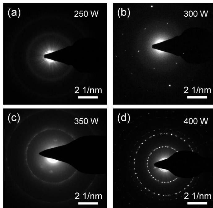
**Fig. S9** (a-d) SAED patterns of VGPNs directly grown on SiO<sub>2</sub> substrates for plasma power of 250 W, 300 W, 350 W and 400 W, respectively, with growth time of 25 min at 550 °C.
