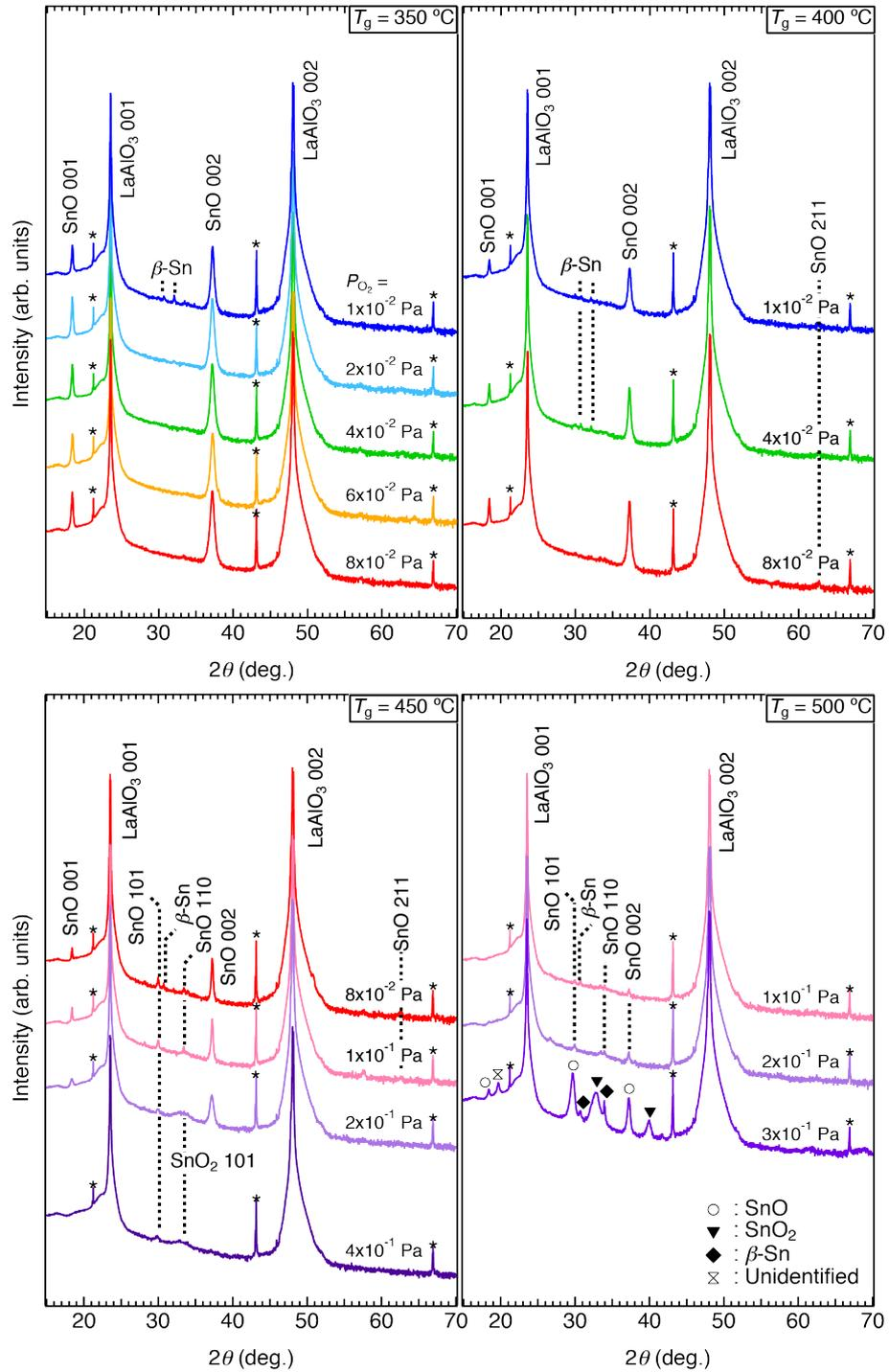
**Figure S1.** XRD patterns of the grown films on a LaAlO<sub>3</sub> (001) substrate at various  $T_g$  and  $P_{O_2}$ . The asterisks indicate the peaks originated by Cu K $\beta$  radiation.
