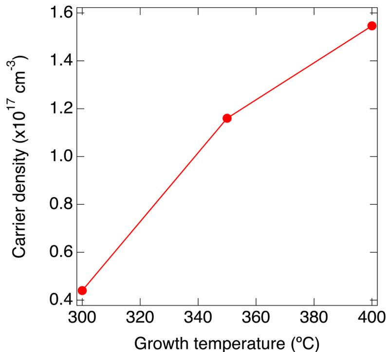
**Figure S5.** Carrier density of single-phase SnO films grown on YSZ substrate as a function of growth temperature.
