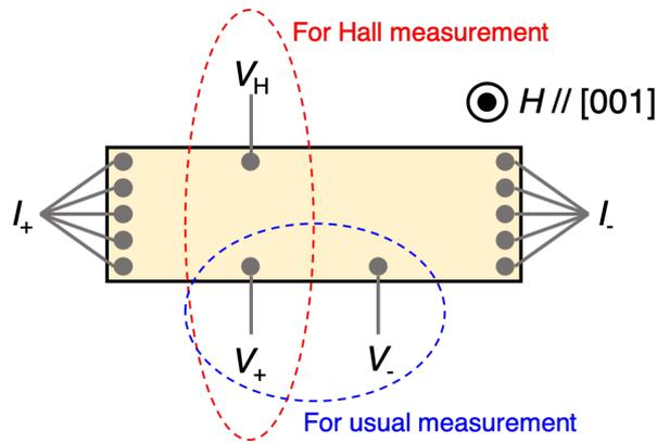
**Figure S3.** Schematic picture for the Hall measurements.
