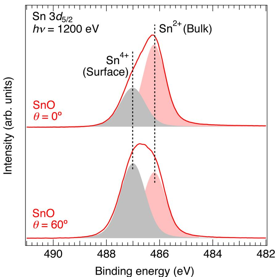
**Figure S2.** Angular (surface-sensitivity) dependent PES spectra from the SnO film for a Sn-3d<sub>5/2</sub> core level. The empirical spectrum can be fitted using two curves shaded with gray and red.
