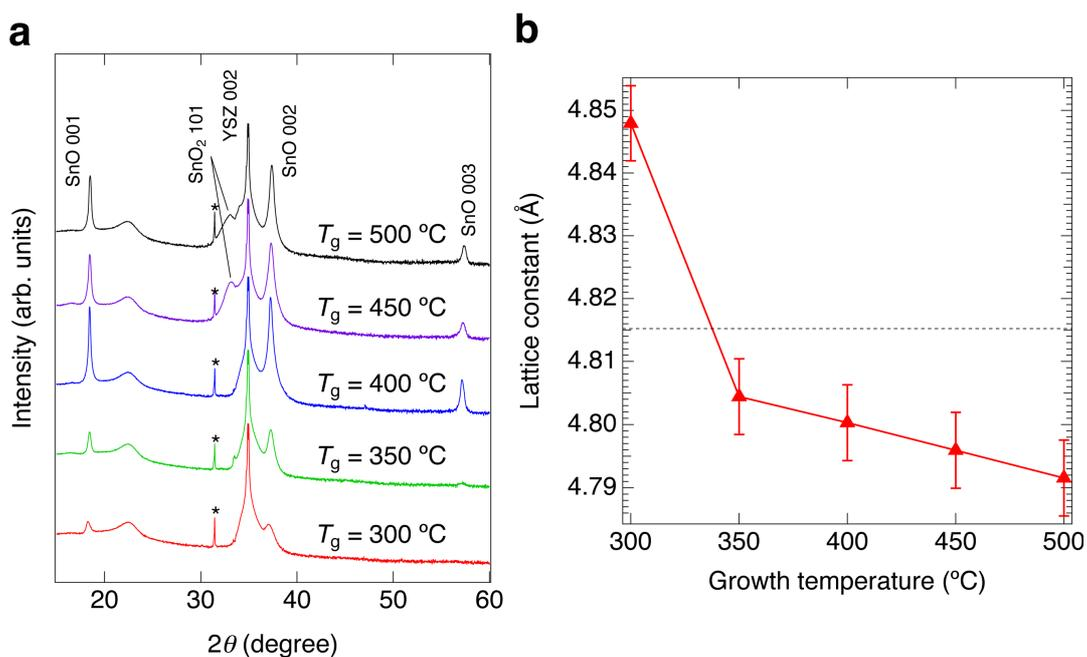
**Figure S4.** (a) XRD patterns of the grown films on a YSZ (001) substrate at various growth temperature  $T_g$ . The asterisks indicate the peaks originated by Cu  $K\beta$  radiation. (b) Estimated lattice constant from (00 $l$ ) Bragg peaks in Fig. S4a. Broken line corresponds to the reported lattice constant of bulk SnO.
