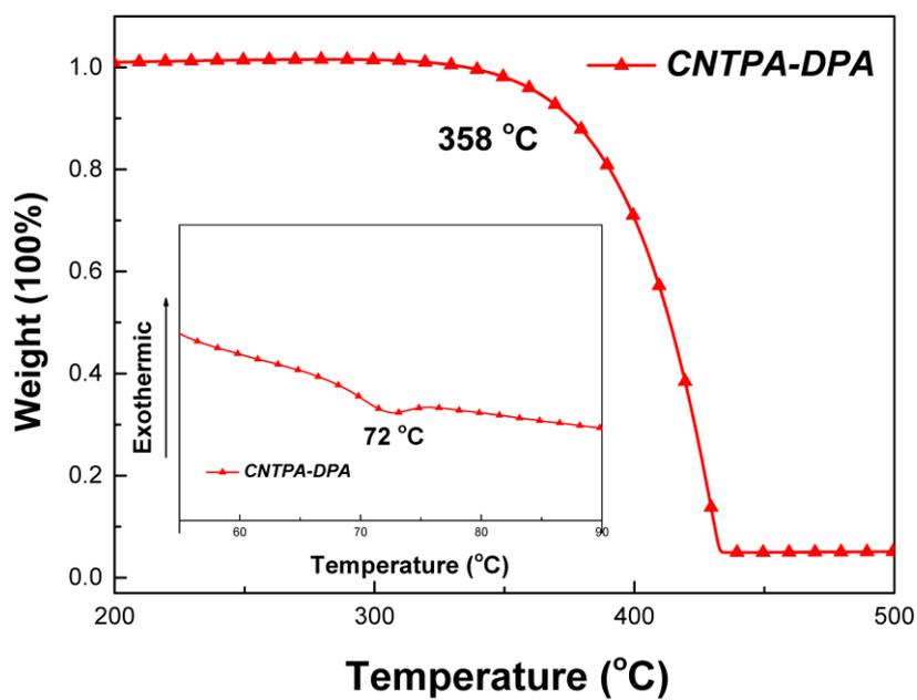
**Fig. S6** DSC traces and TGA curves of CNTPA-DPA recorded at a heating rate of  $10\text{ }^{\circ}\text{C min}^{-1}$ .
