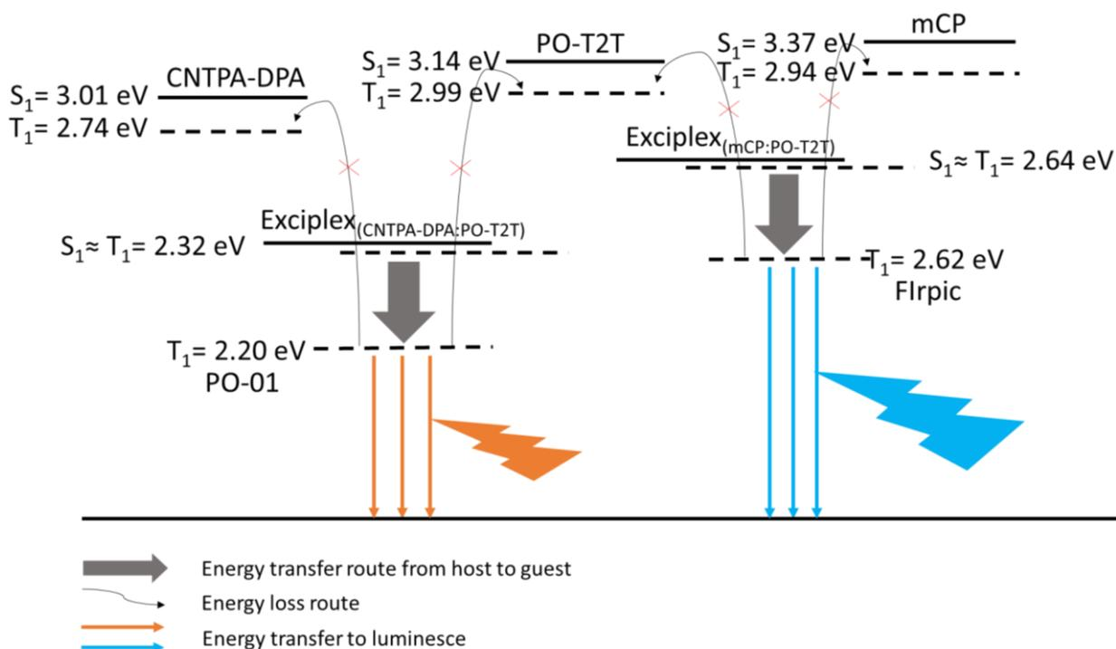
**Fig. S10** Schematic diagram of the exciton energy transfer or loss process of MEHs system.
