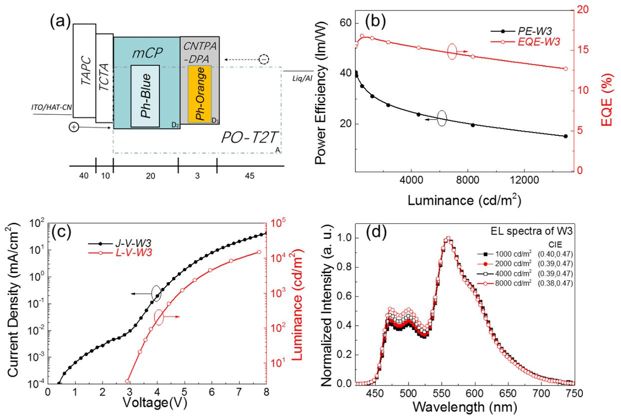
**Fig. S8** EL characteristics of Device W3. (a) Schematic diagram of W3 structure. (b) PE-Luminance-EQE (PE-L-EQE) curves of W3. (c) CE-Voltage-Luminance (CE-V-L) curves of W3. (d) Normalized EL spectra at various luminance of 1000, 2000, 4000 and 8000 cd m<sup>-2</sup> and the corresponding CIE values of W3.
