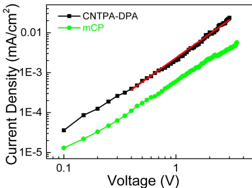
**Fig. S7** Current density versus voltage curves of hole-only devices for CNTPA-DPA and mCP. (ITO/HAT-CN (10 nm)/CNTPA-DPA or mCP (100 nm)/HAT-CN (10 nm)/Al (120 nm)).
