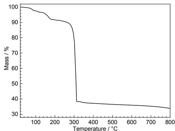
Thermogravimetric analysis of the as-prepared gadolinium trifluoroacetate performed under argon with a heating rate of  $10^{\circ}\text{C}\cdot\text{min}^{-1}$ .
