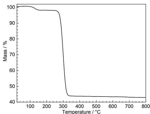
Thermogravimetric analysis of the as-prepared thulium trifluoroacetate performed under argon with a heating rate of 10°C.min<sup>-1</sup>.
