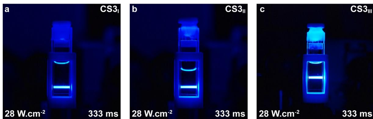
**Figure S6.** Photographs of the as-prepared CS3<sub>I</sub> (a), CS3<sub>II</sub> (b), and CS3<sub>III</sub> (c) upconverting nanocrystals under 980 nm excitation at 28 W.cm<sup>-2</sup>. All photographs were taken with a digital camera Nikon D80 equipped with a Micro-Nikkor objective (60mm f/2.8). All photographs were taken with the same ISO, shutter speed, and aperture photography settings: ISO 800, 1/3 s, f/5.6. A shortpass filter (500 nm) was inserted in front of the camera objective.
