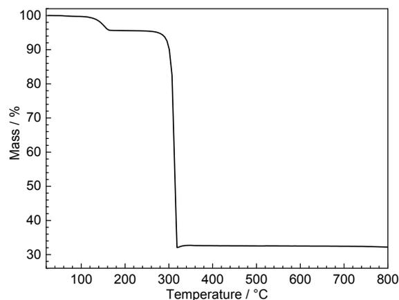
Thermogravimetric analysis of the as-prepared yttrium trifluoroacetate performed under argon with a heating rate of  $10^{\circ}\text{C}\cdot\text{min}^{-1}$ .
