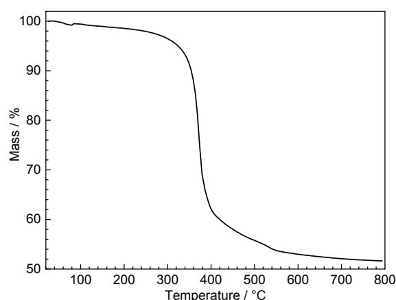
Thermogravimetric analysis of the as-prepared erbium acetate performed under argon with a heating rate of  $10^\circ\text{C}\cdot\text{min}^{-1}$ .
