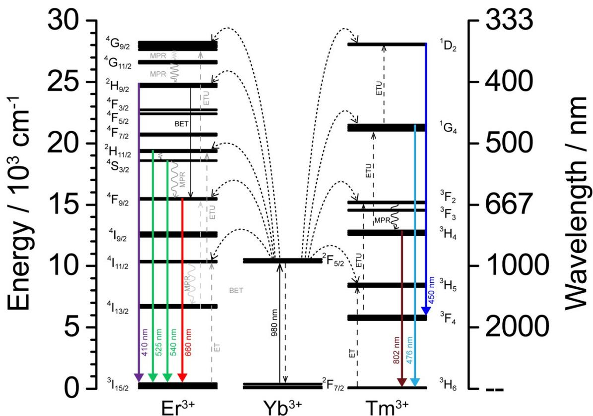
**Figure S3.** Partial electronic energy level diagram for trivalent erbium, ytterbium, and thulium ions. The main radiative transitions and their corresponding wavelengths are indicated as well as typical energy transfer mechanisms between the sensitizer and activators. ET = Energy Transfer, ETU = Energy Transfer Upconversion, MPR = Multi-Phonon Relaxation, BET = Back Energy Transfer.
