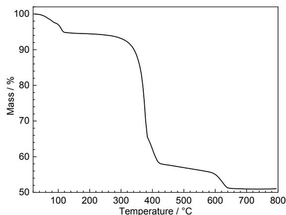
Thermogravimetric analysis of the as-prepared gadolinium acetate performed under argon with a heating rate of 10°C.min<sup>-1</sup>.
