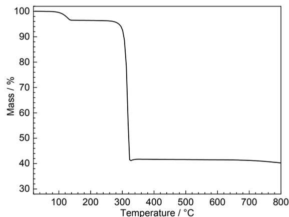
Thermogravimetric analysis of the as-prepared ytterbium trifluoroacetate performed under argon with a heating rate of  $10^{\circ}\text{C}\cdot\text{min}^{-1}$ .
