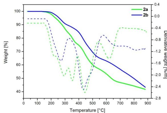
**Figure S1.** TGA and DTG curves of the phenothiazine derivatives **2a** and **2b**.
