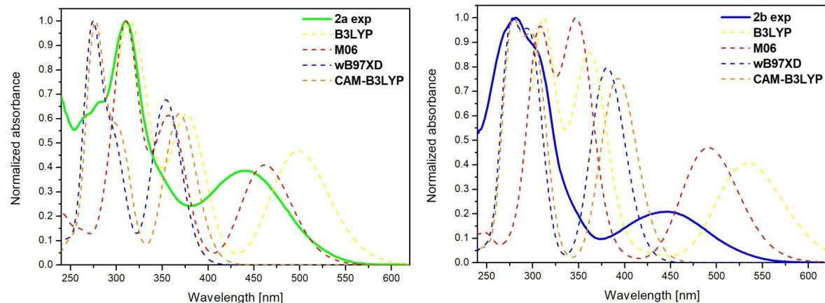
**Figure S3.** The absorption spectra of **2a** and **2b** in CHCl<sub>3</sub>: experimental and theoretical TD/DFT method (B3LYP, M06, CAM-B3LYP, wB97XD).
