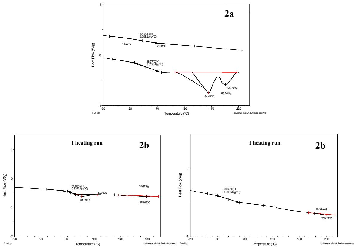
**Figure S2.** DSC curves of compound **2a** and **2b** registered during the first and second heating scans. Heating rate: 20 °C/min.
