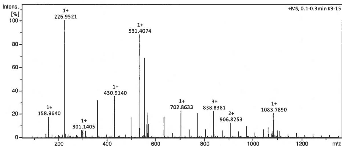
**Figure S11.** ESI-MS spectrum of a mixture of 10 mM ammonium bicarbonate in acetonitrile with water 90:10 (v / v) in positive ion mode.
