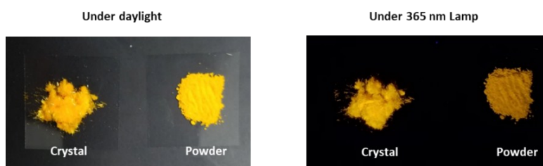
Fig. S6. Photoluminescence images of complex 1c before and after grinding under daylight and 365 nm lamp, respectively.
