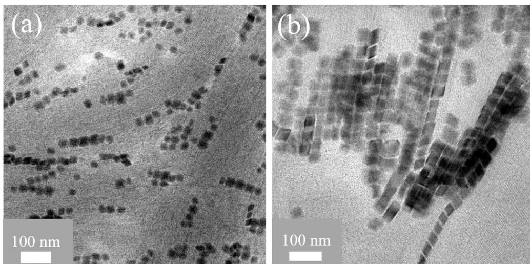
Fig. S1 TEM images of the self-assembled 1DSCs of (a) CsPbCl<sub>1.5</sub>Br<sub>1.5</sub> and (b) CsPbBr<sub>1.5</sub>I<sub>1.5</sub>.
