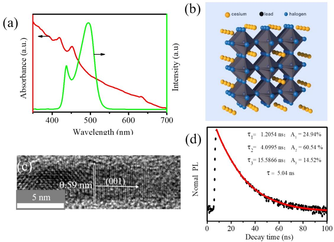
Figure S2 (a) UV-visible absorption (red line) and photoluminescence (green line) spectra of CsPbBr<sub>3</sub> NCs. The photoluminescence spectrum was collected at 365 nm excitation wavelength. (b) Crystal structure of cubic CsPbBr<sub>3</sub>. (c) High-resolution TEM image of CsPbBr<sub>3</sub> NWs. (d) Time-resolved PL decay curves of CsPbBr<sub>3</sub> NCs.
