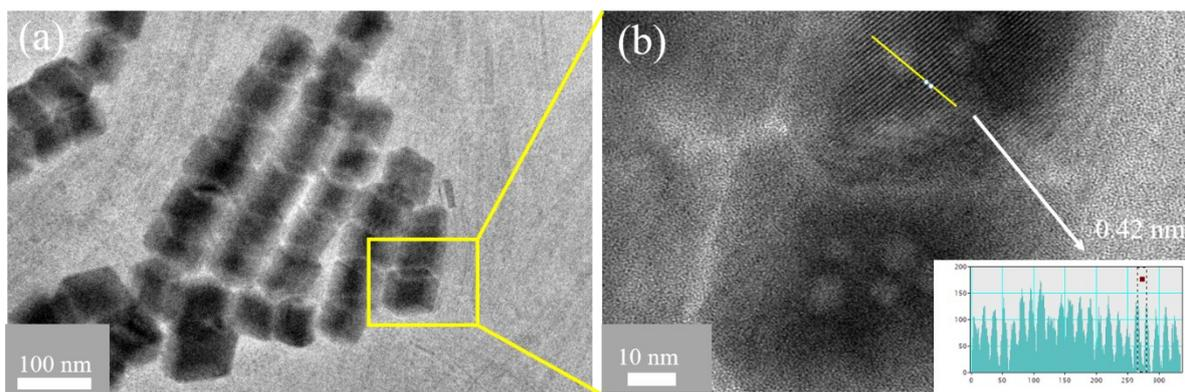
Figure S7 (a) TEM images of the c-CsPbBr<sub>3</sub> 1DSCs: (a) Low resolution. (b) High resolution.
