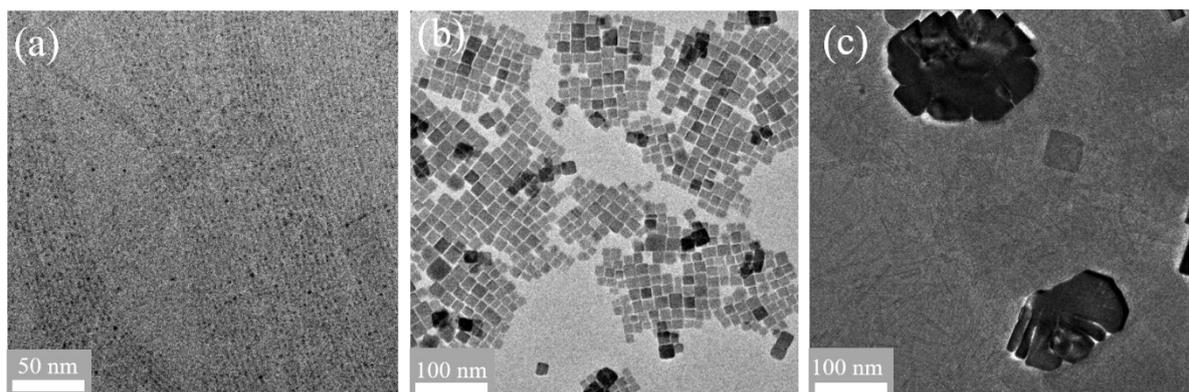
Figure S3 TEM images of CsPbBr<sub>3</sub> NCs: (a) NWs. (b) NSs. (c) Structure collapse of NWs and NSs.
