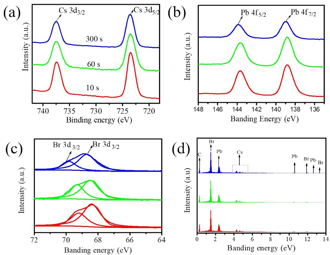
Figure S8. High-resolution XPS spectra of CsPbBr<sub>3</sub> NCs: (a) Cs 3d. (b) Pb 4f. (c) Br 3d. (d) EDS spectra of CsPbBr<sub>3</sub> NCs.
