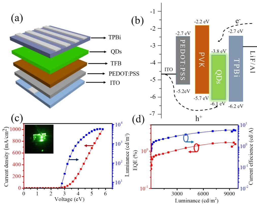
Figure S10 (a) LED device structure. (b) Flat band energy level diagram. (c) Current density (left) and luminance as a function of voltage (right). (d) Current efficiency (left) and external quantum efficiency (right) as a function of luminance.
