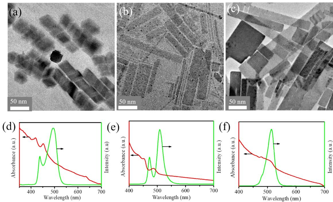
Figure S5 TEM images of CsPbBr<sub>3</sub> 1DSCs; (a) initial 1DSCs. (b) Ethanol-treated 1DSCs within 5 min. (c) Ethanol-treated 1DSCs within 1 hours. UV-visible absorption (red line) and photoluminescence (green line) spectra of CsPbBr<sub>3</sub> NCs: (d) initial 1DSCs. (e) Ethanol-treated 1DSCs within 5 min. (f) Ethanol-treated 1DSCs within 1 hours.
