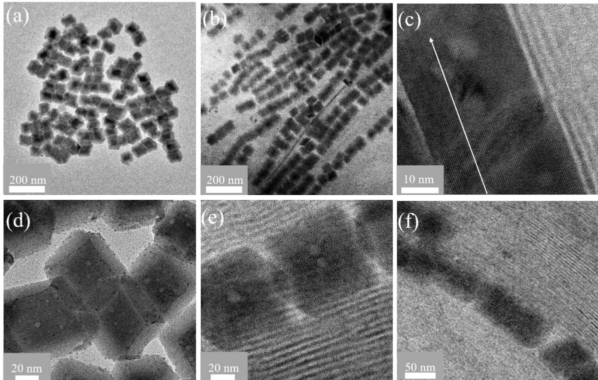
Figure S4 TEM images of randomly dispersed thick CsPbBr<sub>3</sub>NSs: (a) Low resolution. (d) High resolution. TEM images of 1DSCs with the same orientation as the NWs: (b, e) c-1DSCs. (c) s-1DSCs. (f) bent 1DSCs.
