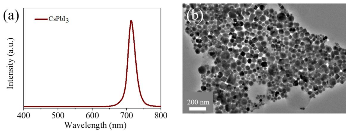
Figure S9 (a) Photoluminescence spectrum of CsPbI<sub>3</sub> NCs. (b)TEM image of CsPbBr<sub>3</sub> NSs.
