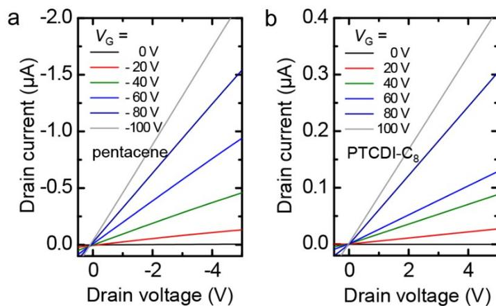
**Figure S3.** Linear plots of output curves of (a) pentacene and (b) PTCDI-C<sub>8</sub> OFETs with NbS<sub>2</sub>.
