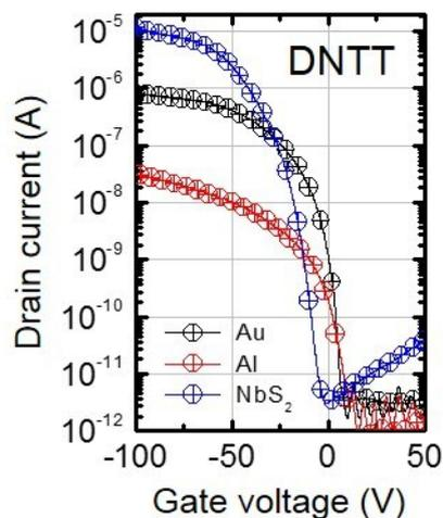
**Figure S4.** Comparison of transfer characteristics for DNTT FETs with Au, Al, and NbS<sub>2</sub> electrodes.
