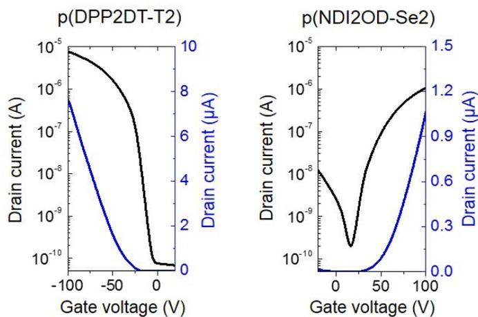
**Figure S5.** Transfer characteristics for p(DPP2DT-T2) FETs (left) and p(NDI2OD-Se2) FETs (right) with NbS<sub>2</sub> electrodes. The calculated carrier mobility was 0.087 Cm<sup>2</sup>/Vs for p(DPP2DT-T2) FETs and 0.013 Cm<sup>2</sup>/Vs for p(NDI2OD-Se2) FETs, respectively.
