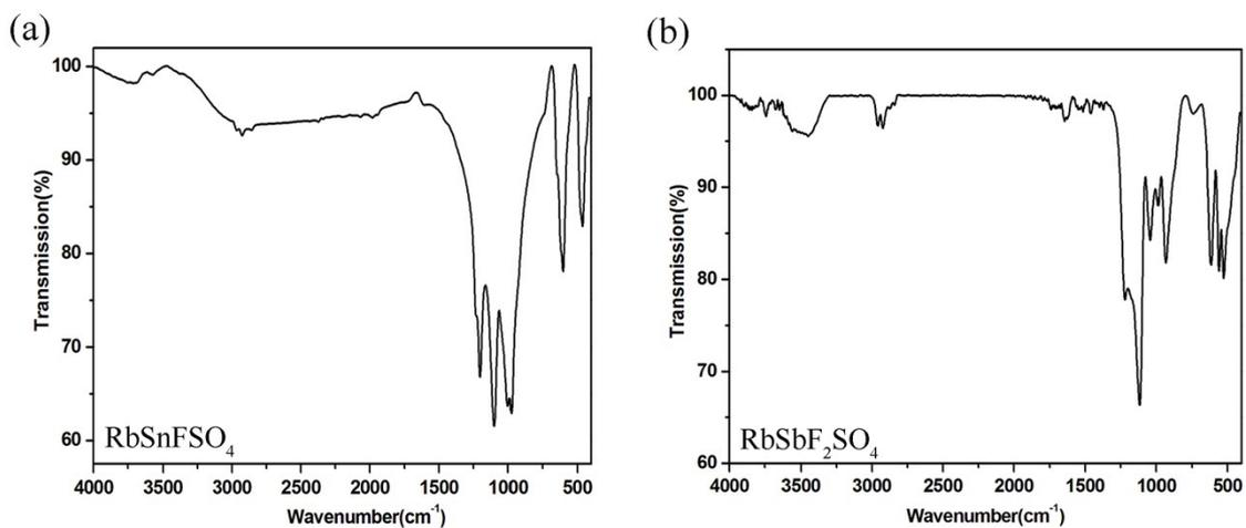
**Fig. S2.** IR spectra for  $\text{RbSnFSO}_4$  (a) and  $\text{RbSbF}_2\text{SO}_4$  (b).
