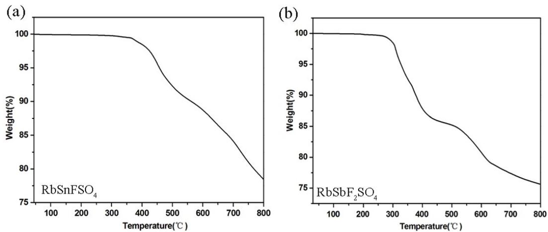
**Fig. S1.** TGA curves for  $\text{RbSnFSO}_4$  (a) and  $\text{RbSbF}_2\text{SO}_4$  (b).
