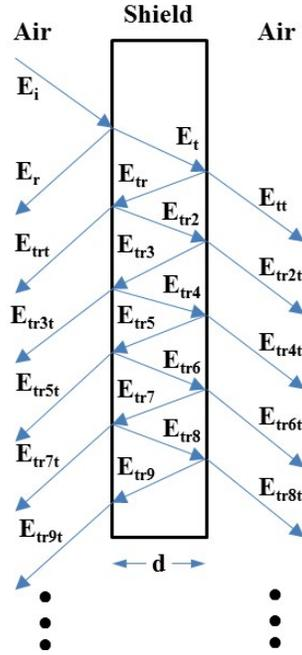
**Figure S1** Schematic illustration of reflection and transmission of electromagnetic wave.<sup>4</sup>
