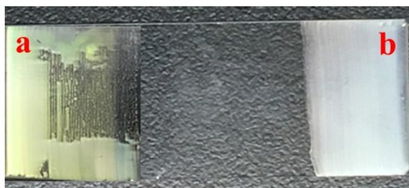
Fig.S6 Represented (a) PS microspheres and (b) PS-co-PNIPAM microspheres formed closed packed crystalline colloidal arrays on silica glass by vertical deposition technique, respectively
