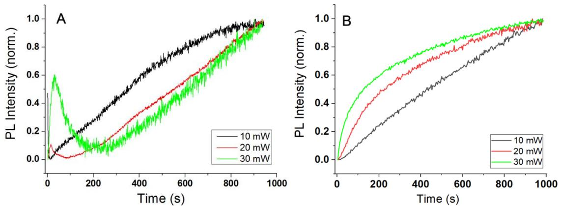
**Figure S5.** Change in PL intensity at 530 nm for MAPbBr<sub>3</sub> films under continuous 407 nm laser illumination in the air (a) and nitrogen environment (b).
