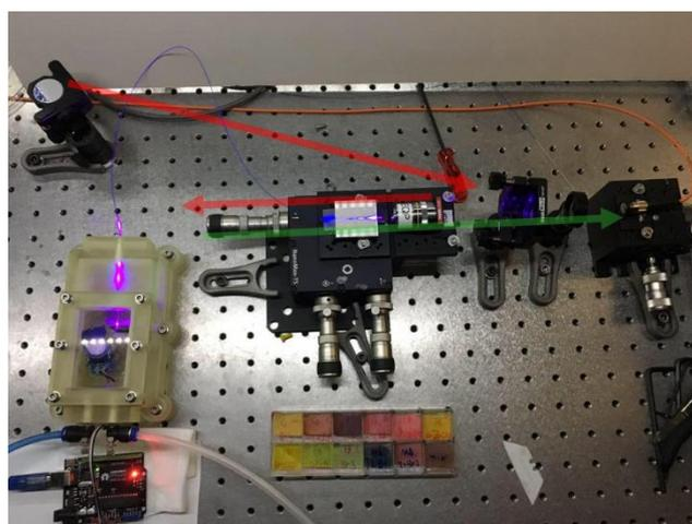
**Figure S14.** The home-built chamber for O<sub>2</sub> controlling experiment. The Oxygen level was controlled through adjusting the gas flow of pure nitrogen and dry air. Red arrow in the picture indicating the incoming 407 nm light for film excitation and green arrow shows the excited PL transmitted backwards to the spectrometer.
