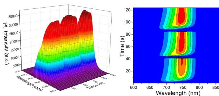
**Figure S7.** The reversible phase segregation of MAPbI<sub>2</sub>Br<sub>1</sub> film under 1 mW 407 nm laser illumination. Laser was blocked for 20 min between each cycle. Samples are measured under ambient condition (22 °C, 40 ± 5% RH).
