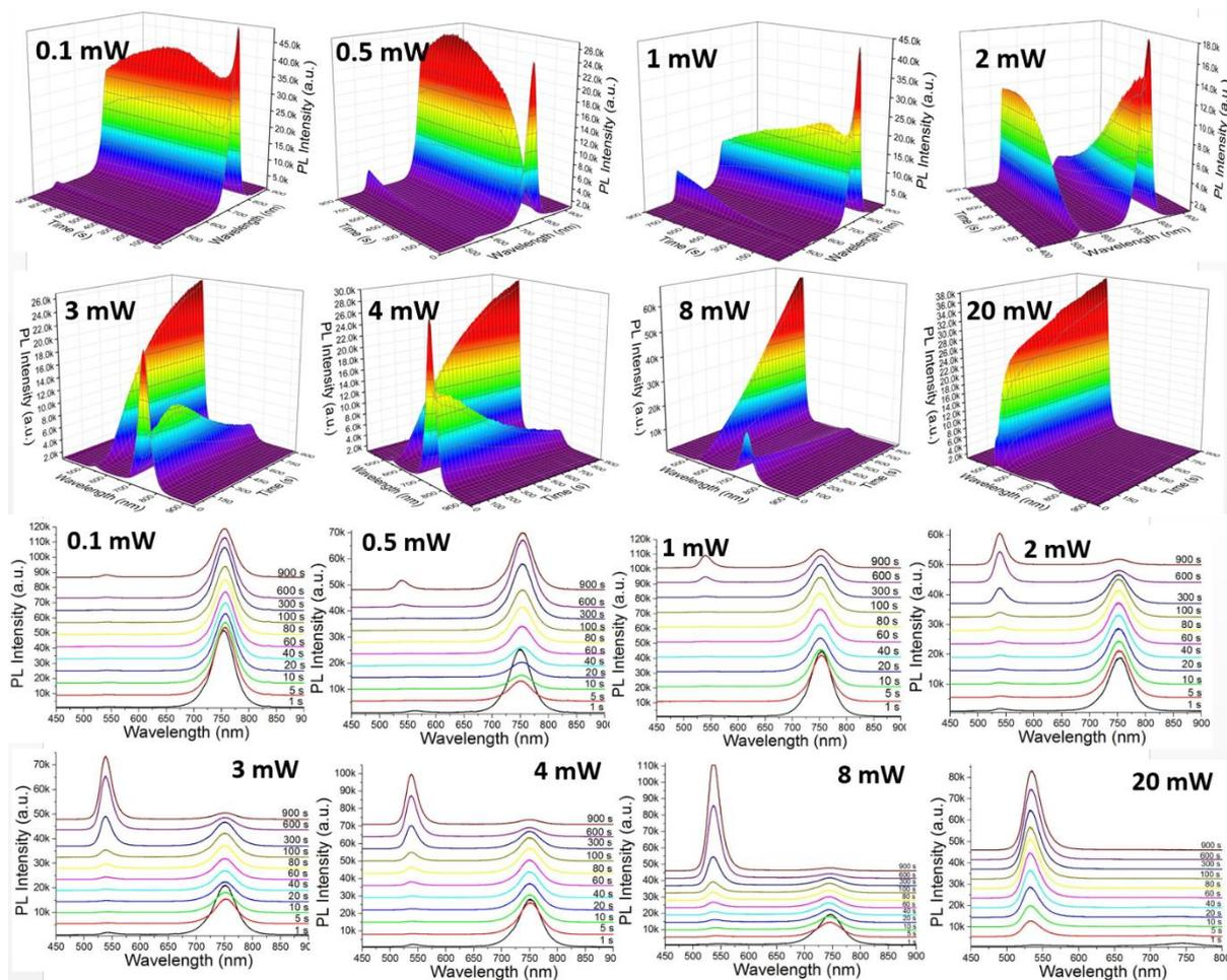
**Figure S13.** PL spectra of MAPbI<sub>0.5</sub>Br<sub>2.5</sub> film as a function of laser power (407 nm) during 900 s. Samples are measured under ambient condition (22 °C, 40 ± 5% RH).
