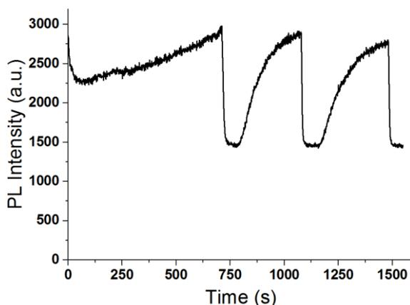
**Figure S17.** PL Spectral evolution of oxygen-dependent PL of degraded MAPbBr<sub>3</sub> film at 530 nm as a function of time in a 1 % oxygen and full nitrogen alternative environment. Film is under illumination by 20 mW 407 nm laser.
