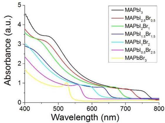
**Figure S3.** The absorbance spectra of the freshly prepared MAPbI<sub>3-x</sub>Br<sub>x</sub> films (x = 0.5, 1.0, 1.5, 2.0, 2.5).
