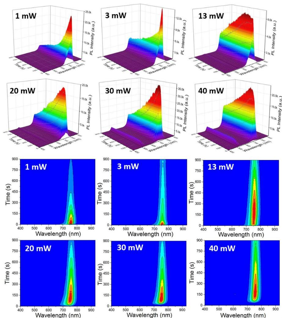
**Figure S11.** PL spectra of MAPbI<sub>2</sub>Br<sub>1</sub> film as a function of laser power (407 nm) during 900 s. Samples are measured under ambient condition (22 °C, 40 ± 5% RH).
