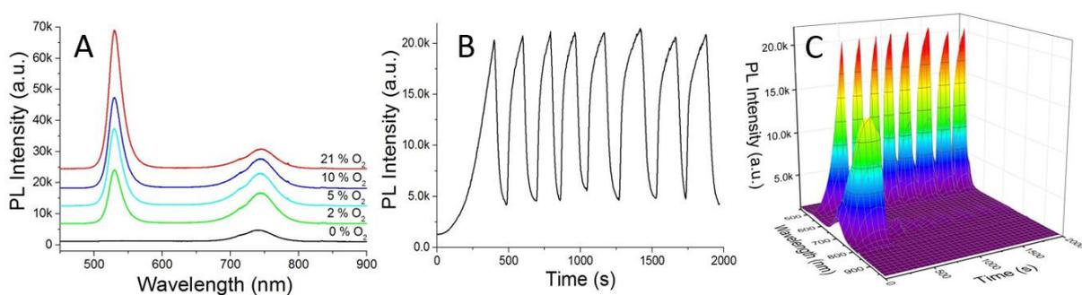
**Figure S16.** PL emission of MAPb<sub>1.5</sub>Br<sub>1.5</sub> film as a function of oxygen concentration after 900 s illumination by 20 mW 407 nm laser (a). Spectral evolution of oxygen-dependent PL of degraded MAPb<sub>1.5</sub>Br<sub>1.5</sub> film at 530 nm as a function of time in a 1 % oxygen and full nitrogen alternative environment (b), and (c) is the corresponding three-dimensional image indicating the peak position at 530 nm.
