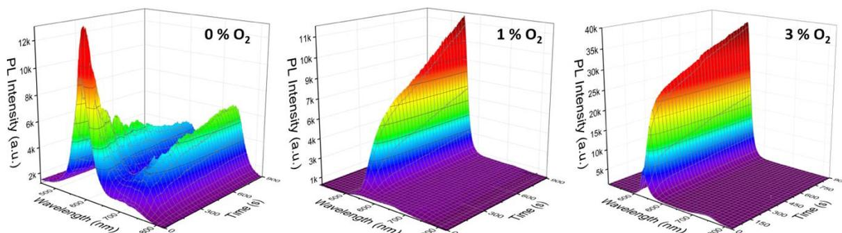
**Figure S15.** The evolving PL spectra during the 900 s continuous 20 mW laser illumination at different oxygen concentrations for MAPb<sub>0.5</sub>Br<sub>2.5</sub> films. Samples are measured under ambient condition (22 °C, 40 ± 5% RH).
