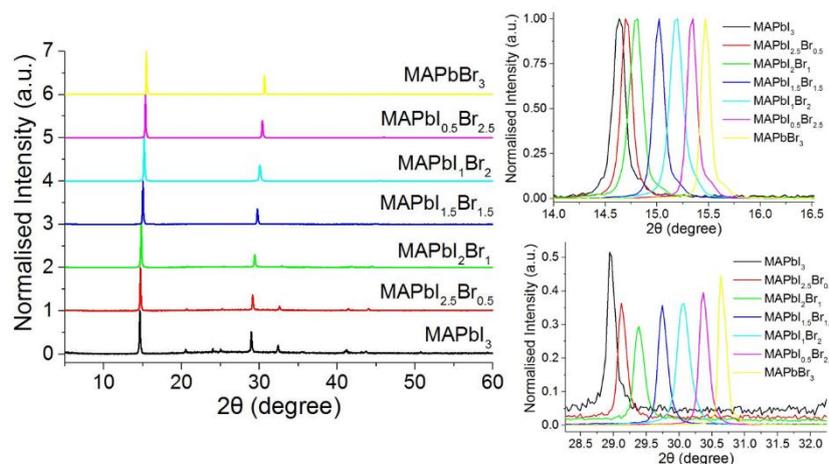
**Figure S2.** The XRD patterns of the freshly prepared MAPbI<sub>3-x</sub>Br<sub>x</sub> films (x = 0.5, 1.0, 1.5, 2.0, 2.5).
