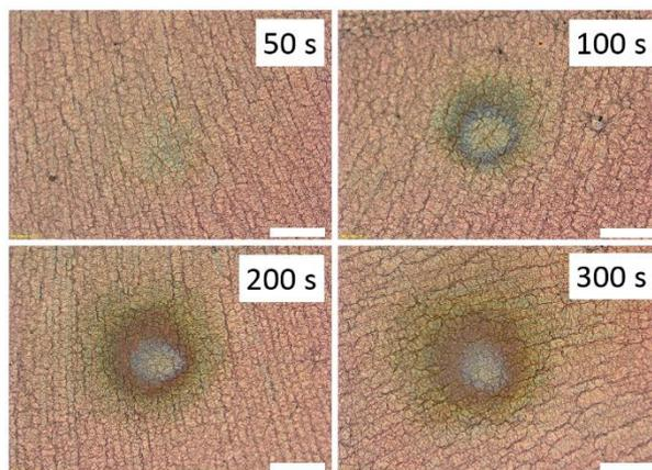
**Figure S9.** The reflection-mode microscopic images of the time-dependent morphology change of MAPbI<sub>1</sub>Br<sub>2</sub> film under 20 mW 407 nm laser. All the scale bars indicate 200 μm. We identified the core size of the damaged spot is ~150 μm. The appearance of the dark colour surrounding the core is possibly due to light scattering or local heating induced by strong laser.
