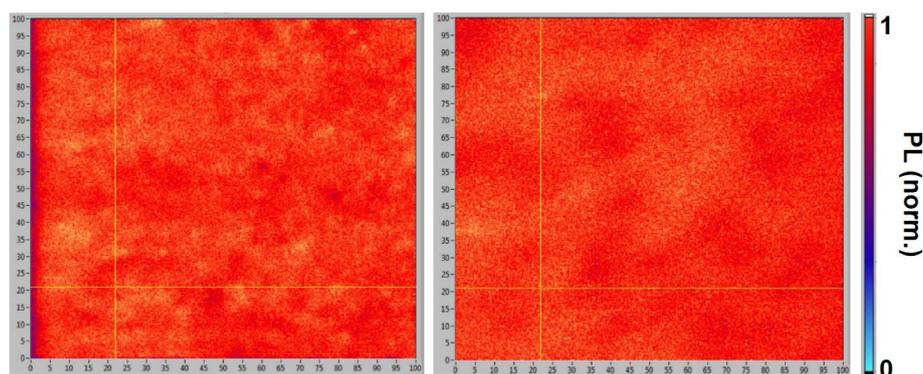
**Figure S1.** The PL mapping images of MAPbI<sub>1</sub>Br<sub>2</sub> and MAPbI<sub>2</sub>Br<sub>1</sub> films excited by 407 nm laser. The measured PL for MAPbI<sub>1</sub>Br<sub>2</sub> is 650 nm and for MAPbI<sub>2</sub>Br<sub>1</sub> is 690 nm,
