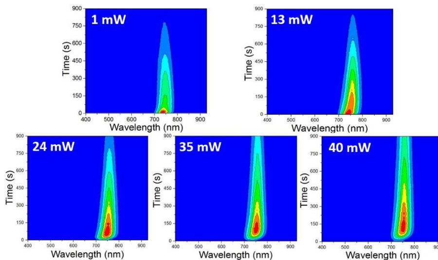
**Figure S10.** PL spectra of MAPbI<sub>2.5</sub>Br<sub>0.5</sub> film as a function of laser power (407 nm) over 900 s. Samples are measured under ambient condition (22 °C, 40 ± 5% RH).
