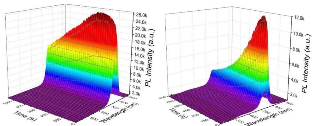
**Figure S18.** PL spectra of the encapsulated MAPbI<sub>1</sub>Br<sub>2</sub> (left) and MAPbI<sub>2</sub>Br<sub>1</sub> (right) film under 20 mW laser power (407 nm) illumination during 900 s. No peak was found at 530 nm.
