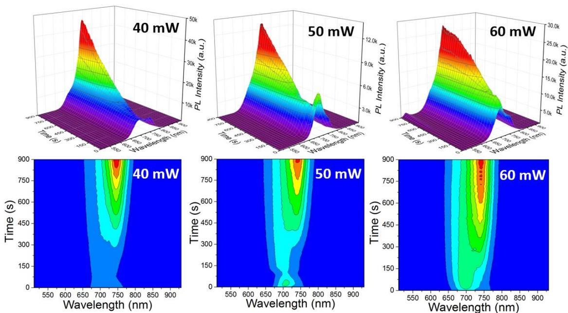
**Figure S19.** PL spectra of MAPbI<sub>1</sub>Br<sub>2</sub> perovskite film as a function of laser power (488 nm) during 900 s at ambient conditions.
