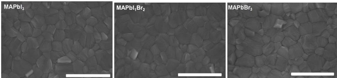
**Figure S4.** The SEM images of MAPbI<sub>3</sub> (left) MAPbI<sub>1</sub>Br<sub>2</sub> (middle) MAPbBr<sub>3</sub> (right). The scale bar indicates 1  $\mu$ m.
