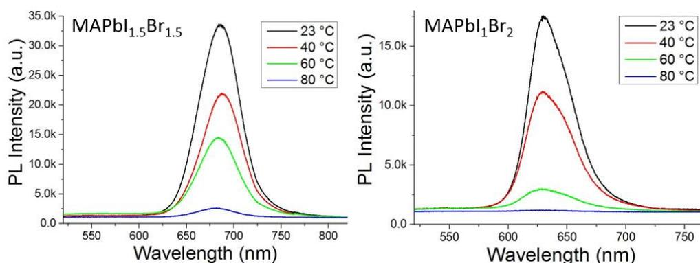
**Figure S6.** High temperature induced PL quenching for perovskite films in the open air. No peak was found at 530 nm.
