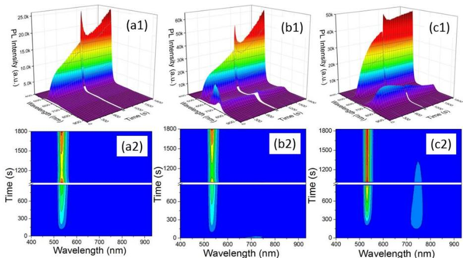
**Figure S8.** The irreversible phase degradation of MAPbI<sub>0.5</sub>Br<sub>2.5</sub> (a), MAPbI<sub>1</sub>Br<sub>2</sub> (b) and MAPbI<sub>1.5</sub>Br<sub>1.5</sub> (c) films under 40 mW 407 nm laser illumination. Laser was blocked for 20 min between each cycle. Samples are measured under ambient condition (22 °C, 40 ± 5% RH).
