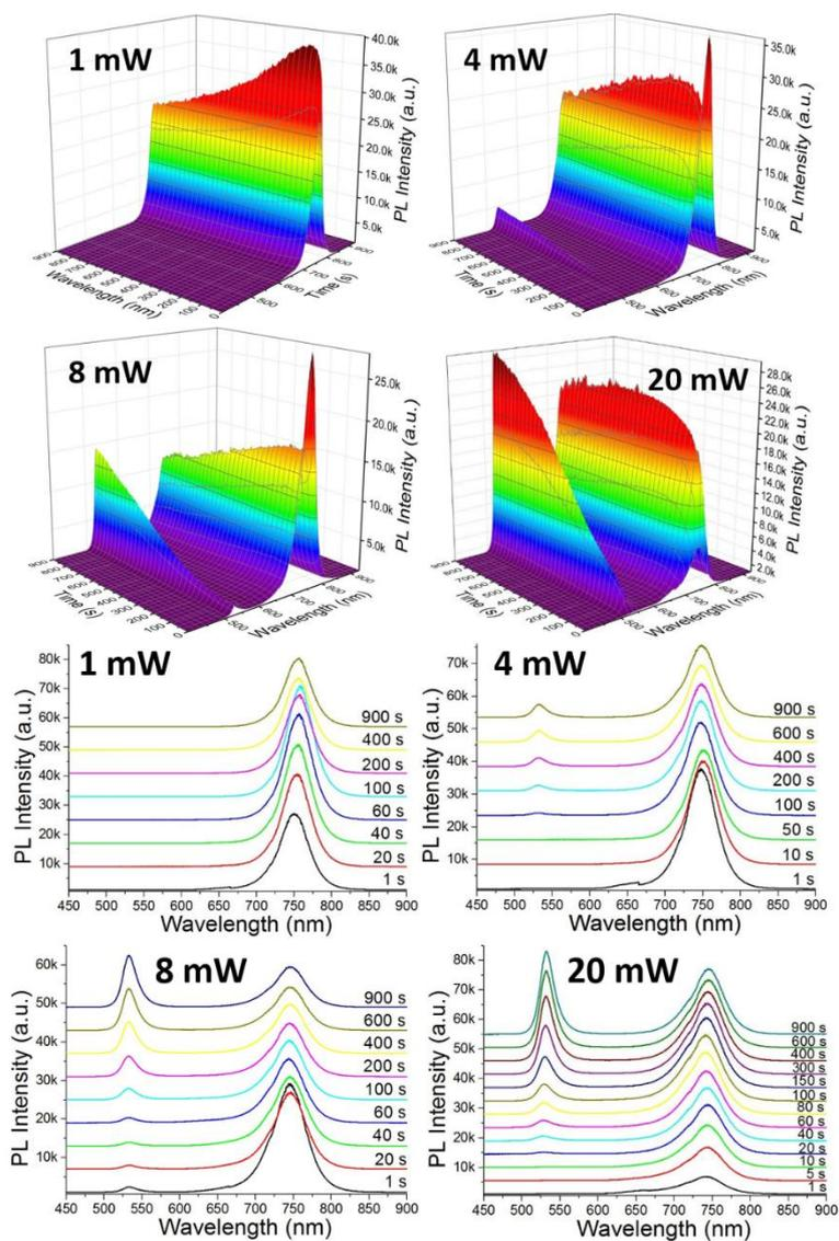
**Figure S12.** PL spectra of MAPbI<sub>1.5</sub>Br<sub>1.5</sub> film as a function of laser power (407 nm) over 900 s. Samples are measured under ambient condition (22 °C, 40 ± 5% RH).
