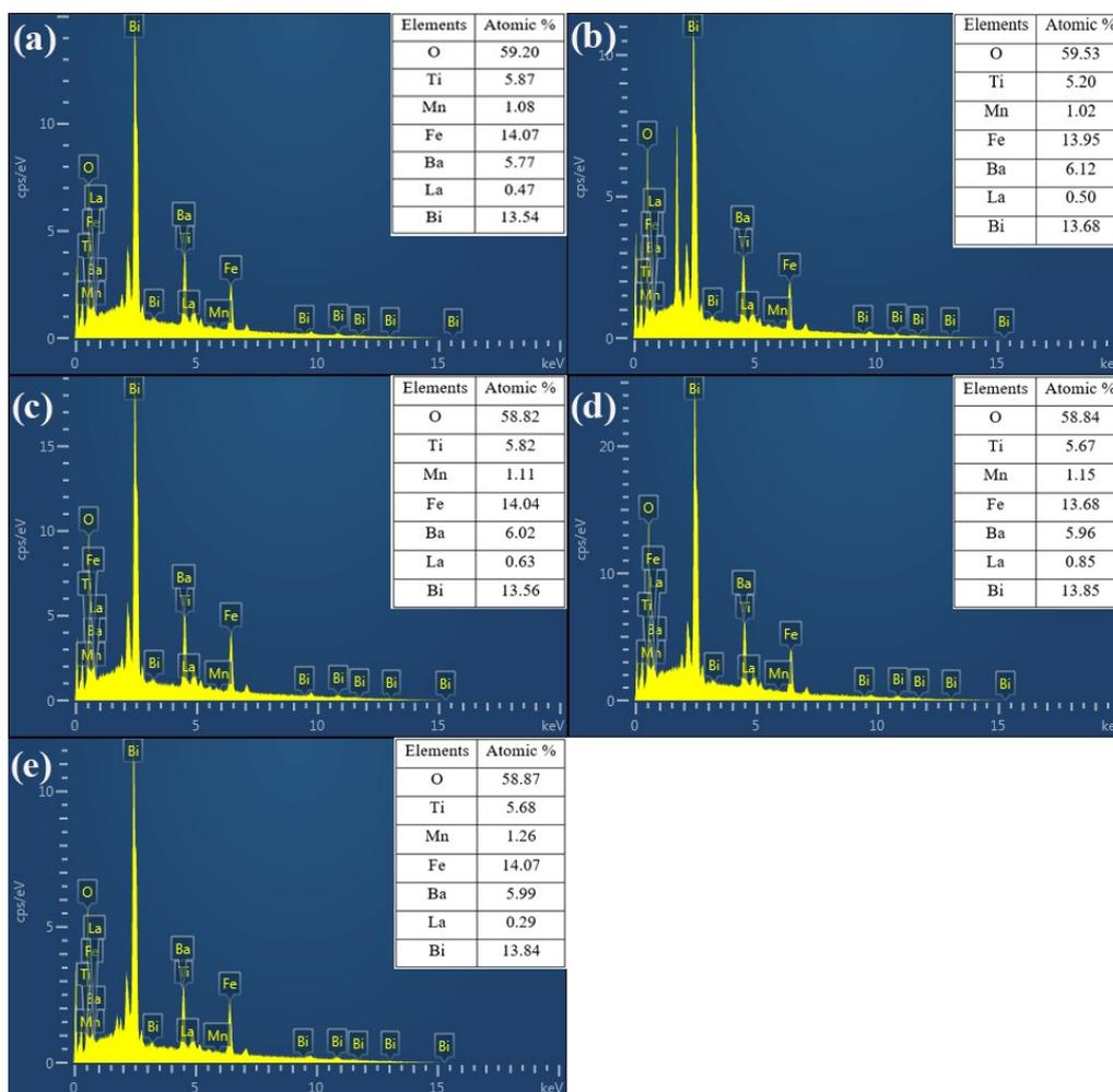
Fig. S8 EDS patterns of BFO–BTO–LFO–Mn–1 ceramics sintered at (a) T=975°C, (b) T=1000°C, (c) T=1025°C, (d) T=1050°C, (e) T=1075°C.
