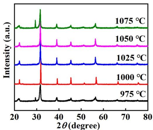
Fig. S5 XRD patterns of BFO-BTO-LFO-Mn-1 ceramics sintered at different temperature.
