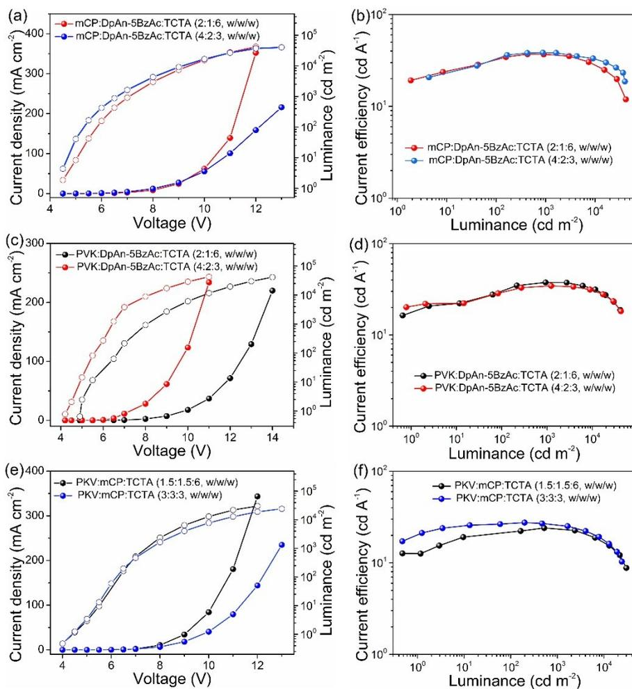
Figure S6. The current density-luminance-voltage (left) and current efficiency versus luminance (right) characteristics for Devices C-1 (a and b), C-2 (c and d) and C-3 (e and f) with different host doping ratios.
