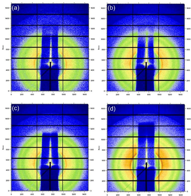
Figure S7. Two-dimensional (2D) GISAXS patterns of (a) mCP:DpAn-5BzAc:Ir(ppy)<sub>2</sub>acac; (b) PVK:DpAn-5BzAc:Ir(ppy)<sub>2</sub>acac; (c) PVK:mCP:Ir(ppy)<sub>2</sub>acac and (d) mCP:DpAn-5BzAc:TCTA:Ir(ppy)<sub>2</sub>acac.
