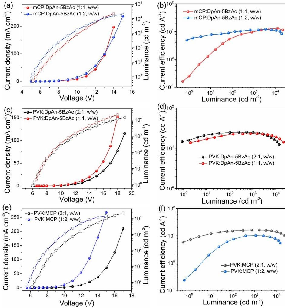
Figure S3. The current density-luminance-voltage (left) and current efficiency versus luminance (right) characteristics for Devices B-1 (a and b), B-2 (c and d) and B-3 (e and f) with different host doping ratios.
