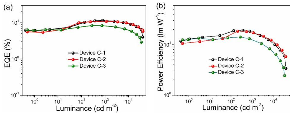
Figure S5. The EQE-L (left) and PE-L (right) characteristics for ternary blend hosts based devices.
