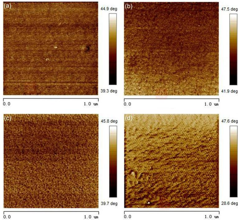
Figure S4. AFM phase images ( $1 \mu\text{m} \times 1\mu\text{m}$ ) of the (a) mCP:DpAn-5BzAc:Ir(ppy)<sub>2</sub>acac; (b) PVK:DpAn-5BzAc:Ir(ppy)<sub>2</sub>acac; (c) PVK:mCP:Ir(ppy)<sub>2</sub>acac and (d) mCP:DpAn-5BzAc:TCTA:Ir(ppy)<sub>2</sub>acac films deposited on glass substrate.
