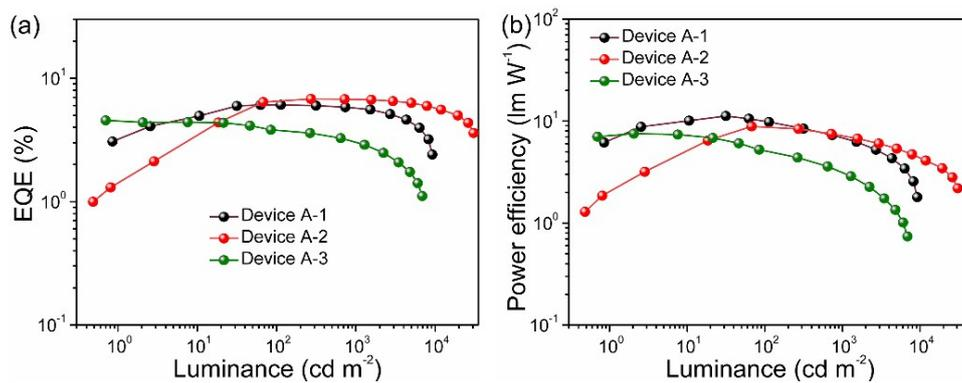
Figure S1. The EQE-L (left) and PE-L (right) characteristics for single host based devices.
