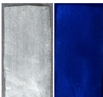
Fig. S2 Photographs of PVA film under visible light (left) and 365 nm UV light illumination (right).
