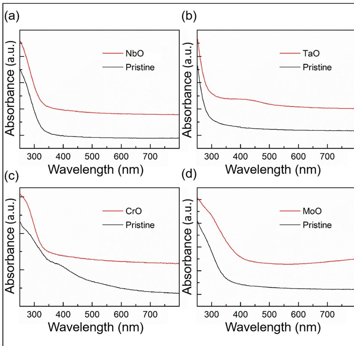
**Fig. S19** UV-vis absorption spectra of (a) NbO, (b) TaO, (c) CrO, (d) MoO before and after H<sub>2</sub> annealing treatment.
