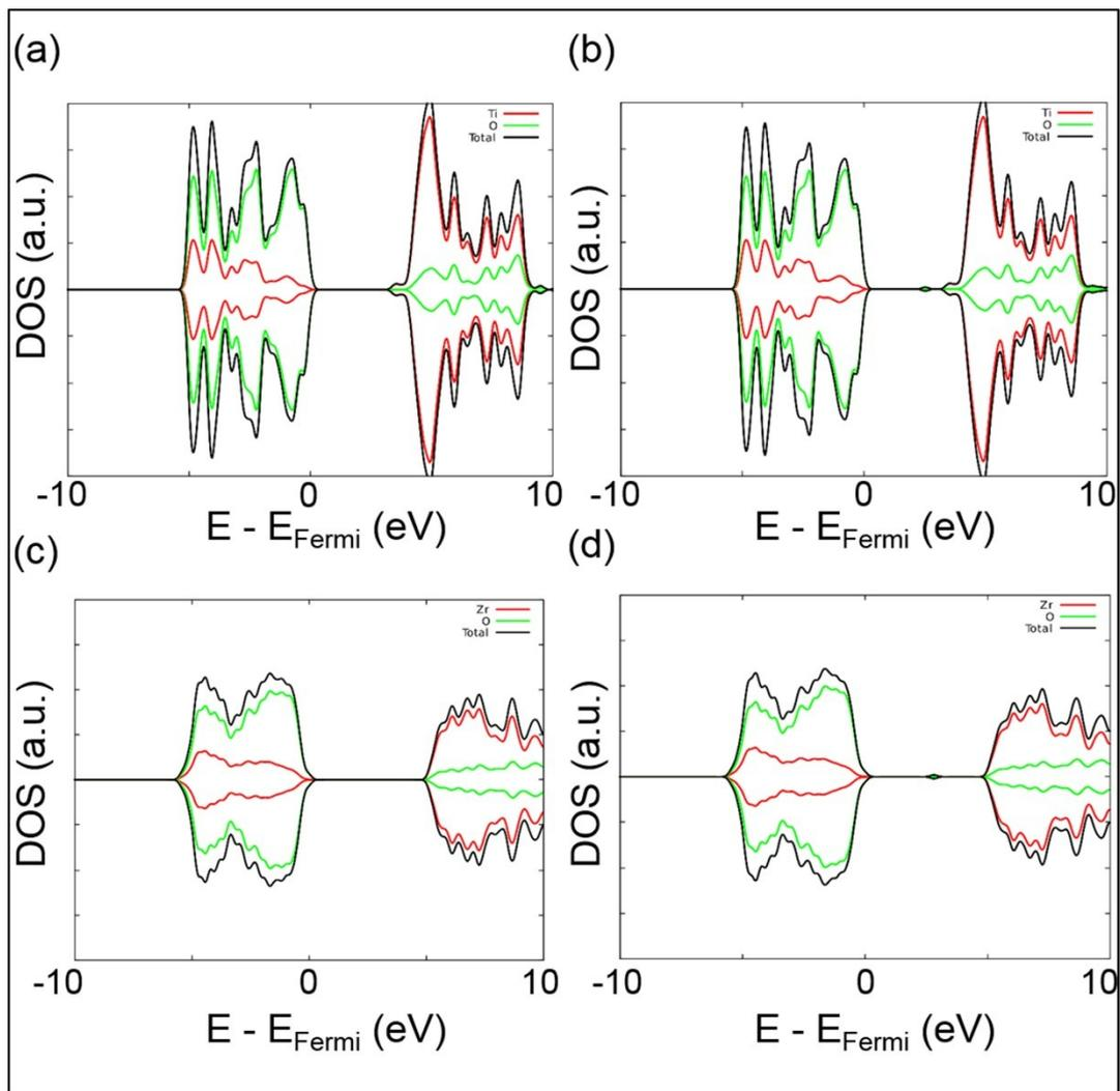
**Fig. S26** The PDOS of (a and b) TiO and (c and d) ZrO before and after annealing, respectively.
