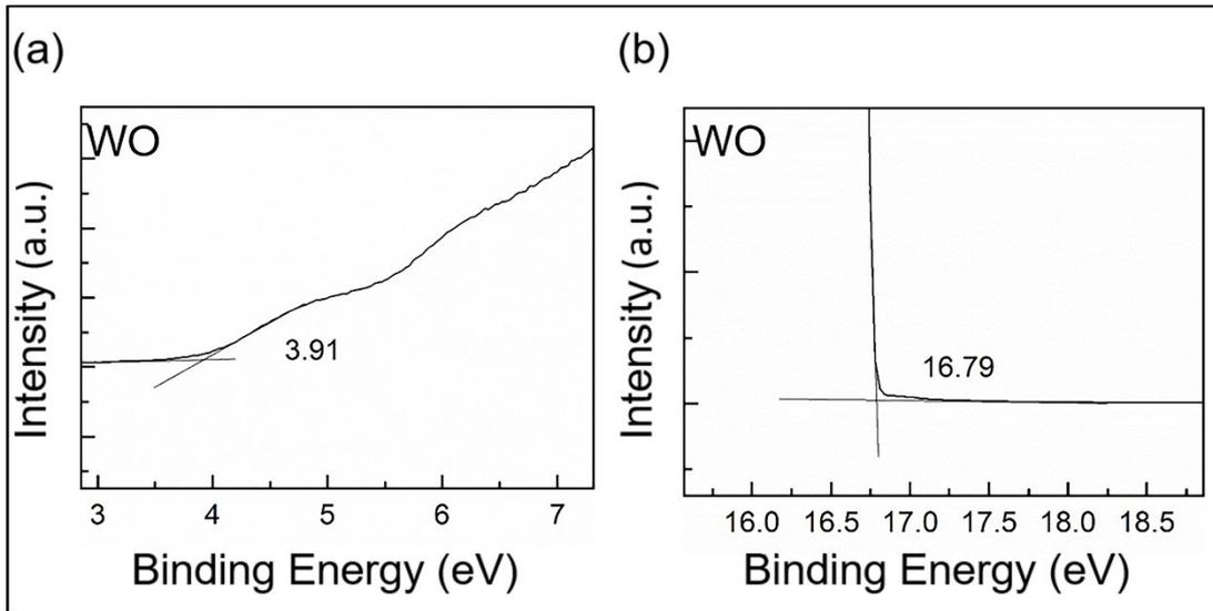
**Fig. S5** The UPS spectra of (a and b) WO after annealing. The work function of WO is 4.43 eV ( $21.22 - 16.79$ ). The VB level of WO is situated at 8.34 eV ( $4.43 + 3.91$ ).
