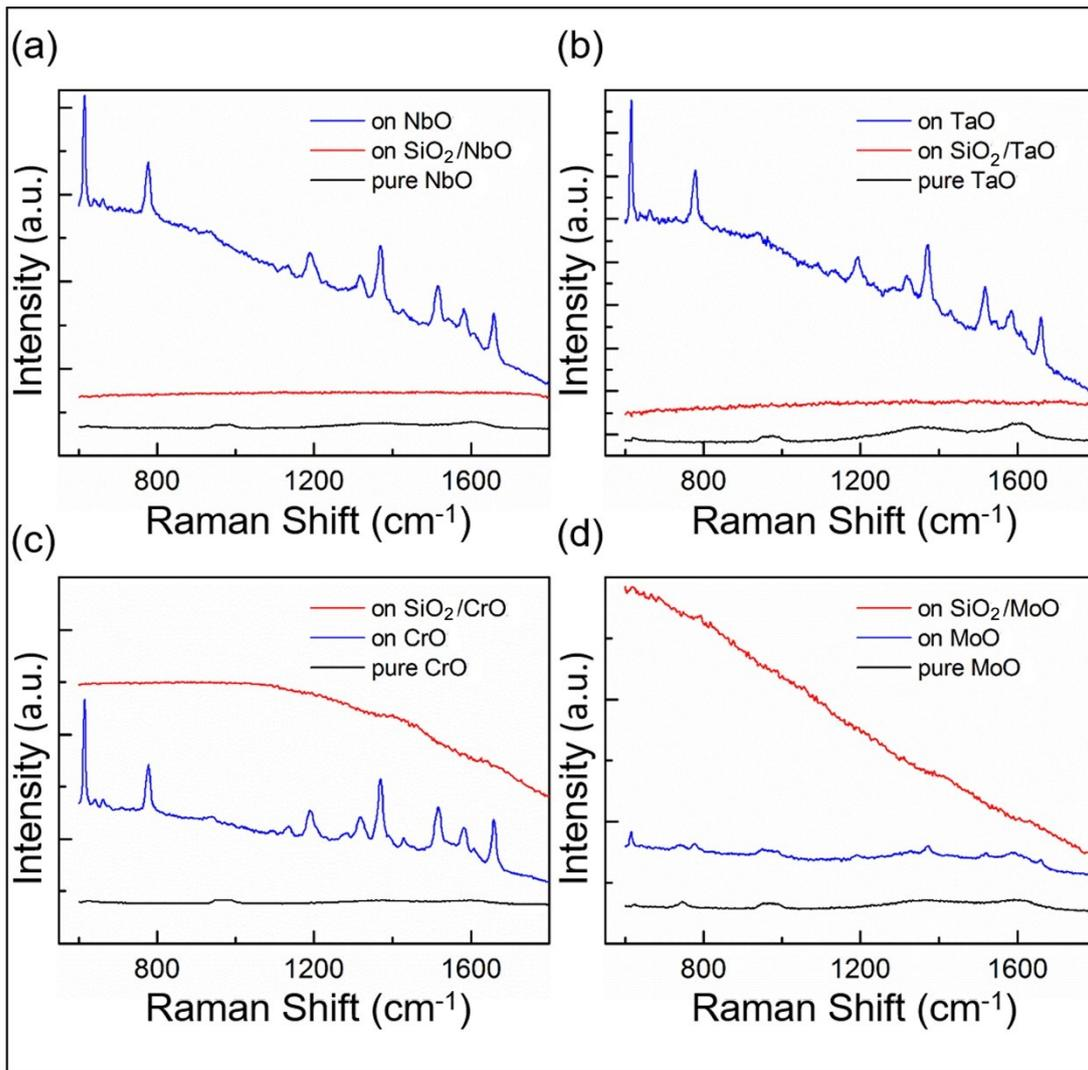
**Fig. S21** The Raman spectra of R6g at a concentration of  $10^{-5}$  M absorbed on (a) NbO, (b) TaO, (c) CrO, (d) MoO and a SiO<sub>2</sub> dielectric layer coated on them after H<sub>2</sub> annealing treatment.
