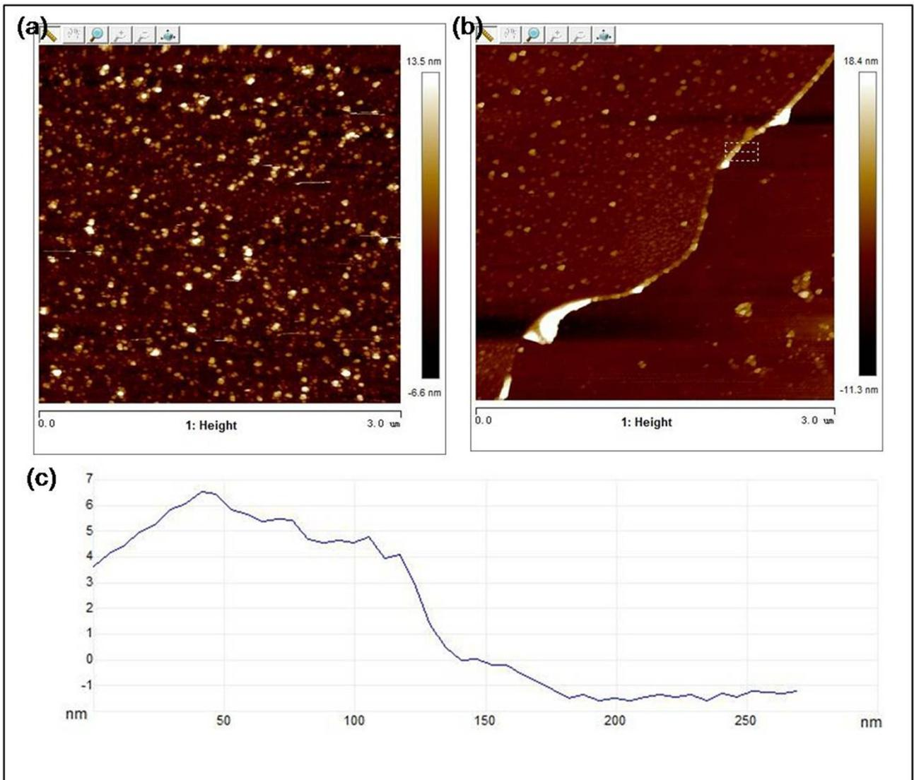
**Fig. S11** The roughness (a) and thickness (b) of HfO<sub>2</sub>. The Ra value of roughness is 1.840 nm. (c) The value of thickness is below 9 nm.
