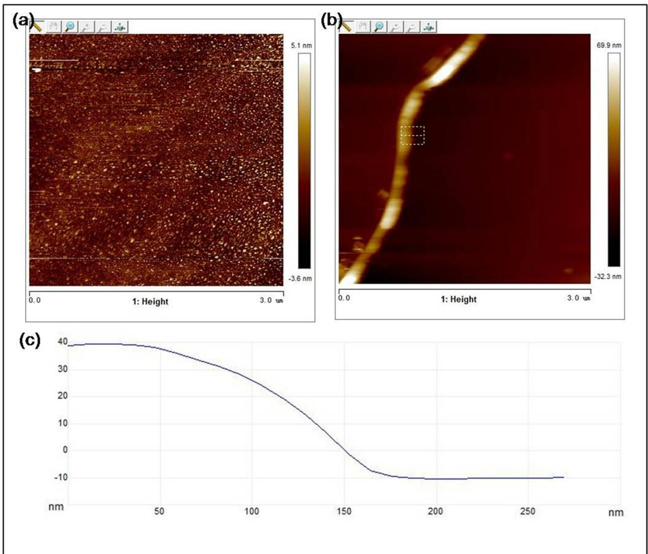
**Fig. S14** The roughness (a) and thickness (b) of TaO. The Ra value of roughness is 0.786 nm. (c) The value of thickness is below 50 nm.
