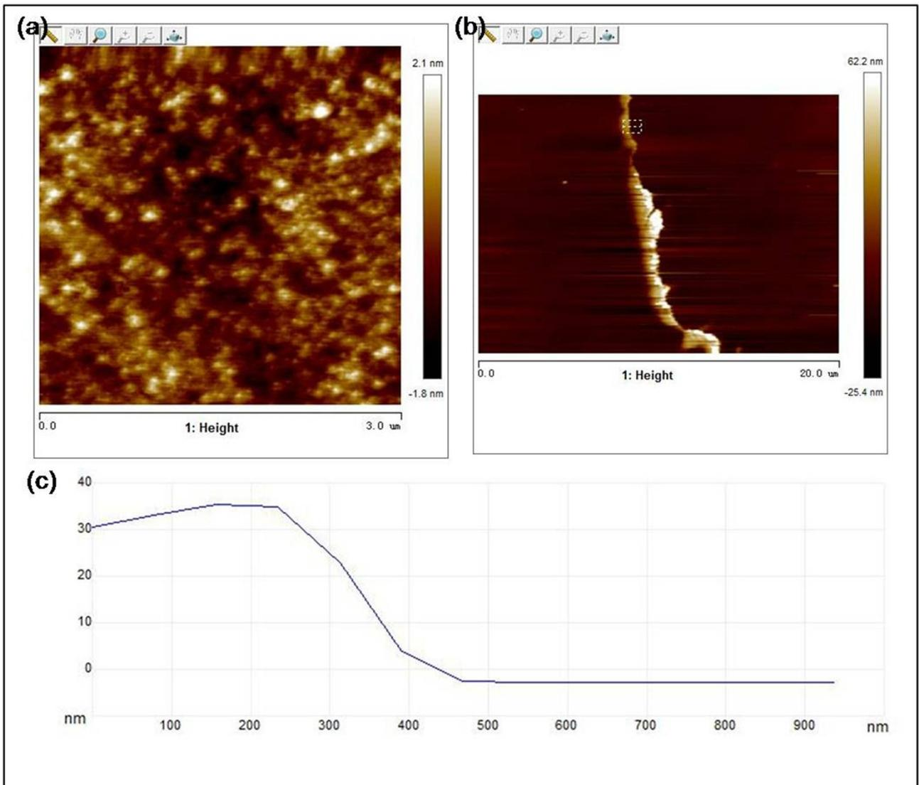
**Fig. S10** The roughness (a) and thickness (b) of ZrO. The Ra value of roughness is 0.360 nm. (c) The value of thickness is below 40 nm.
