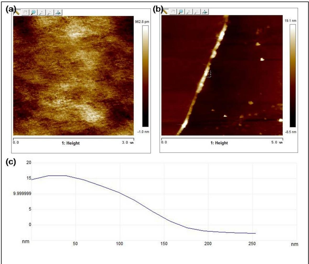
**Fig. S13** The roughness (a) and thickness (b) of NbO. The Ra value of roughness is 0.134 nm. (c) The value of thickness is below 20 nm.
