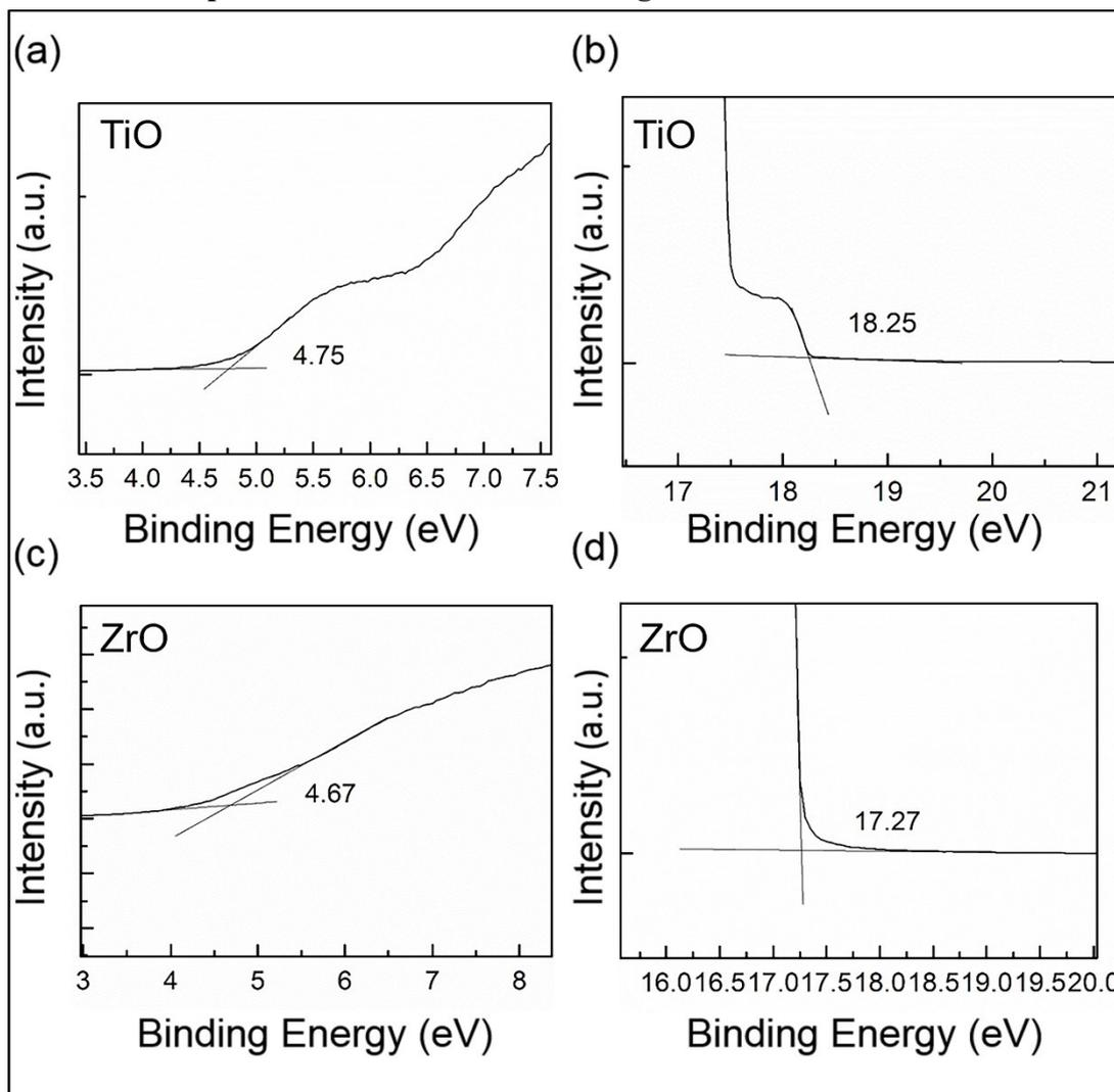
**Fig. S1** The UPS spectra of (a and b) TiO and (c and d) ZrO after annealing. The work function of TiO is 2.97 eV ( $21.22 - 18.25$ ). The VB level of TiO is situated at 7.72 eV ( $2.97 + 4.75$ ).<sup>1</sup> The work function of ZrO is 3.95 eV ( $21.22 - 17.27$ ). The VB level of ZrO is situated at 8.62 eV ( $3.95 + 4.67$ ).
