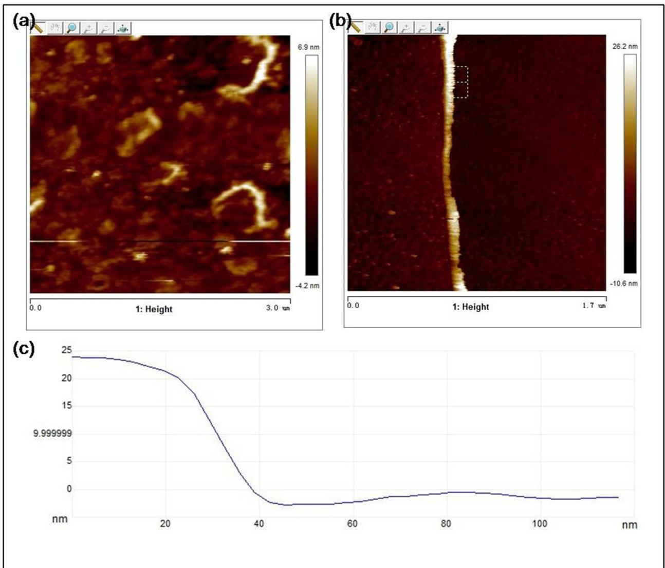
**Fig. S17** The roughness (a) and thickness (b) of WO. The Ra value of roughness is 0.826 nm. (c) The value of thickness is below 30 nm.
