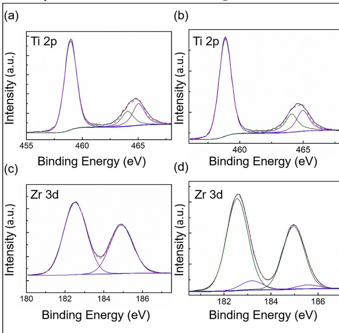
**Fig. S22** XPS spectra of (a and b) Ti 2p core levels for TiO and (c and d) Zr 3d core levels for ZrO before and after annealing, respectively.
