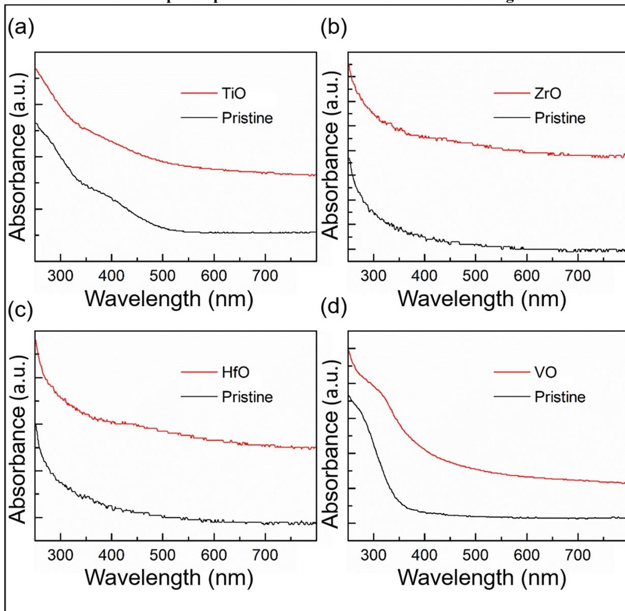
Fig. S18 UV-vis absorption spectra of (a) TiO, (b) ZrO, (c) HfO, (d) VO before and after H<sub>2</sub> annealing treatment.
