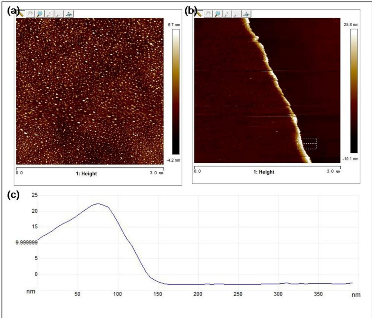
**Fig. S9** The roughness (a) and thickness (b) of TiO. The Ra value of roughness is 1.130 nm. (c) The value of thickness is below 25 nm.
