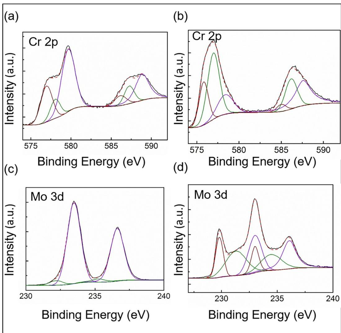
**Fig. S25** XPS spectra of (a and b) Cr 2p core levels for CrO and (c and d) Mo 3d core levels for MoO before and after annealing, respectively.
