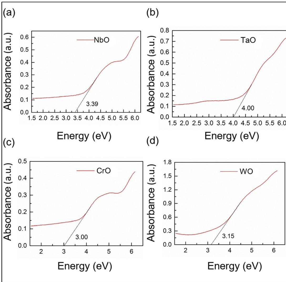
**Fig. S7**  $(\alpha\hbar\omega)^{1/2}$  as a function of photon energy ( $\hbar\omega$ ) for (a) NbO, (b) TaO, (c) CrO and (d) WO.  $E_g$  are 3.39 eV (NbO), 4.00 eV (TaO), 3.00 eV (CrO) and 3.15 eV (WO), respectively. The CB level of NbO is situated at 4.81 eV (8.20 – 3.39). The CB level of TaO is situated at 6.58 eV (10.58 – 4.00). The CB level of CrO is situated at 5.56 eV (8.56 – 3.00). The CB level of WO is situated at 5.19 eV (8.34 – 3.15).
