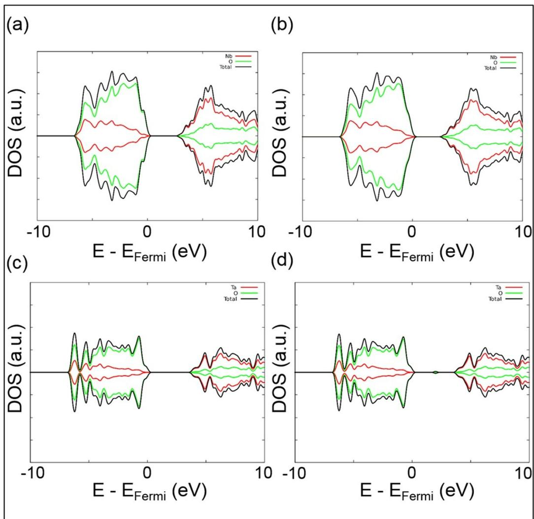
**Fig. S28** The PDOS of (a and b) NbO and (c and d) TaO before and after annealing, respectively.
