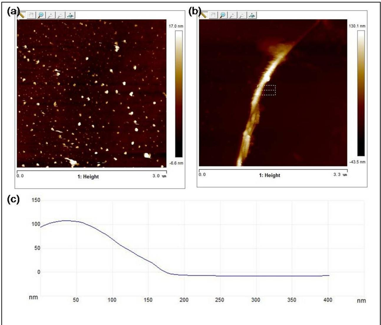
**Fig. S15** The roughness (a) and thickness (b) of CrO. The Ra value of roughness is 1.250 nm. (c) The value of thickness is below 110 nm.
