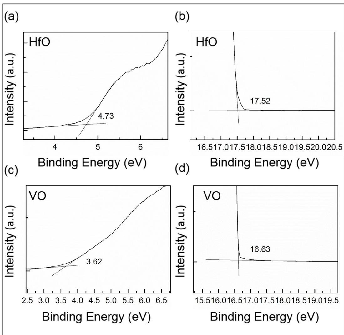
**Fig. S2** The UPS spectra of (a and b) HfO and (c and d) VO after annealing. The work function of HfO is 3.70 eV (21.22 – 17.52). The VB level of HfO is situated at 8.43 eV (3.70 + 4.73). The work function of VO is 4.59 eV (21.22 – 16.63). The VB level of VO is situated at 8.21 eV (4.59 + 3.62).
