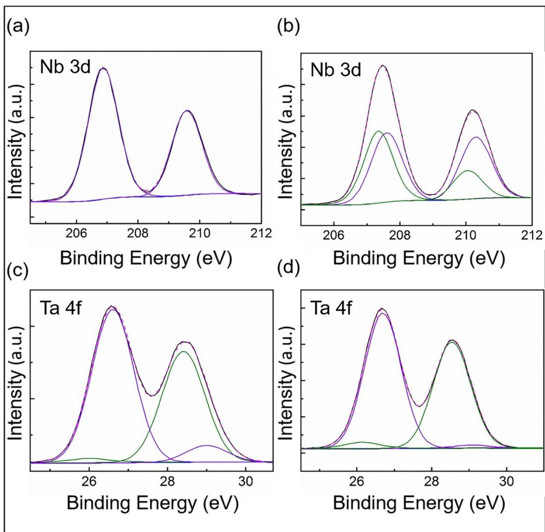
**Fig. S24** XPS spectra of (a and b) Nb 3d core levels for NbO and (c and d) Ta 4f core levels for TaO before and after annealing, respectively.
