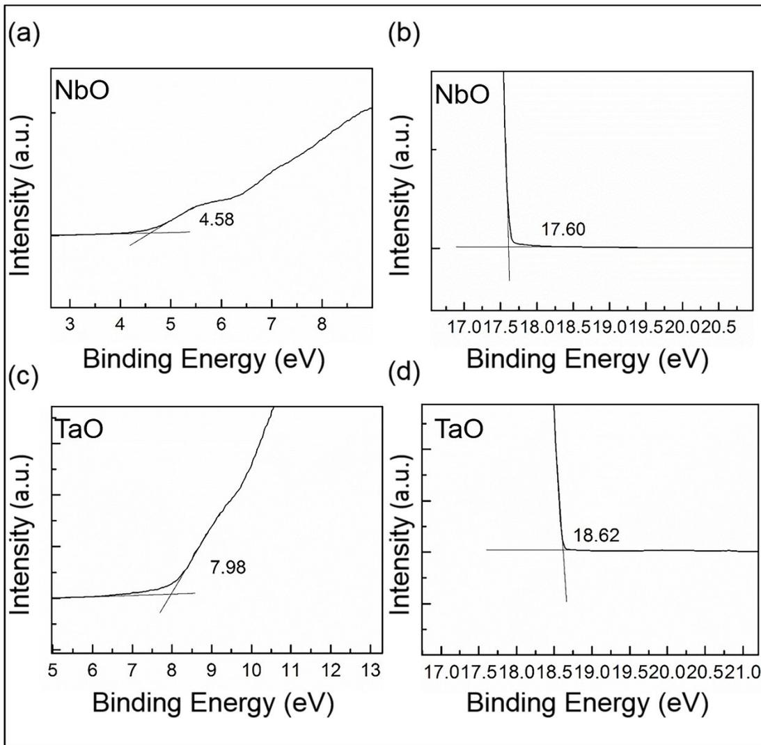
**Fig. S3** The UPS spectra of (a and b) NbO and (c and d) TaO after annealing. The work function of NbO is 3.62 eV (21.22 – 17.60). The VB level of NbO is situated at 8.20 eV (3.62 + 4.58). The work function of TaO is 2.60 eV (21.22 – 18.62). The VB level of TaO is situated at 10.58 eV (2.60 + 7.98).
