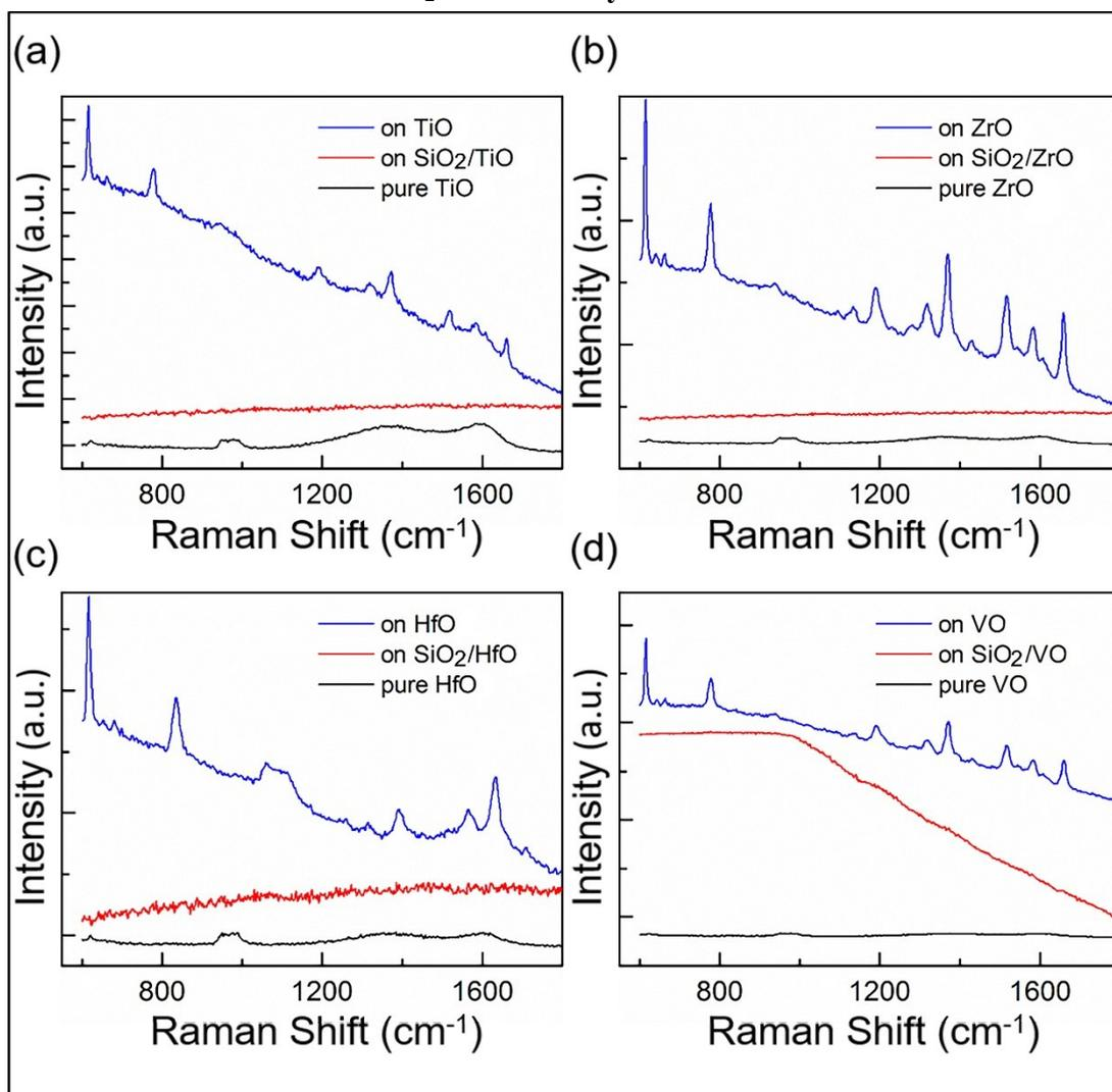
**Fig. S20** The Raman spectra of R6g at a concentration of  $10^{-5}$  M absorbed on (a) TiO, (b) ZrO, (c) HfO, (d) VO and a SiO<sub>2</sub> dielectric layer coated on them after H<sub>2</sub>annealing treatment.
