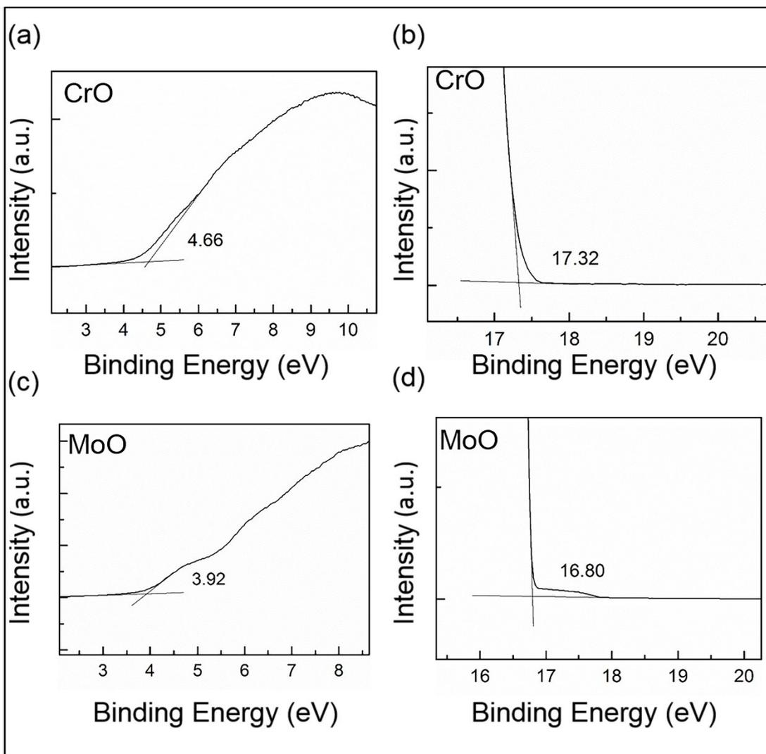
**Fig. S4** The UPS spectra of (a and b) CrO and (c and d) MoO after annealing. The work function of CrO is 3.90 eV ( $21.22 - 17.32$ ). The VB level of CrO is situated at 8.56 eV ( $3.90 + 4.66$ ). The work function of MoO is 4.42 eV ( $21.22 - 16.80$ ). The VB level of MoO is situated at 8.34 eV ( $4.42 + 3.92$ ).
