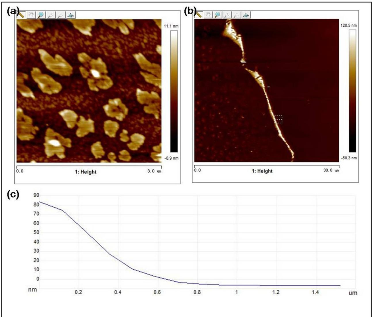
**Fig. S16** The roughness (a) and thickness (b) of MoO. The Ra value of roughness is 2.510 nm. (c) The value of thickness is below 90 nm.
