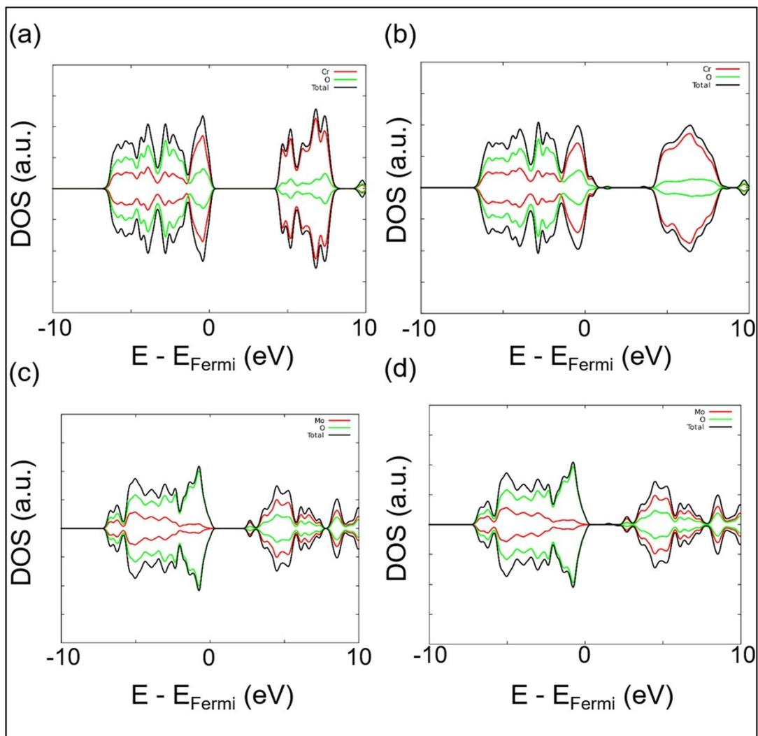
**Fig. S29** The PDOS of (a and b) CrO and (c and d) MoO before and after annealing, respectively.
