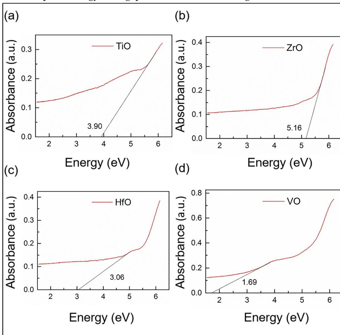
**Fig. S6**  $(\alpha\hbar\omega)^{1/2}$  as a function of photon energy ( $\hbar\omega$ ) for (a) TiO, (b) ZrO, (c) HfO and (d) VO. The optical energy band gap ( $E_g$ ) are 3.90 eV (TiO), 5.16 eV (ZrO), 3.06 eV (HfO) and 1.69 eV (VO), respectively.<sup>2</sup> The CB level of TiO is situated at 3.82 eV (7.72 – 3.90). The CB level of ZrO is situated at 3.46 eV (8.62 – 5.16). The CB level of HfO is situated at 5.37 eV (8.43 – 3.06). The CB level of VO is situated at 6.52 eV (8.21 – 1.69).
