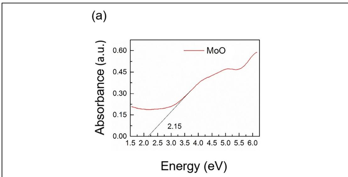
**Fig. S8**  $(\alpha\hbar\omega)^{1/2}$  as a function of photon energy ( $\hbar\omega$ ) for MoO.  $E_g$  is 2.15 eV. The CB level is situated at 6.19 eV (8.34 – 2.15).
