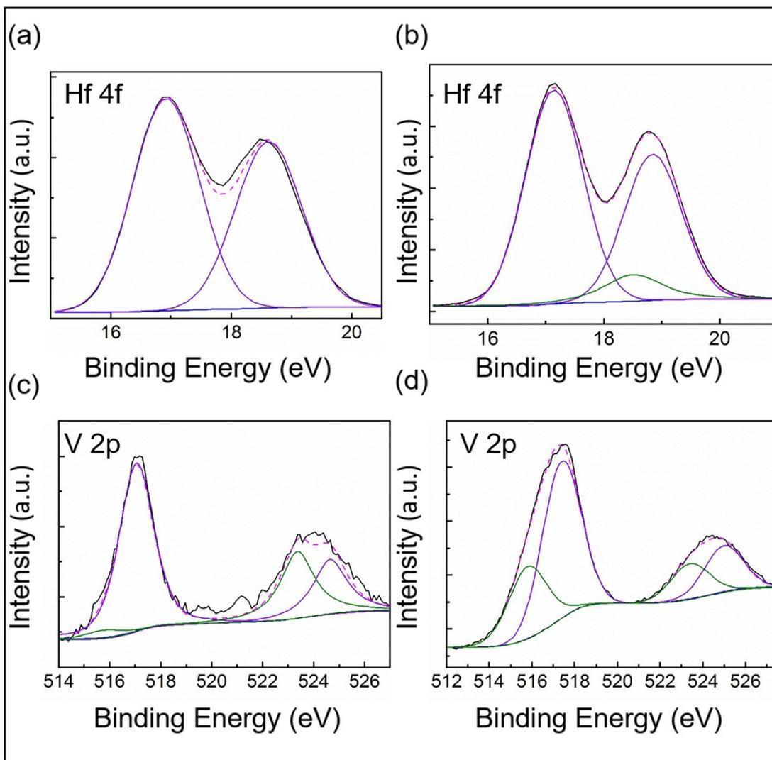
**Fig. S23** XPS spectra of (a and b) Hf 4f core levels for HfO and (c and d) V 2p core levels for VO before and after annealing, respectively.
