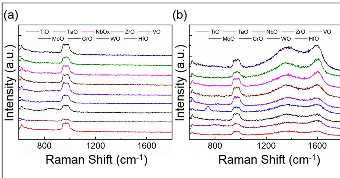
Fig. S30 Raman spectra of TMOs(a) before and (b) after H<sub>2</sub> annealing treatment.
