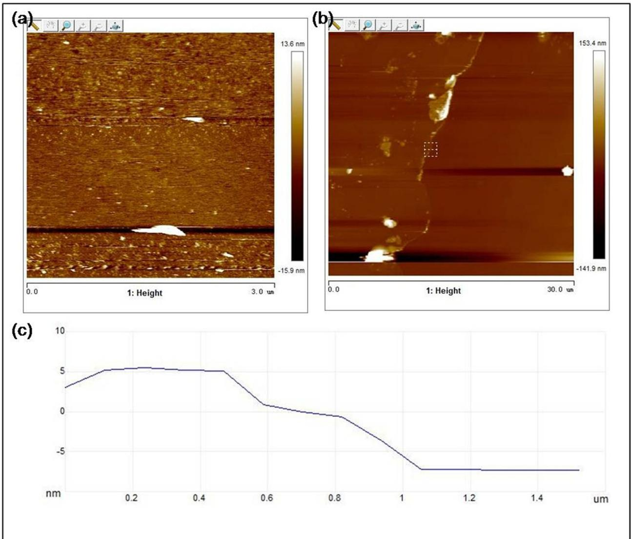
**Fig. S12** The roughness (a) and thickness (b) of VO. The Ra value of roughness is 1.730 nm. (c) The value of thickness is below 13 nm.
