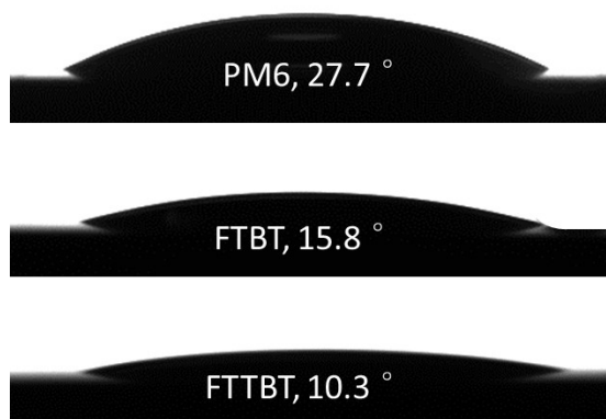
Figure S7. Contact angles of ethanol (EA) droplets on PM6, FTBT and FTTBT pristine films.
