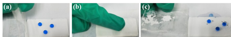
Fig. S10. Tape-peeling process on the SSF: (a) water droplets beaded on the intact SSF before tape-peeling test, (b) tape was tightly adhered to the SSF under pressure and (c) water droplets beaded on the damaged SSF after 30 cycles tape-peeling test.
