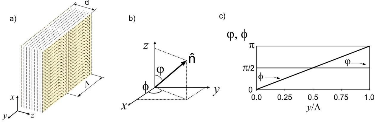
**Figure S2.** a) Schematic draw of the analyzed LC cell with the thickness of  $d$ . Black sectors indicate molecular alignment within LC layer as forced by the boundary conditions. b) Spatial orientation of the director specified by the orientation angles  $\phi$  and  $\phi$ . c) Orientation angles along  $y$ -direction (in the section limited to the single spatial interval of the periodic structure) when no voltage is applied to the LC cell.
