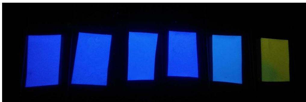
Figure S6: A comparison of normalized emission spectra of 4 and 7-11 in PMMA film (top). The fluorescence photograph of compounds 4 and 7-11 (left to right) in PMMA film (bottom). Irradiation was performed with a UV lamp with a wavelength of 365 nm.
