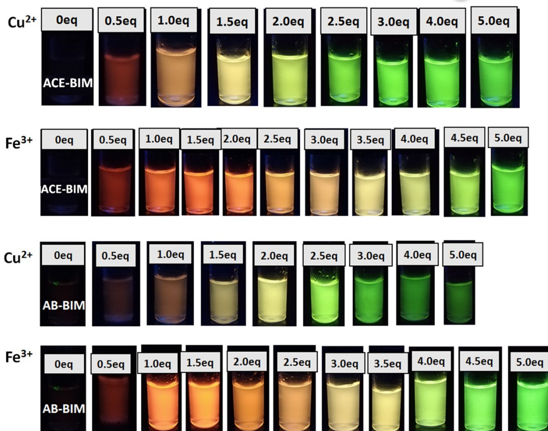
Fig. S5 Photographs of ACE-BIM and AB-BIM in \text{CH}_3\text{CN} upon titration of \text{Cu}^{2+} or \text{Fe}^{3+} ion under 365 nm of UV light.
