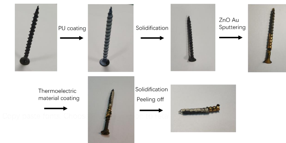
Fig. S1. The fabrication process of the integral device. PU was coated on a screw and solidified. After solidification, ZnO and Au were sputtered on the opposite sides on the latter part of the PU substrate. Thermoelectric materials and Ag contacts were coated on the left part. A complete device was fabricated after solidification and peeling.
